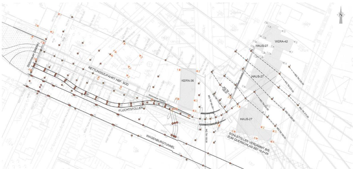
Figure 4.11: Surface Measurement Points/Sections TM 130 to TM 235
