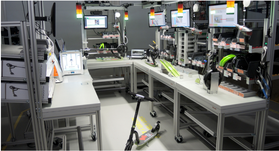
Figure 1.1: The digital state of the IIM LEAD Factory where scooters are assembled. In this state of the learning factory, many implementations of digitization are helping the training participants to optimize the throughput on the production line. These include camera systems for process recognition, cameras to capture facial expressions, gesture control of workplaces and many more.
