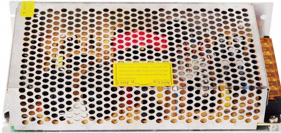
Figure 3.13: The power supply for the pick-to-light system. A version with 100 watt power was chosen, because in the worst case all 300 LED's with a total consumption of 90 watt (0.3 watt each) have to be supplied and additionally the controller has to be supplied with power. The output voltage is around 5 volts, whereby the exact output voltage can be adjusted with a screw.
