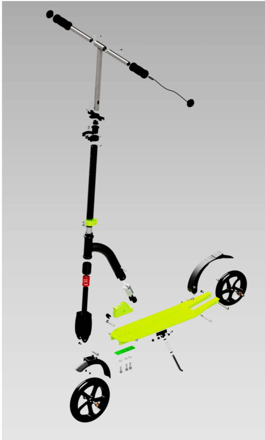
Figure 1.2: The IIM scooter which is assembled in the LEAD Factory exploded in its 60 parts. All these parts need to be assembled by the training participants of the LEAD Factory.
