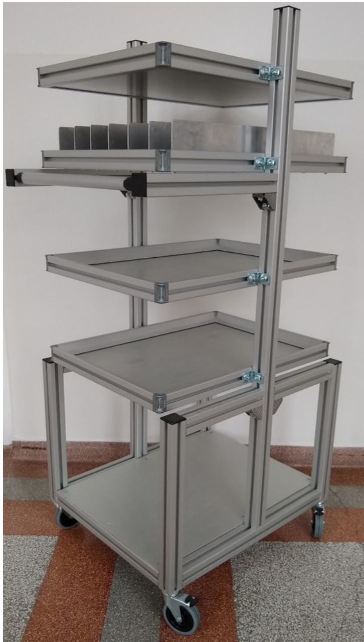
Figure 3.7: The milk wagon as used in the LEAD Factory is a device to transport material of all kind or boxes through the factory. It is supposed to support the logistics employee in his or her work. There are five levels on which the boxes can be placed. This makes it possible to transport a large number of boxes at the same time, which saves time and reduces costs. Milk wagons support lean manufacturing by reducing the seven types of waste. In this case it is mainly waste of transportation, waste from waiting time and waste from inventory.
