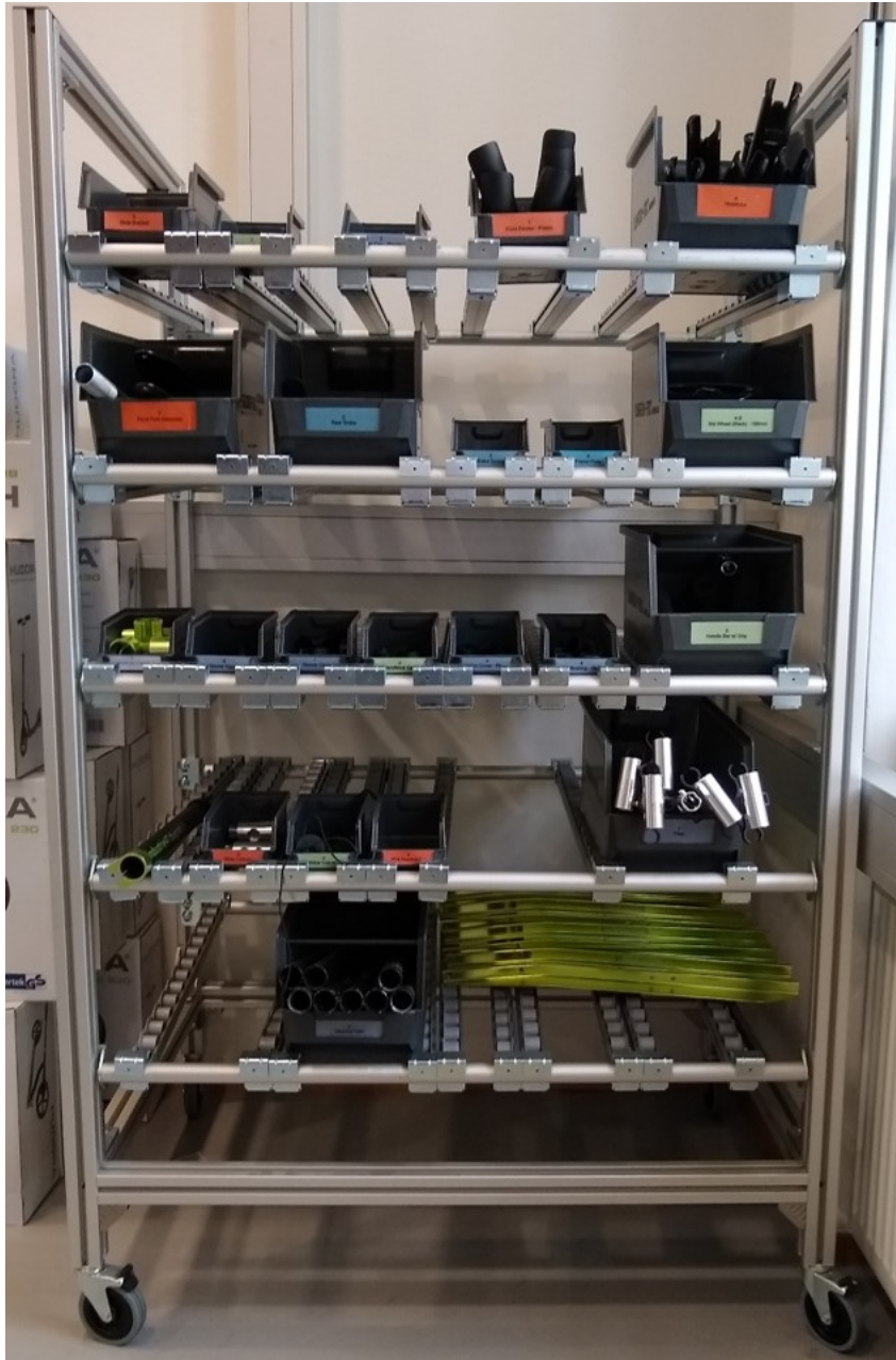
Figure 3.8: The supermarket or warehouse is the central supply station for the LEAD Factory. It contains 27 different parts which are needed for the milk-run. There are 23 different parts directly on the shelf. One part is on the left side and 3 more are on the right side of the shelf. The reason for this is that some parts are too big for the shelf.
