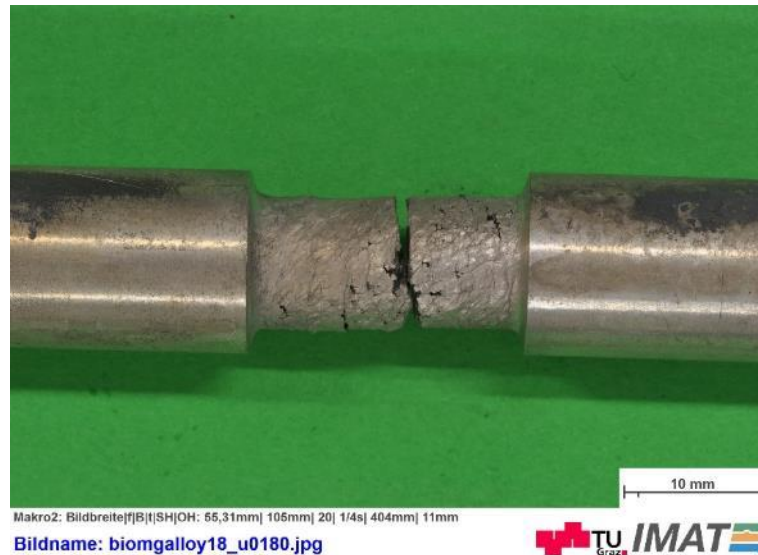
Figure 26: Sample deformed at 400 °C with \dot{\epsilon} = 0.001/s . Crack and surface damage.
