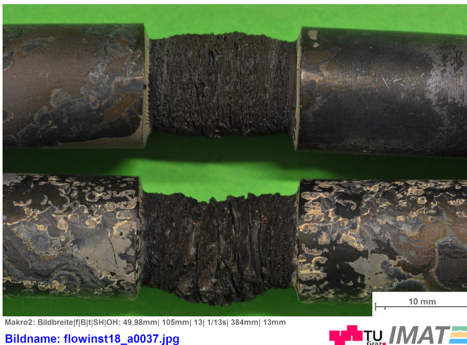
Figure 51: Macropicture of samples deformed at 950 °C 0.1 1/s strain rate up to strains of 8. Top: after deformation of as received structure, bottom: lamellar initial microstructure.
