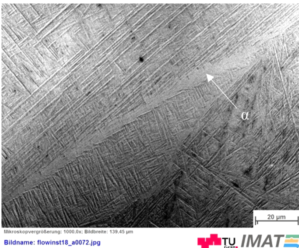
Figure 53: 970°C 1 1/s lamellar. Grain boundary \alpha .
