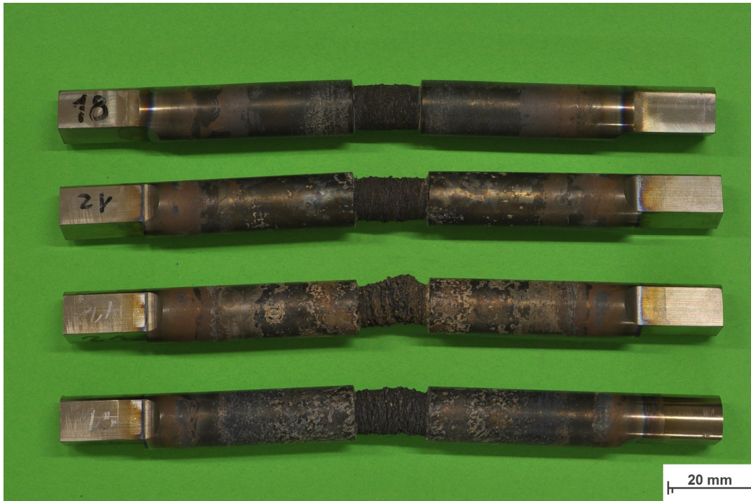
Figure 88: Torsion samples prepared for metallography deformed at 970°C. From top to bottom: 970°C 0.1 1/s, 970°C Clam 0.1 1/s, 970°C Clam 1 1/s, 970°C 0.1 1/s, 970°C 0.01 lam 1/s.
