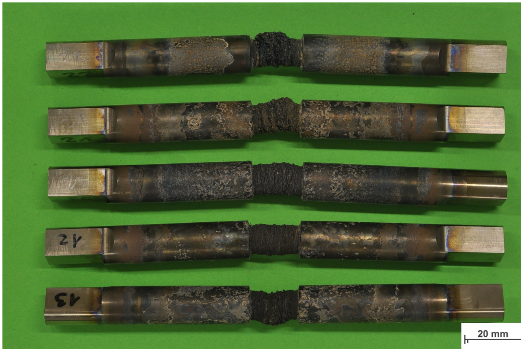
Figure 87: Torsion samples with lamellar structure prepared for metallography. From top to bottom: 950°C 1 1/s, 970°C 1 1/s, 970°C 0.01 1/s, 970°C 0.1 1/s, 950°C 0.1 1/s.
