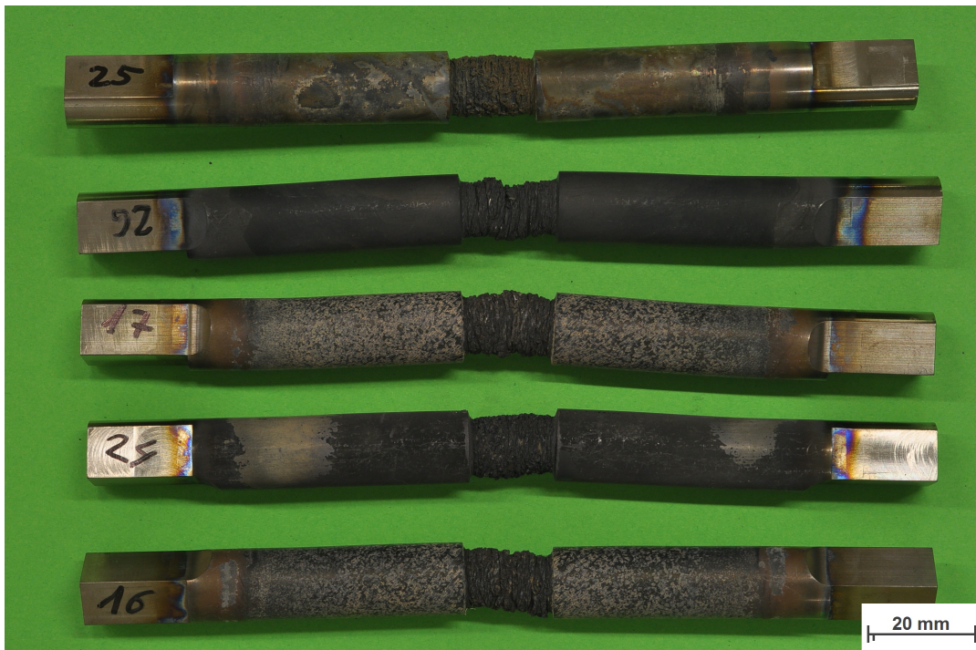
Figure 88: Torsion samples prepared for metallography deformed at 970°C. From top to bottom: 970°C 0.1 1/s, 970°C Clam 0.1 1/s, 970°C Clam 1 1/s, 970°C 0.1 1/s, 970°C 0.01 lam 1/s.
