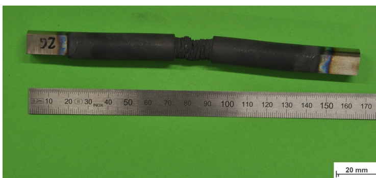
Figure 12: Assembly of torsion sample in the Gleeble® 3800.
