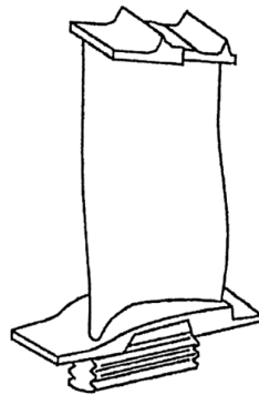
Figure 2.10: Shrouded tip geometry (Source: Earl and Ramendra (1995))
