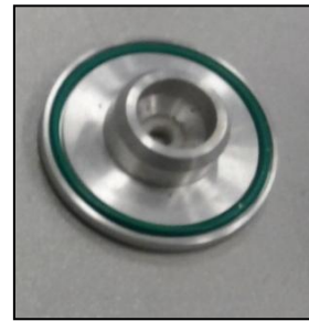
Figure 4.7: Cover plate of the oxidation air chamber
