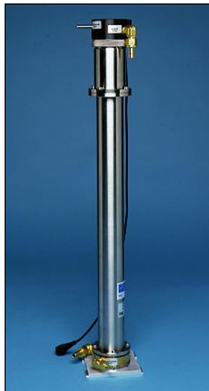
Figure 2.8: Long DMA from TSI, model 3081 (6)
