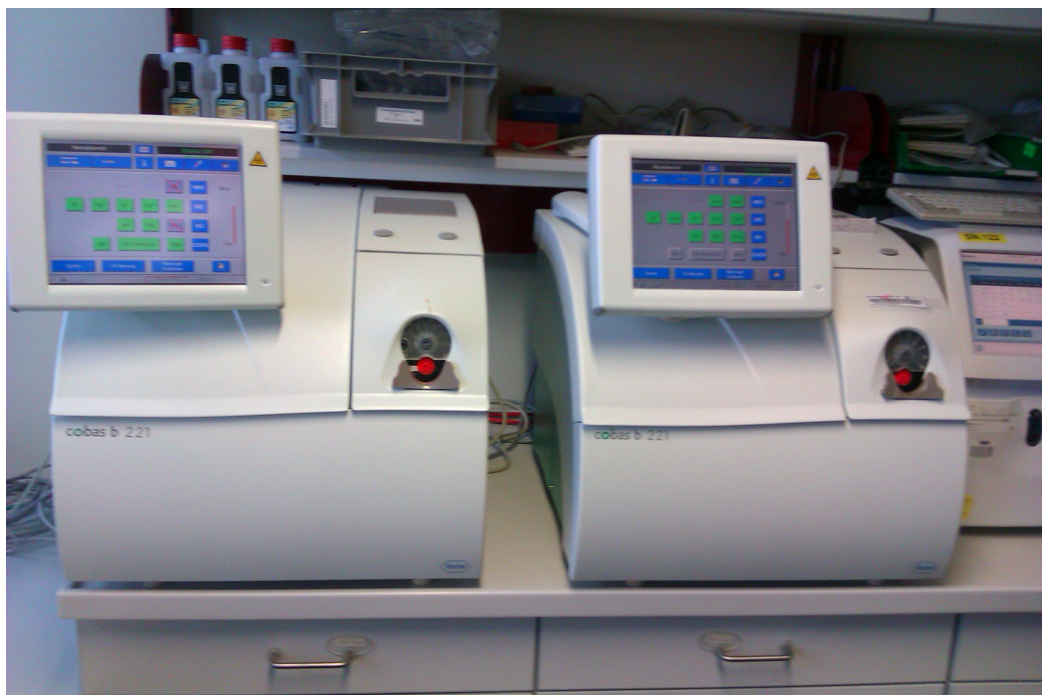
Figure C.3.: laboratory setup, cobas b221 , used as reference measuring devices for the ISE parameters.
