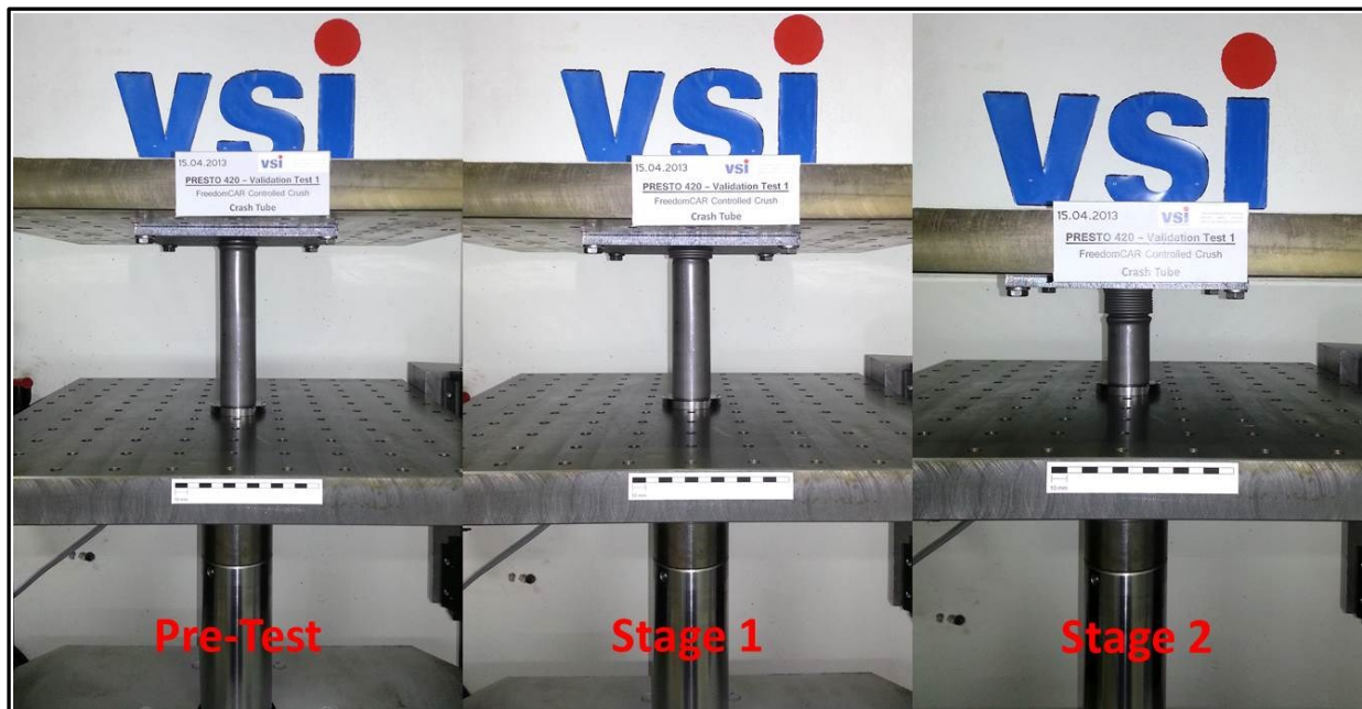
Figure 46: “PRESTO 420 – Validation Test 1 – Crush Tube”
