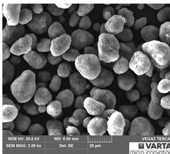
Figure 62: SEM pictures of a Gen3 powder
