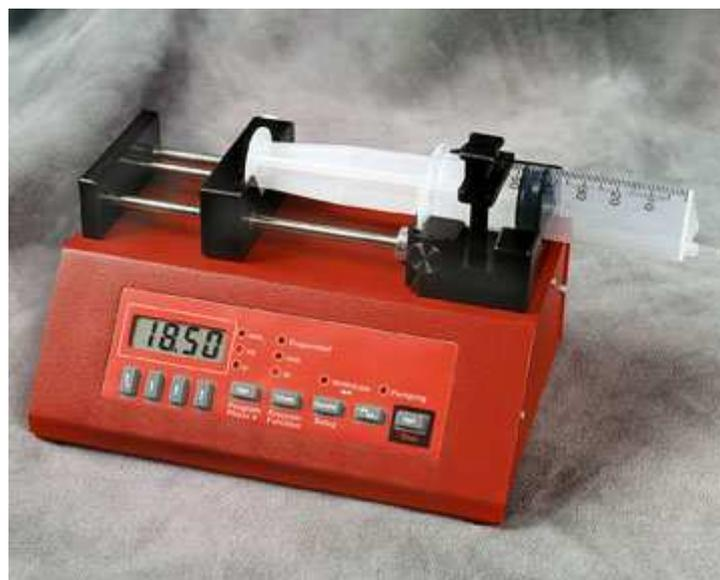
**Fig. 12:** The syringe pump used in the cOFM setup is an Aladdin, World Precision Instruments capable of push and pull mode. It is driven by a microcontroller system connected to a step motor, allowing a large range of flow rates configured to the inside diameter of the used syringe. The syringe is connected to the motor via a drive-screw and drive-nut mechanism.
