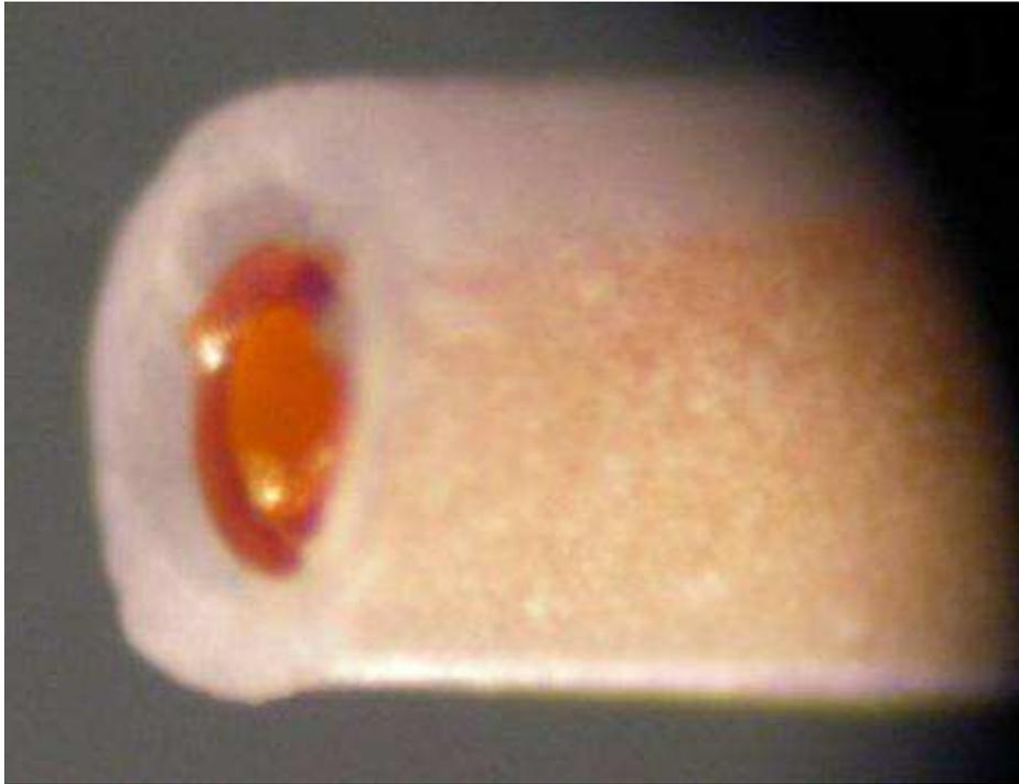
**Fig. 11: Magnified photo of the probe tip: The outer white transparent tubing is the guide cannula; the inner orange tubing is the inflow tubing.**
