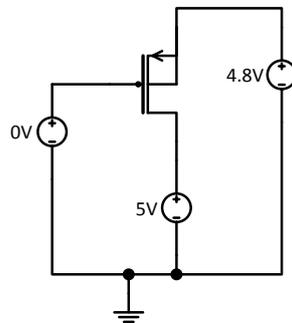
Figure 37 Test-bench for the 28V HV PMOS transistor as active-diode
