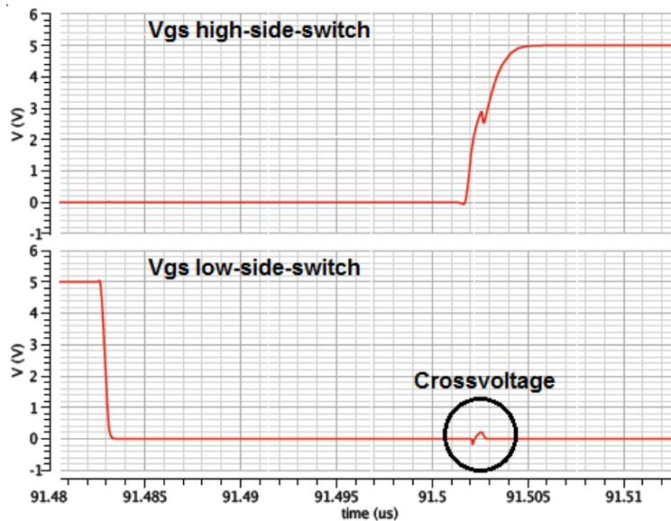
Figure 27 Shows the rising  $V_{GS}$  of the HSS and the generated crossvoltage at the LSS
