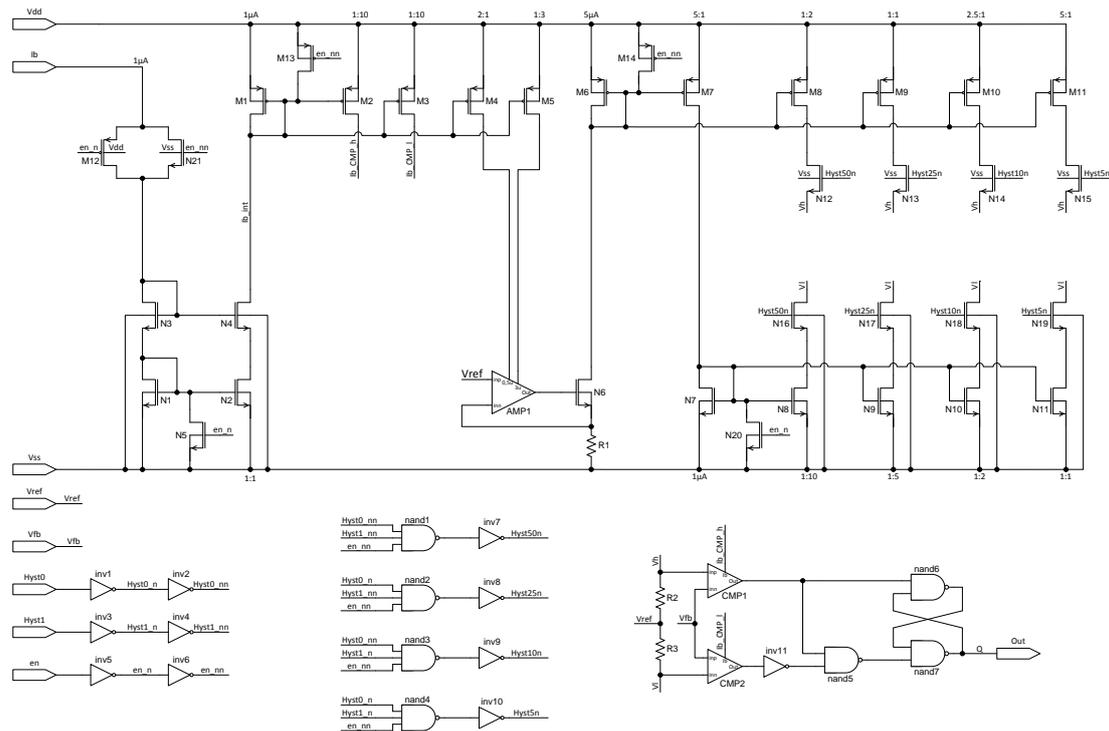
Figure 41 Shows the schematic of the hysteretic-comparator
