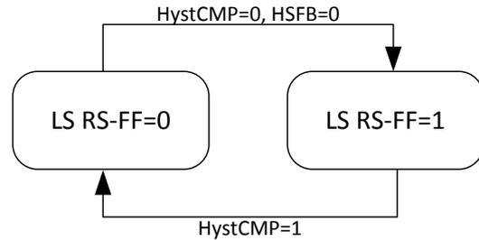
Figure 45 State-diagram for the HS LS-FF
