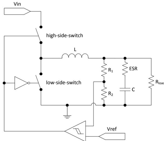
Figure 24 Shows a principle buck converter with hysteretic control loop
