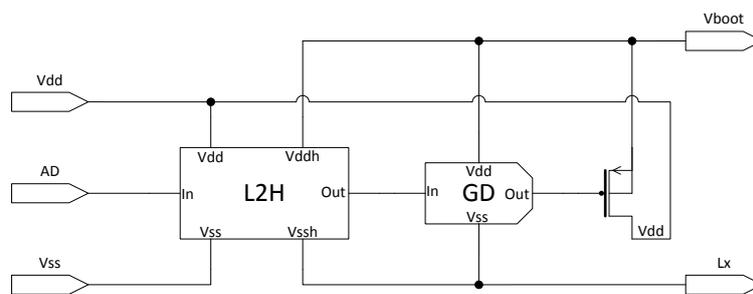
Figure 36 Shows the schematic of the active-diode block
