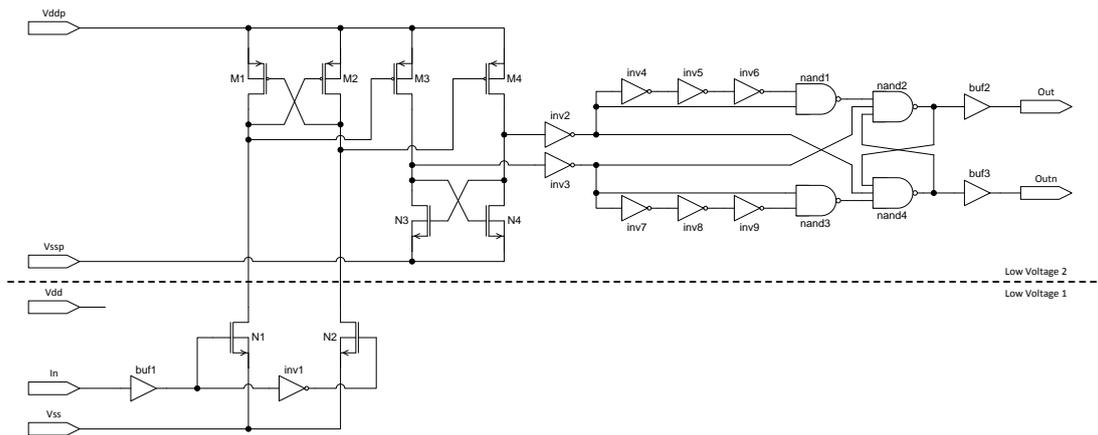
Figure 32 Shows the schematic of the low-to-low level-shifter for the gate-driver
