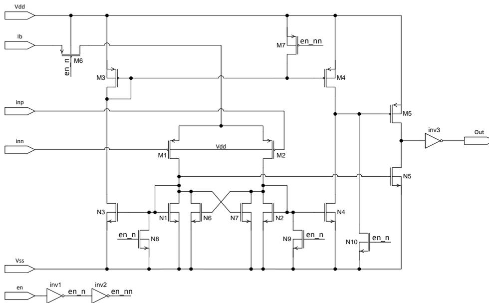
Figure 40 Shows the schematic of the comparator
