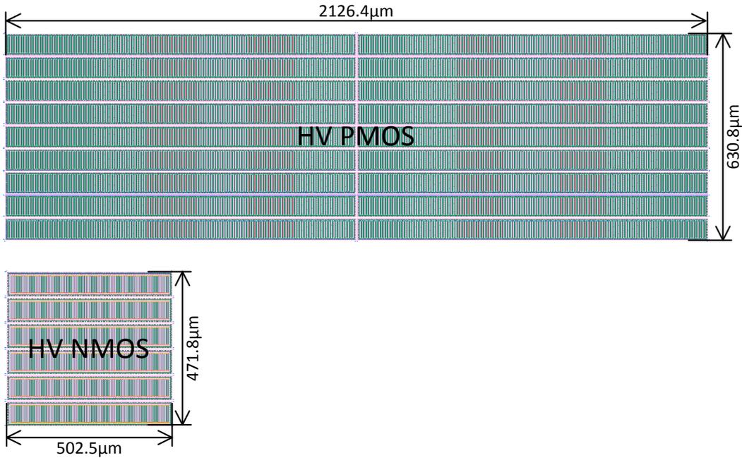
Figure 23 Silicon-area of HV PMOS transistor and HV NMOS transistor
