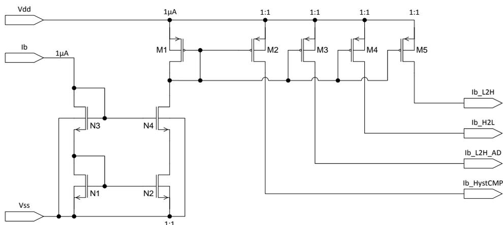
Figure 46 Shows the schematic of the current-bank
