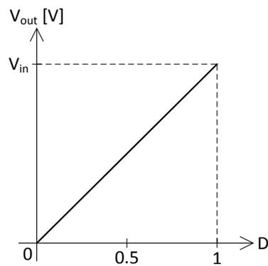
Figure 7  $V_{out}$  vs. duty cycle for an ideal buck converter [1]
