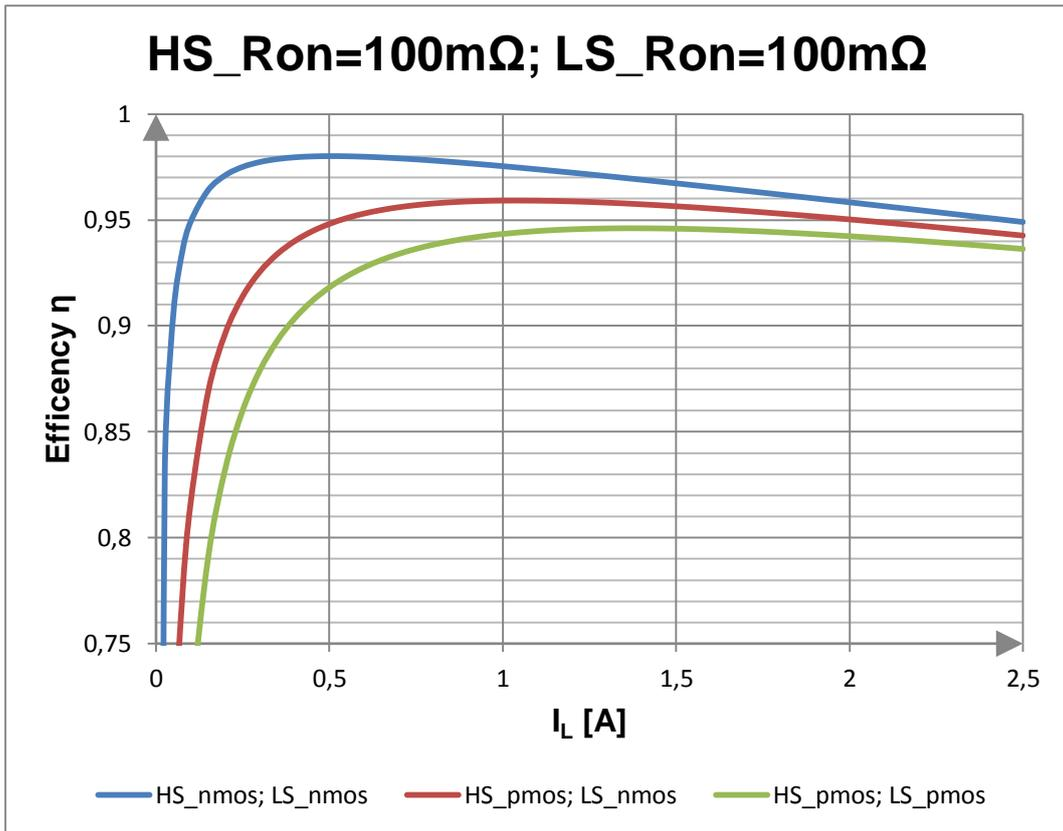
Figure 20 Results of the efficiency calculation for  $R_{ON}=100m\Omega$  for both switches
