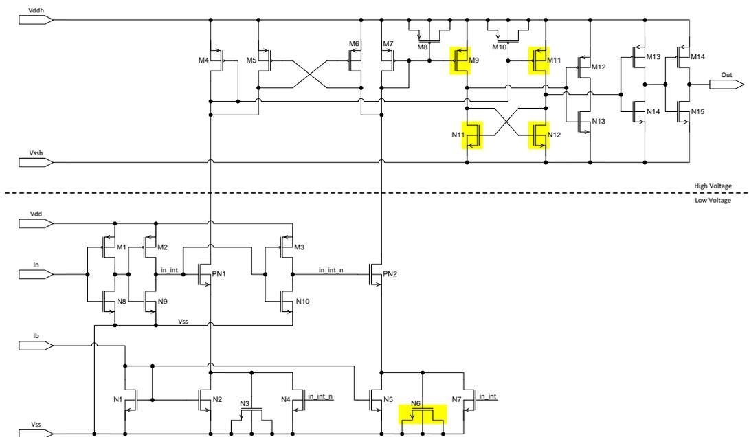
Figure 30 Shows the schematic of the low-to-high level-shifter for active-diode
