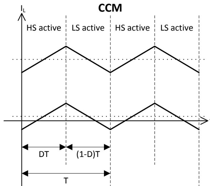
Figure 8 Shows possible coil currents of a buck converter in CCM [4]
