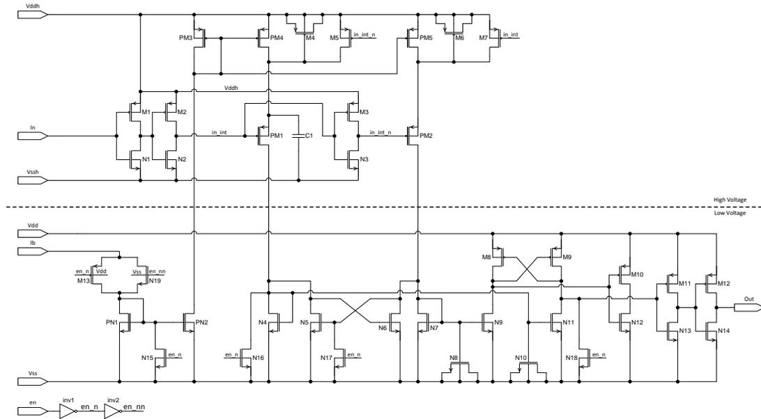
Figure 31 Shows the schematic of the high-to-low level-shifter
