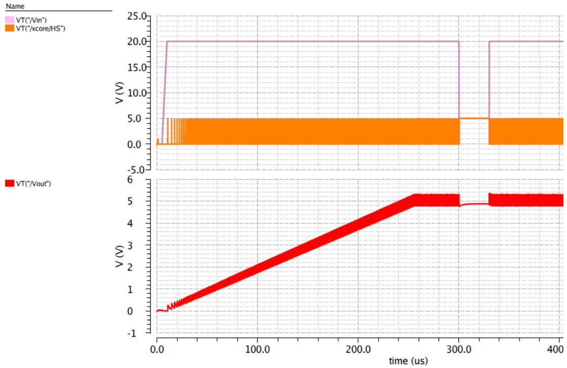
Figure 48 Shows the start-up of the buck converter for  $V_{in}=20V$  and a  $V_{out}$  of 5V
