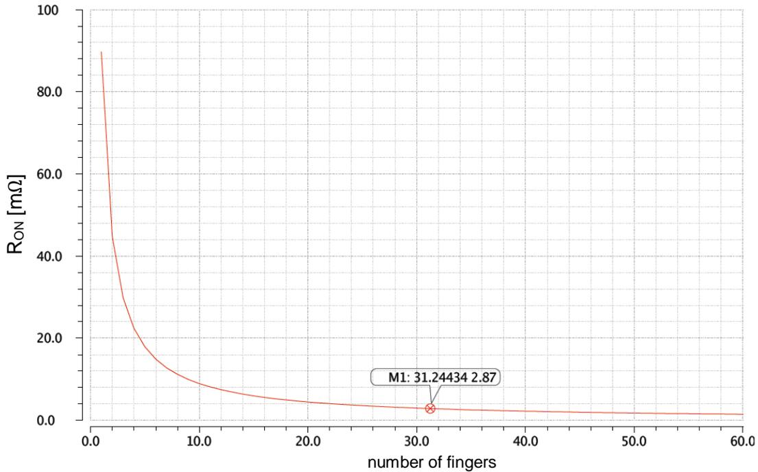
Figure 38 Sweep simulation over numbers of fingers for a 28V HV PMOS transistor
