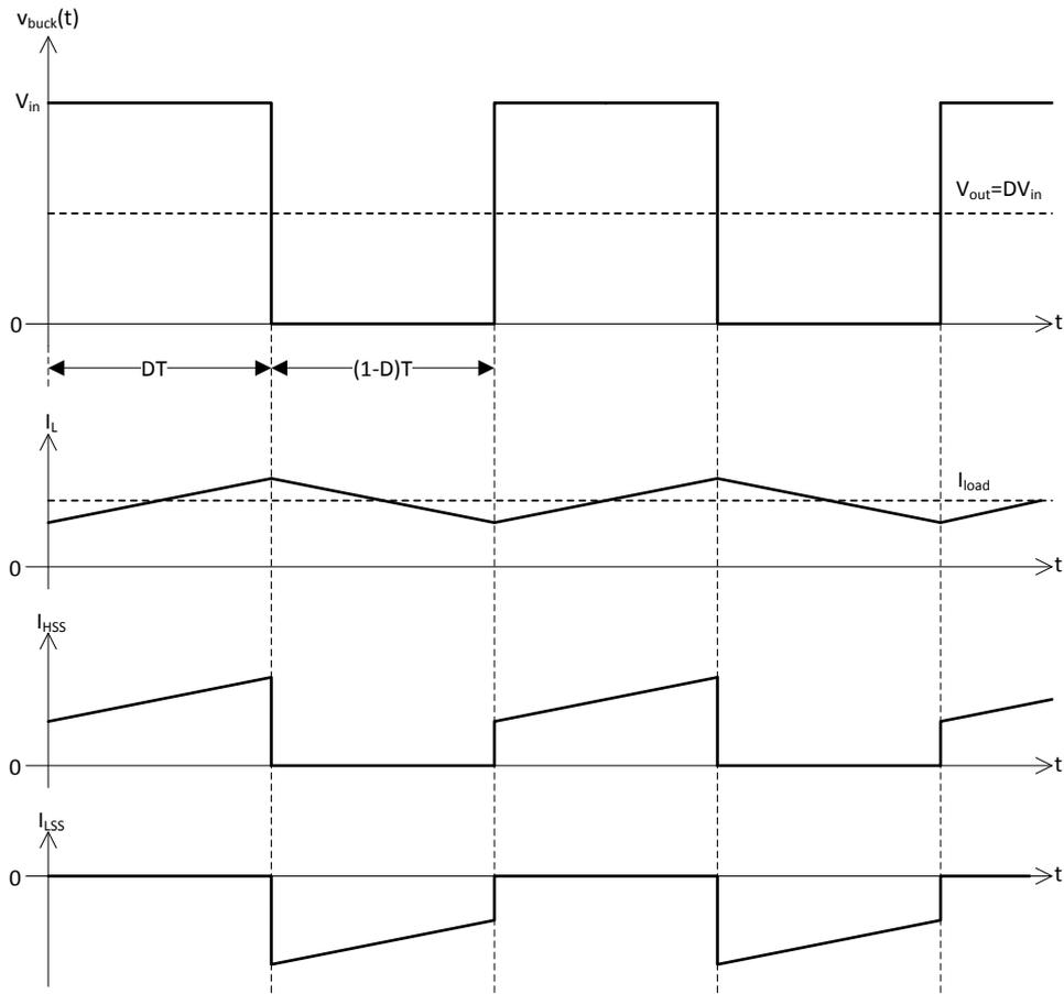
Figure 6 Shows the currents through the coil and both switches of the buck converter
