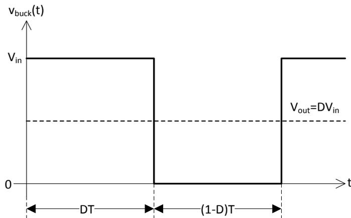
Figure 4  $v_{\text{buck}}(t)$  of the buck converter and  $V_{\text{out}}$  which is the average voltage of it [1]
