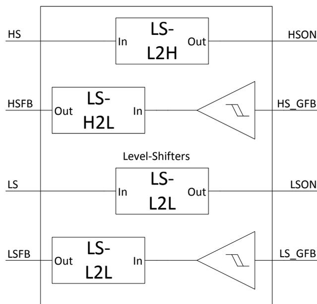
Figure 14 Shows a level-shifters and Schmitt-trigger sub-block
