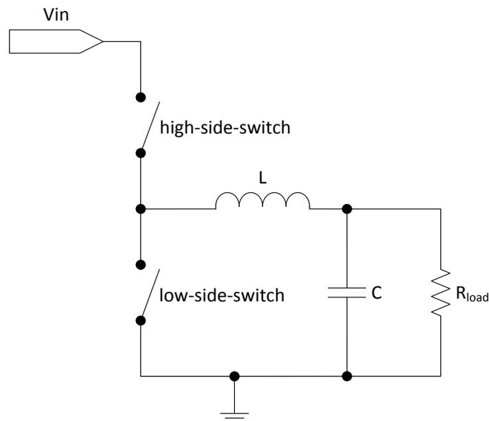
Figure 5 Shows an ideal circuit of a buck converter [1]
