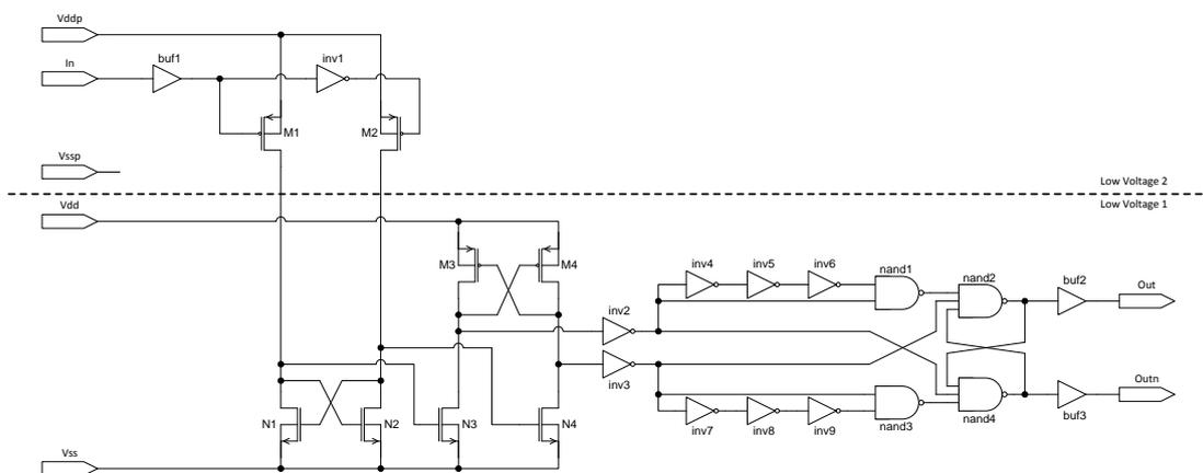
Figure 33 Shows the schematic of the low-to-low level-shifter for the gate-feedback
