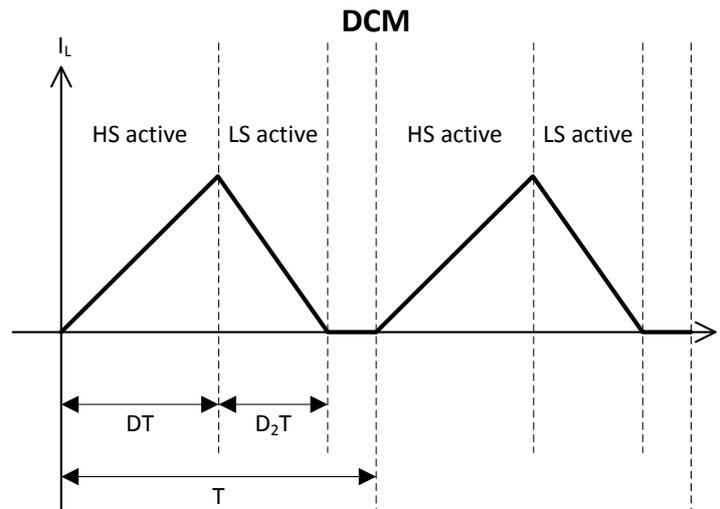
Figure 10 Shows the coil current of a buck converter in DCM [4]
