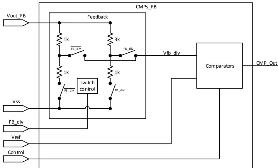
Figure 15 Shows a principle block for the feedback and the control loop comparator
