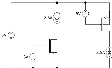
Figure 18 Test-bench for simulation of  $V_{DS}$
