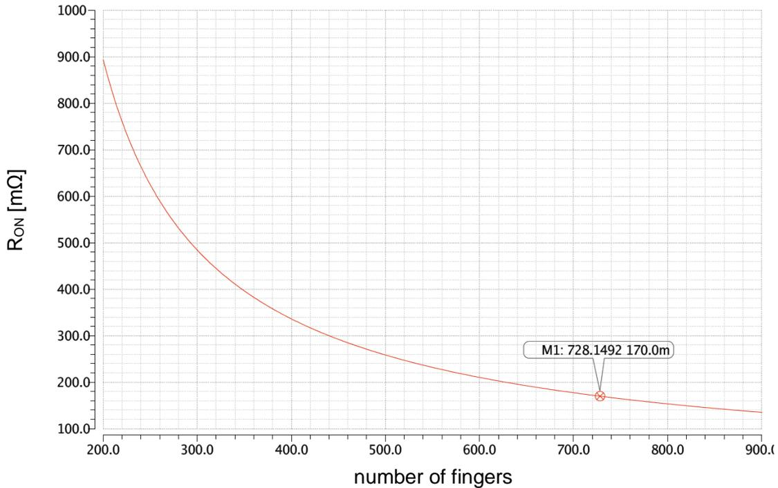
Figure 26 Sweep simulation over numbers of fingers for a 20V HV NMOS transistor
