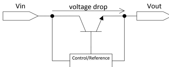
Figure 1 Simple block diagram of a linear regulator [10],[11]
