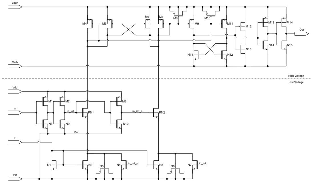
Figure 29 Shows the schematic of the low-to-high level-shifter
