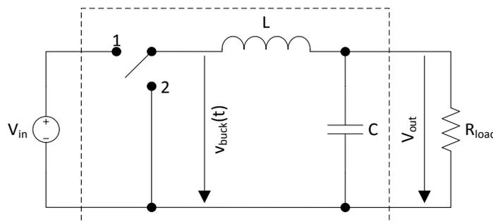
Figure 3 Principle circuit of a buck converter [1]
