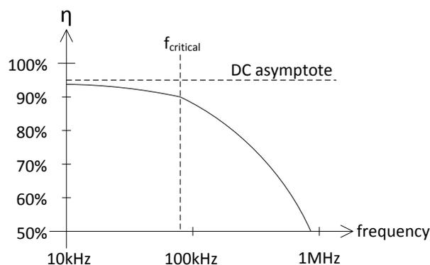
Figure 11 Shows the efficiency vs. switching frequency [1]
