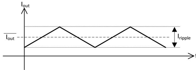
Figure 9 Shows a possible form of a current ripple
