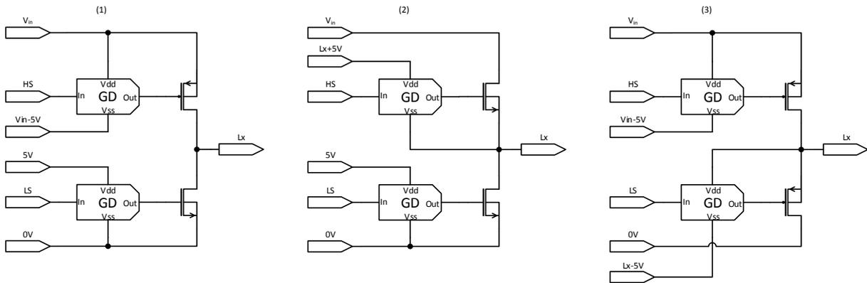
Figure 17 Shows the half-bridges for the different topologies: (1) PMOS for HSS, NMOS for LSS (2) NMOS for both switches (3) PMOS for both switches
