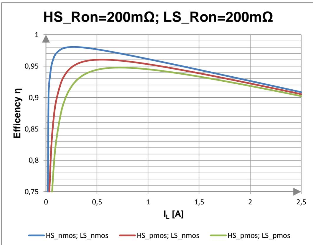
Figure 21 Results of the efficiency calculation for  $R_{ON}=200m\Omega$  for both switches
