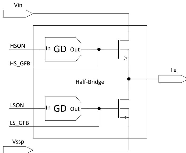
Figure 12 Example for a half-bridge sub-block
