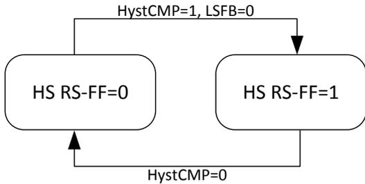
Figure 44 State-diagram for the HS RS-FF
