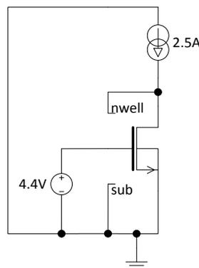
Figure 25 Test-bench for simulation of the  $R_{ON}$  of the 20V HV NMOS transistor
