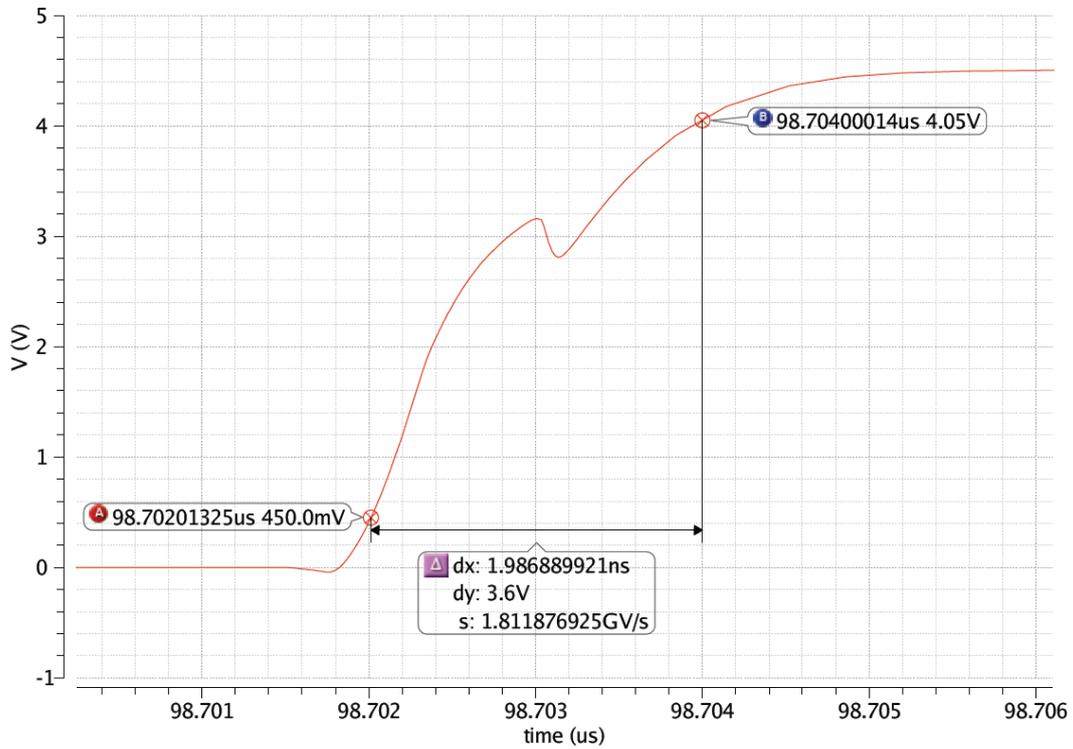
Figure 13 Shows rising of the output voltage from the gate-driver. The Miller-plateau can clearly be seen.
