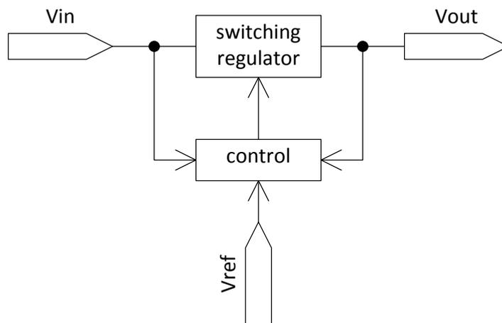
Figure 2 Simple block diagram of a switching regulator [1]
