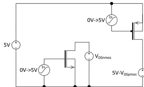
Figure 19 Test-bench for simulation of  $Q$  and  $C_G$
