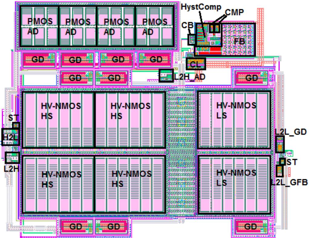
Figure 59 Shows the floor plan of the entire design
