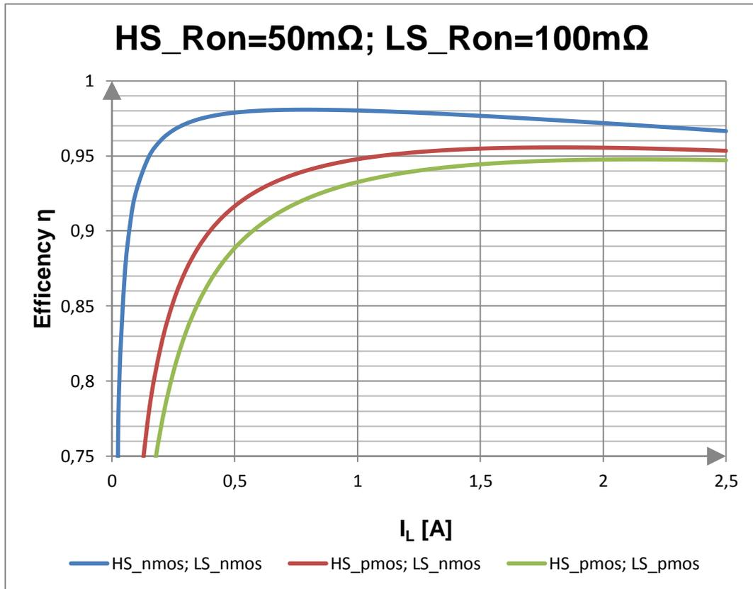
Figure 22 Results of the efficiency calculation for different values of  $R_{ON}$  for HSS and LSS
