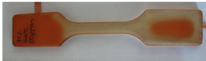
Figure 36. pDCPD cured with 50 ppm M2 at 40 °C exhibiting two zones (red and yellow).
