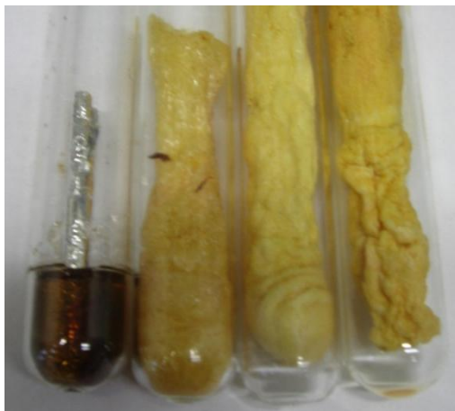
Figure 48. Poly- DCPD-co-norbornadiene (ratios: 1:0, 2:1, 1:1, 1:2) polymerised with 150 ppm M2 at 25 °C.
