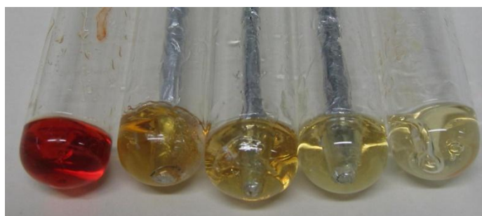
Figure 67. Poly9 polymerised with 25 ppm M2 and 50, 75, 100 and 150 ppm M20 (l.t.r.) at 25 °C.
