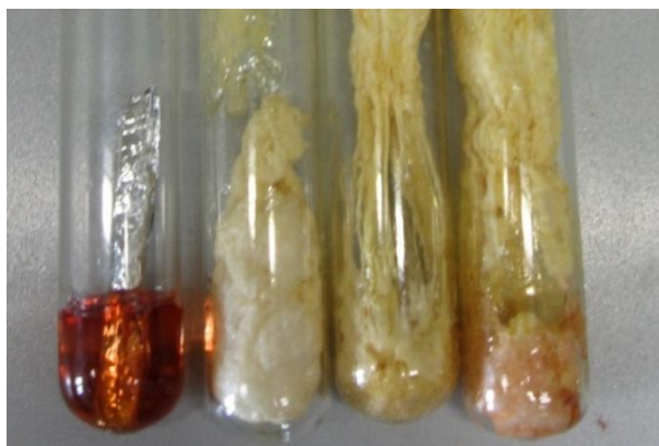
Figure 45. Polynorbornadiene polymerised with 50, 75, 100 and 150 ppm M2 (l.t.r.) at 25 °C.
