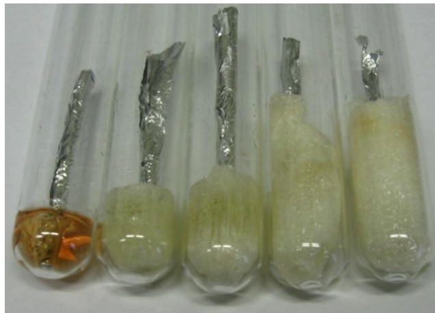
Figure 51. Poly3 polymerised with 25, 50, 75, 100 and 150 ppm M2 (l.t.r.) at 25 °C.
