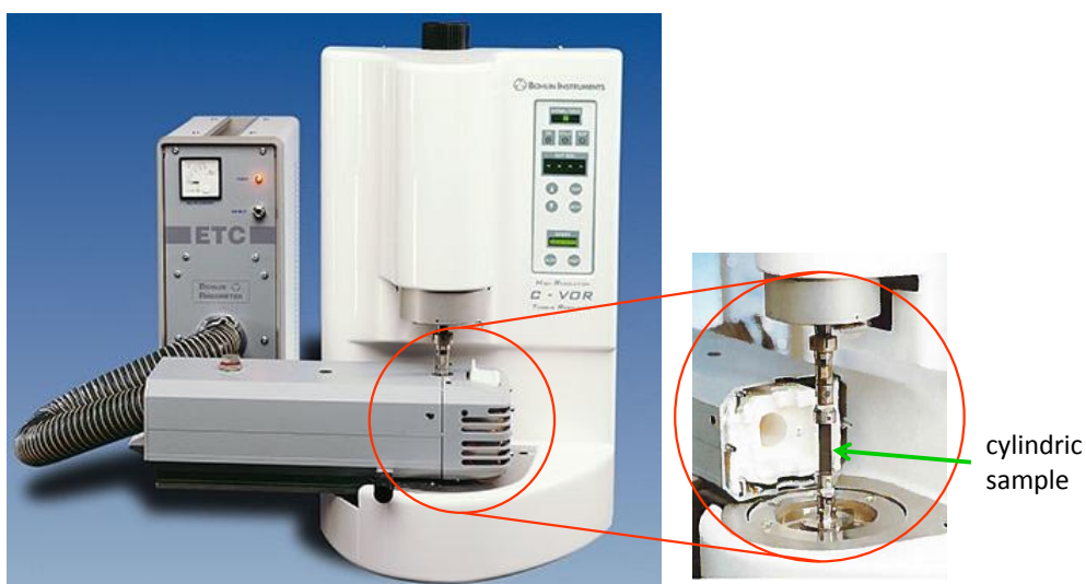
Figure 17. Rheometer for DMA measurement; closed furnace (left); open furnace (right).
