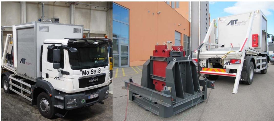
FIGURE 3-9 MOBILE SEISMIC SIMULATOR FROM AIT (PICTURE AIT)
