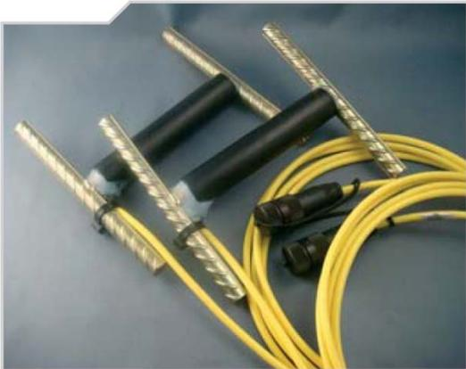
FIGURE 2-12 SHOTCRETE STRAINGAUGE (GEODATA ZT GMBH, 2008B)
