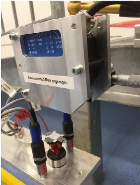
FIGURE 4-4 OPTONCDT ILD1700-50 MOUNTED ABOVE THE PRISM
