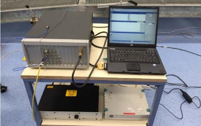
FIGURE 4-2 PC FOR SHAKER CONTROL, LMS (UPPER LEFT) AND AMPLIFIER (LOWER LEFT)
