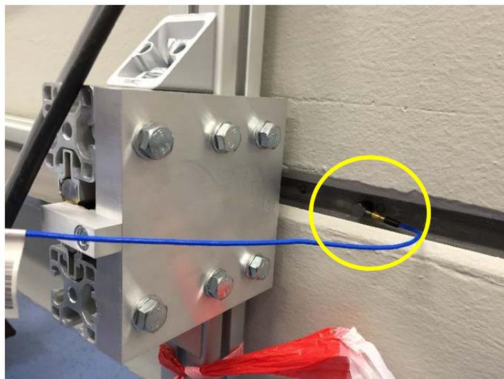
FIGURE 5-21 ACCELEROMETER MOUNTED ON THE COMPARATOR BENCH
