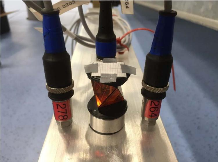
FIGURE 4-3 ACCELEROMETERS AND 360° MINI PRISM MOUNTED ON THE TEST BED
