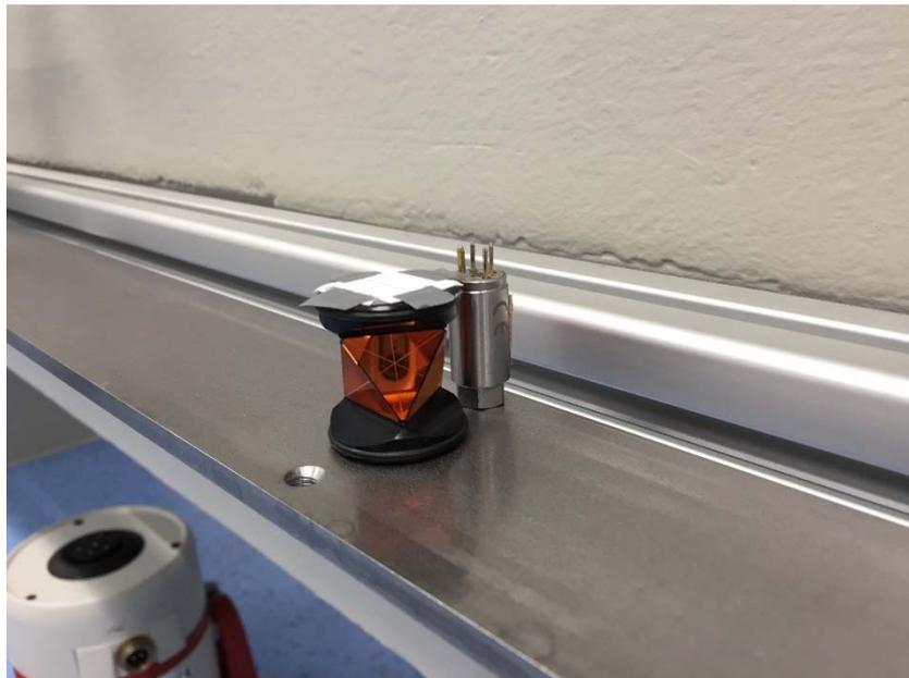
FIGURE 5-5 PRISM AND ACCELEROMETER
