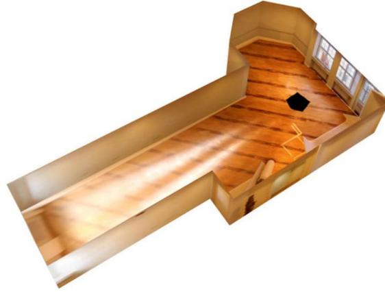
**Figure 1.4:** A sample room scanned in the course of the DURAARK project. The scanner was placed above the dark spot. Due to the chosen scanning position, the wall surfaces and thus the room structure is captured at once. However, the chosen scan position is unfavorable in terms of data density on long-sided wall segments. This image was taken from [33].
