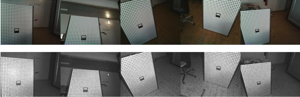
**Figure 2.6:** Camera calibration target with circular pattern from different positions and angles as captured by the RGB sensor (top) and the IR sensor (bottom).
