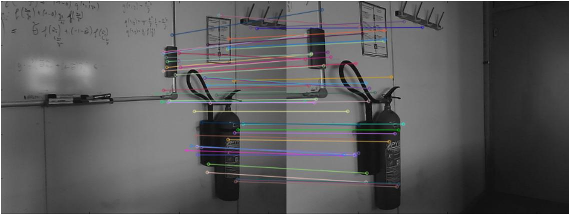
**Figure 2.10:** Real world data of SURF features and matches. Only the 50 best matches are drawn.
