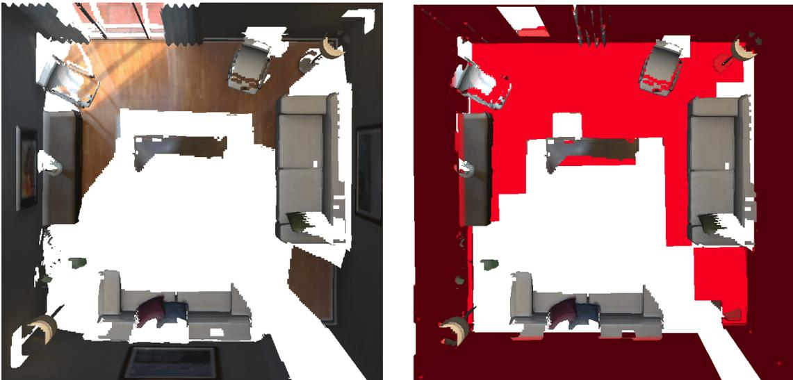
Figure 4.6: Plane estimation (depicted in red) in the icl/lr1 dataset with groundtruth trajectory.
