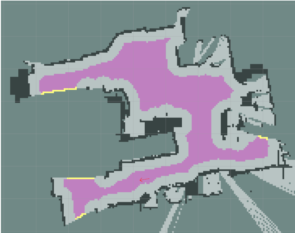
Figure 5.16: A map with accessible cells (purple and yellow cells) and frontiers (yellow cells)
