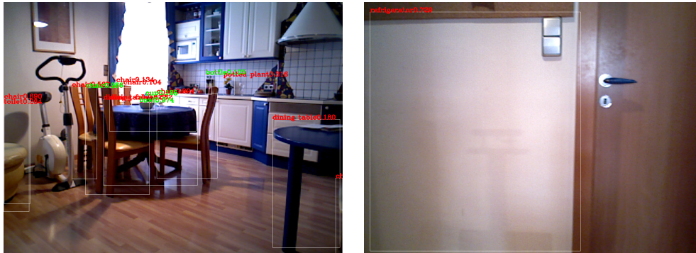
(a) High confidence for the chairs in front and the bowl, low confidences for all other objects; the wine glass on the right of the potted plant was not detected at all
