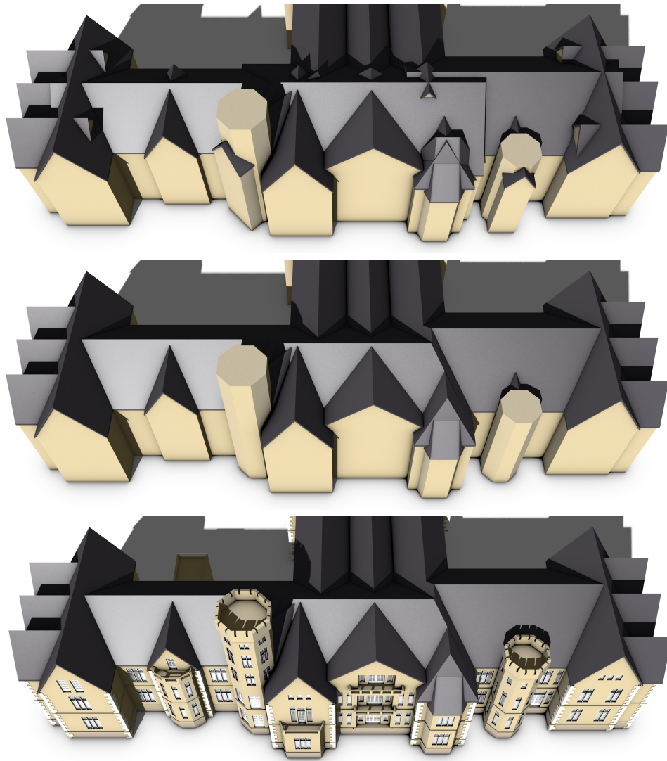
Figure 5.1.: Modeling a building by parametrizable parts greatly reduces the necessary effort. A simple union of parts might lead to undesirable results (top). Therefore, we introduce automatic roof trimming for solid building primitives (middle). The resulting model can be further refined using existing procedural approaches (bottom).
