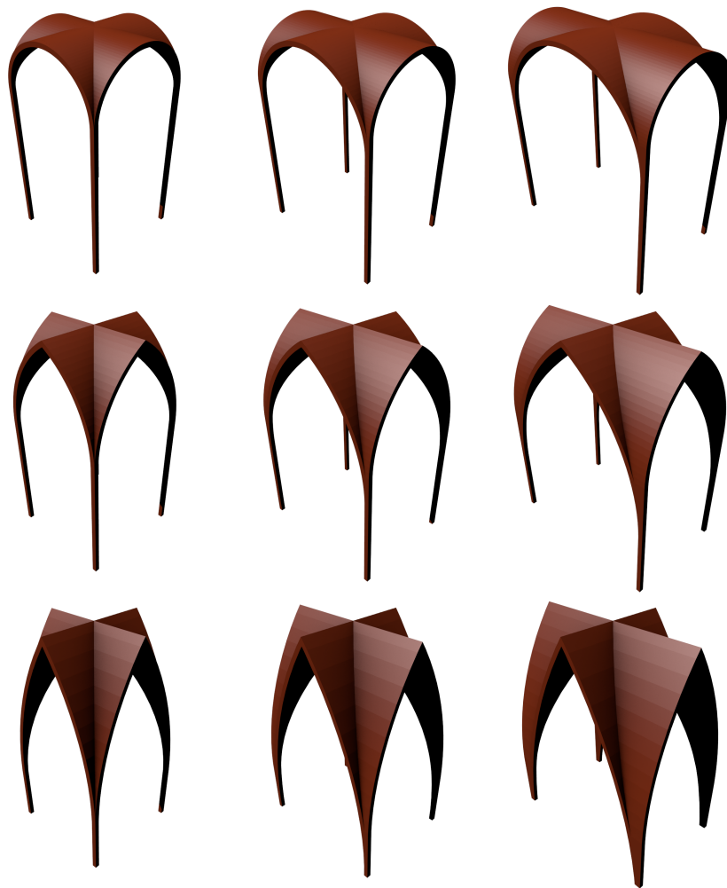
Figure 6.7.: Variations of a procedural cross-vault model. To the right the width increases, and the arch automatically adapts to the new space. To the bottom the angle of the arch decreases and the arch becomes a pointed arch.
