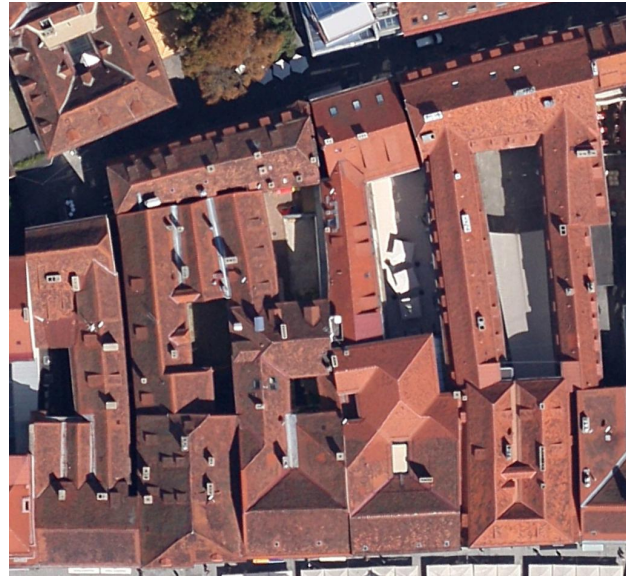
Figure 5.4.: Aerial image of the inner city of Graz, Austria. Different roof parts merge and form a complex roof landscape. There are many implicit dependencies of parameters of roof faces like slope, height of eave, etc. This roof landscape is not easily created with existing modeling tools. Imagery ©2015 Google, Map data ©2015 Google.
