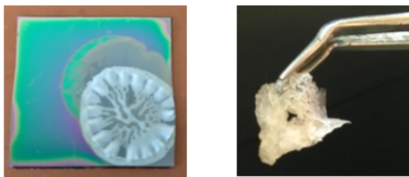
Figure 25: Si substrate pre-coated with p(HEMA-EGDMA), drop-cast with IL which was solidified in another iCVD process. The solidified IL starts to detach from the substrate (left) and can be pulled off to gain free-standing membranes (right).
