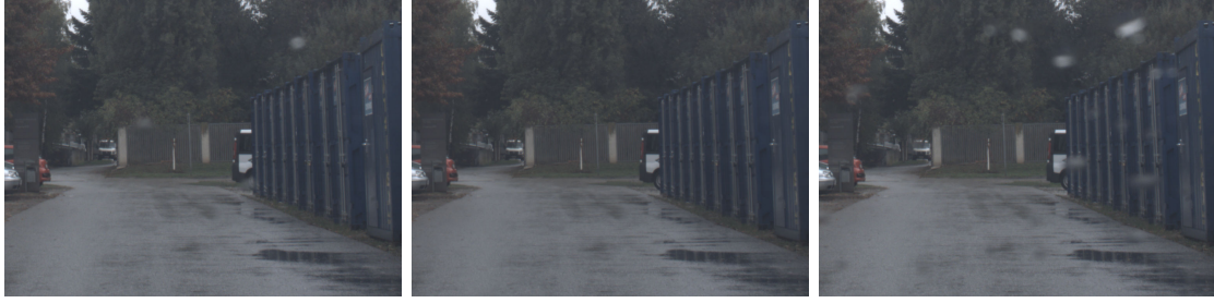
Figure 3.4: Comparison between details of clean and dirty images for an image on a rainy day. Left is one image with as few raindrops as possible to generate a clean image. The middle image is the generated clean image. On the right the dirty image with raindrops present.
