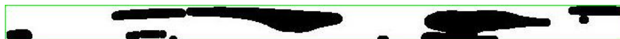
Figure 5.4 Highlight mask which holds bright and dark spots to improve iris-lens border detection
