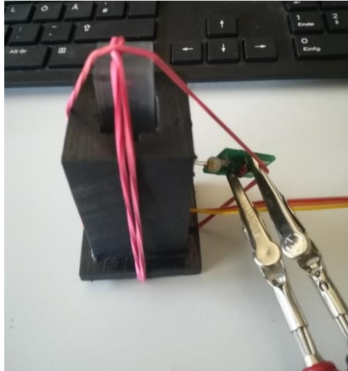
Figure 42 3D-printing as a holder for the cuvette and the small PCB in between
