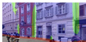
(c) Segmentation Result (blue: background, green: vertical edge, red: horizontal edge)
