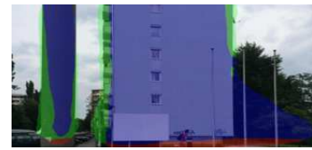
(c) Segmentation Result (blue: , green: vertical edge, red: horizontal edge)
