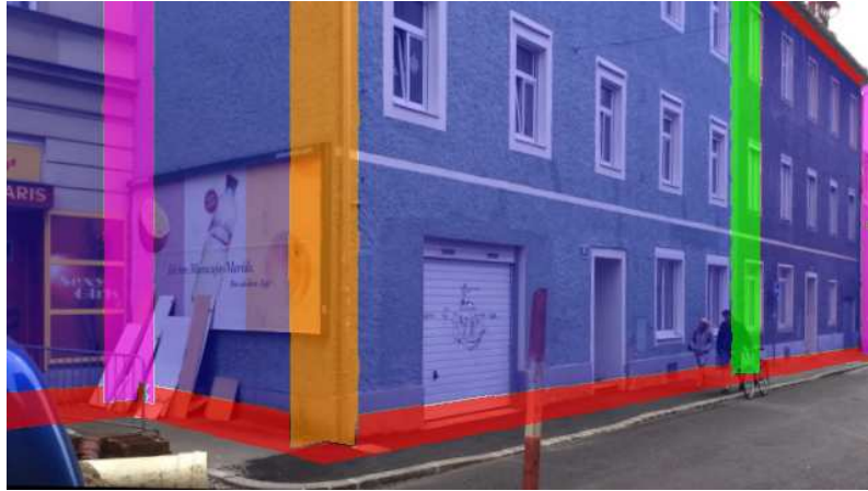
Figure 6.1: Renderings of the convex, concave and flat vertical edges of the 2.5D map under the ground truth pose are overlaid on the input image. We show an example of the different vertical edge types such as convex (orange), concave (magenta) and flat (green) that can be further exploited for urban camera localization.
