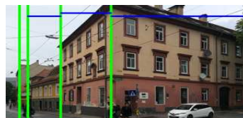
(h) Found corners (green) and defined facades (blue) shown over the rectified input image.
