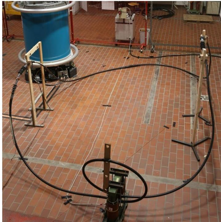
Figure 6-6: PQ test setup
