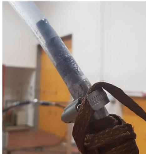
Figure 6-10: Water resistor, conical shaped plug
