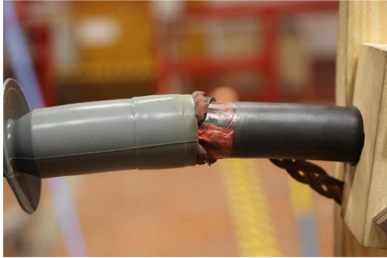
Figure 7-8: Visible stress at back end of termination
