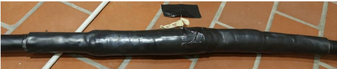
Figure 6-5: Installed standard 12/20 kV AC cable joint
