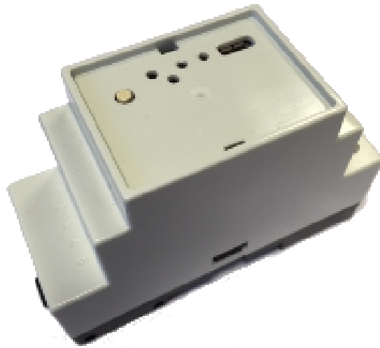
Figure 1.2: The "Compact Unbranded", a blank for various brands. After electric and housing assembly but before provisioning
