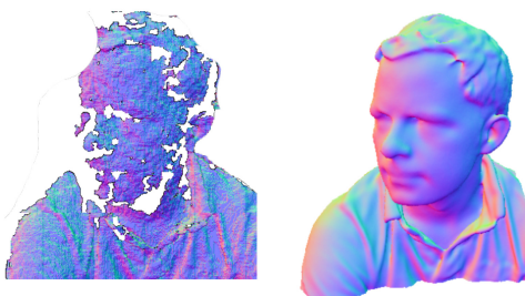
Figure 2.1: KinectFusion - Input Data and Static Reconstruction (Newcombe et al., 2011) (Image taken from Newcombe et al. (2011).)
