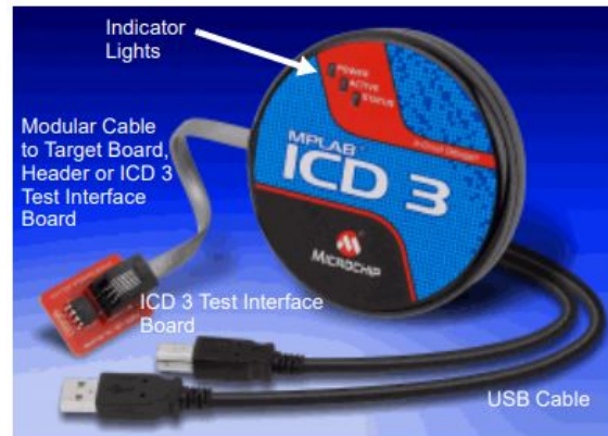
Figure 2.8.: The ICD 3 is an in-circuit debugger controlled by the MPLAB X IDE software. It allows the user to debug his application with his own hardware, with hardware and software breakpoints and monitor the internal registers. It is also used to program the device. [14]
