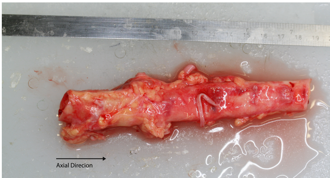
Figure 7: Abdominal aortic tissue from Institute of Pathology with surrounding connective tissue which needs to be removed before testing without harming the adventitia. The photographed centimeter scale provides a dimensional reference.
