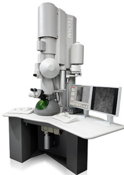
Figure 5: Electron Transmission Microscope FEI Tecnai™ F20 ©FEI Company.
