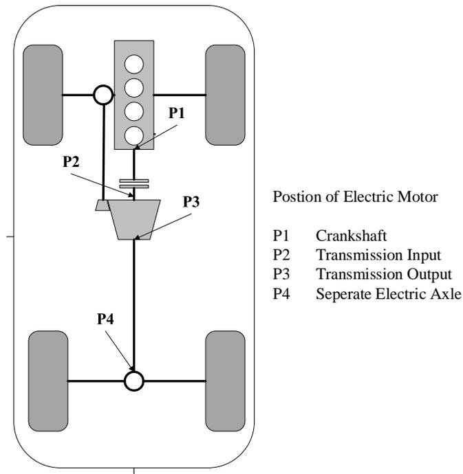
Figure 30: Position of Electric Motor Integration, when converting a Conventional All-Wheel Drive Layout to a Parallel Hybrid (P1-4).
