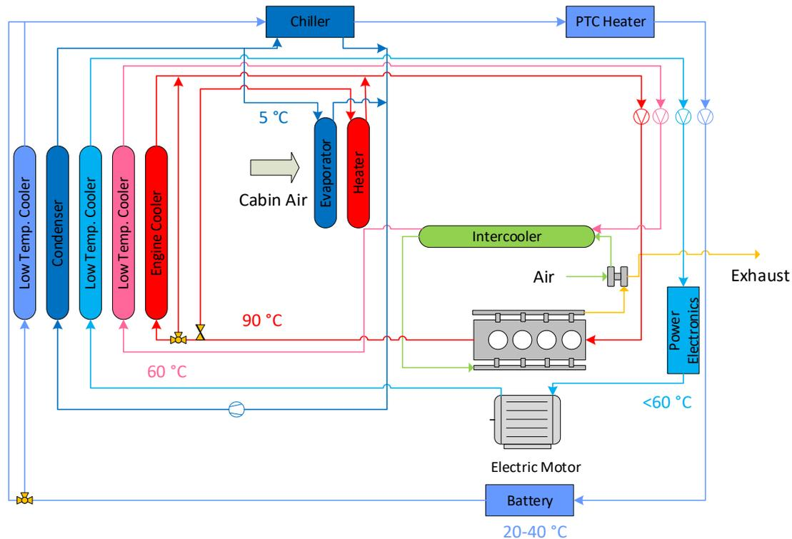
Figure 21: Thermal Management for Hybrid Vehicles (cf. Wawzyniak et al., 2017)
