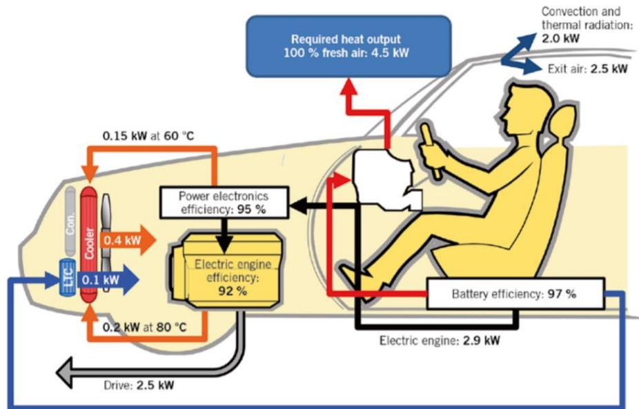
Figure 24: Energy Flow in a Battery Electric Vehicle. (Jung et al., 2011)
