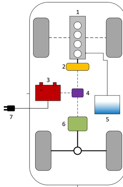
Figure 1: Series Hybrid. 1 combustion engine, 2 generator, 3 traction battery, 4 power electronics, 5 tank, 6 electric machine, 7 power plug. (cf. Tschöke, 2014)
