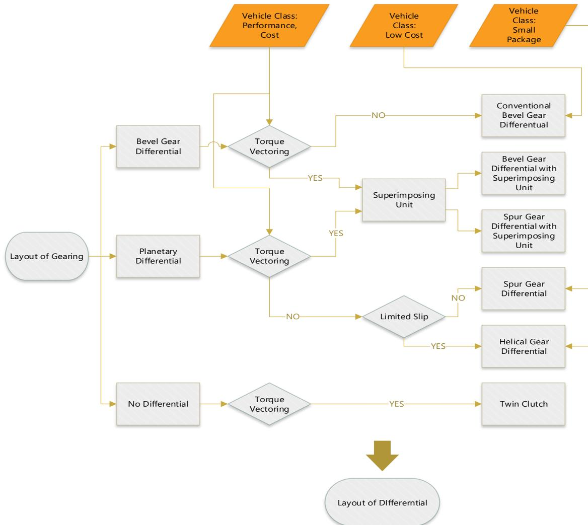
Figure 50: Layout Options of Electric Axle Differentials.
