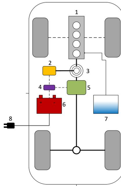
Figure 4: Power-Split or Combined Hybrid. 1 combustion engine, 2 generator, 3 planetary gearbox, 4 power electronics, 5 electric motor, 6 traction battery, 7 tank, 8 power plug. (cf. Tschöke, 2014)
