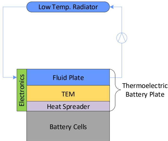
Figure 27: Elements of a Thermoelectric Battery Plate. (cf. Wehowski et al., 2015)
