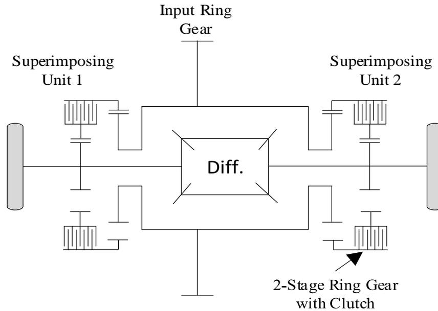
Figure 43: Schematic View of an Asymmetric Ring Gear Superimposing Unit. (cf. Meissner et al., 2010)
