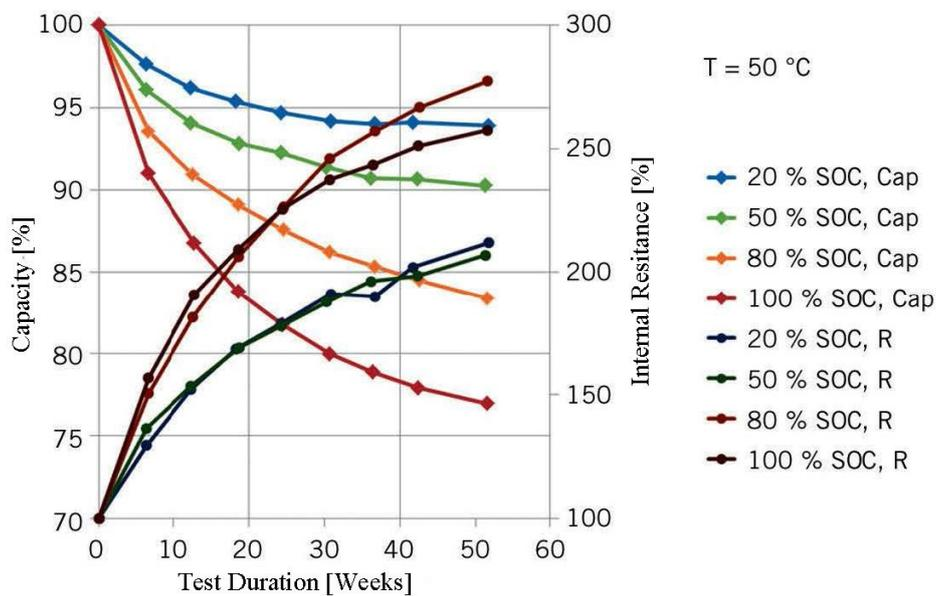
Figure 18: Aging of a Li-Ion cell in regards to capacity and internal resistance depending on SOC. (Ecker and Sauer, 2013)
