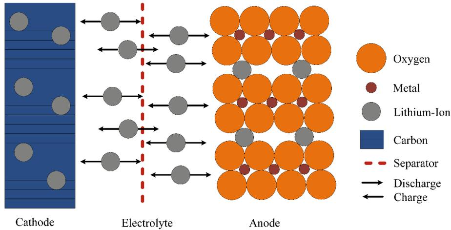
Figure 17: Schematic layout of a li-ion cell. (Ecker and Sauer, 2013)
