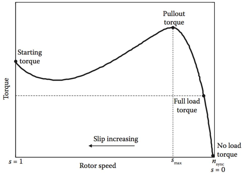
Figure 12: Torque-speed characteristic of an IM. (Emadi, 2014)
