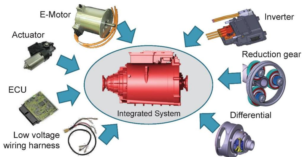
Figure 29: Integration of Components into an Electric Axle. (Schermann, 2015)
