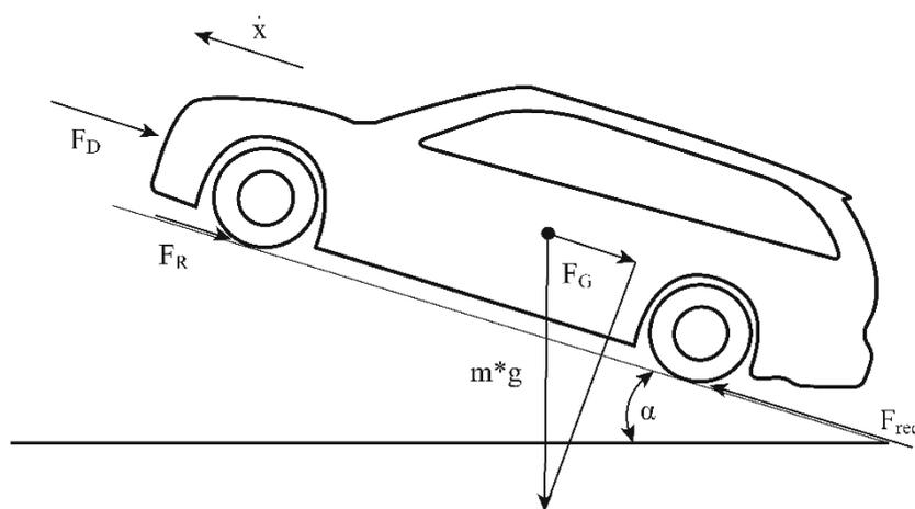
Figure 46: Resistance of Motion of a Vehicle. (Fischer et al., 2016)
