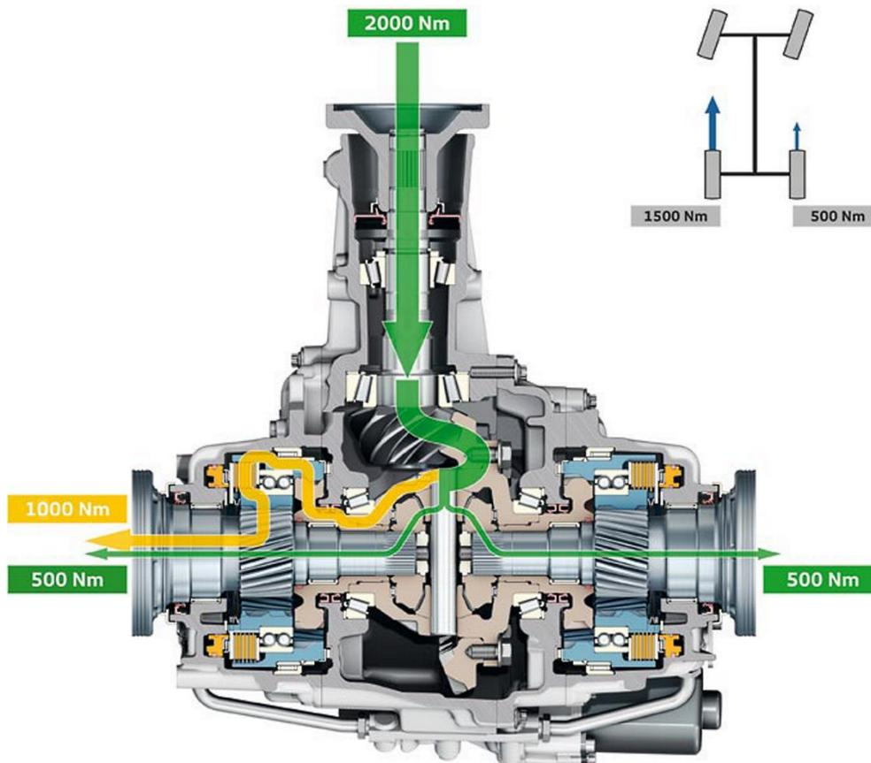
Figure 44: Cross Section of the Audi Sport Differential with Torque Vectoring. (Meissner et al., 2010)
