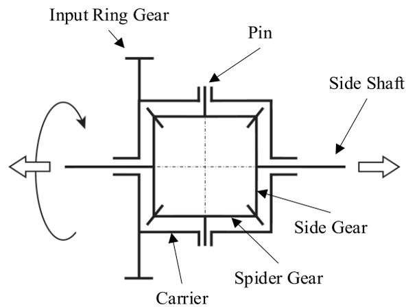
Figure 34: Schematic view of a differential. (Fischer et al., 2016)
