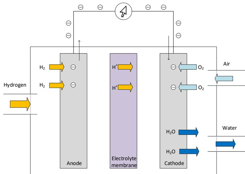
Figure 7: Polymer Electrolyte Membrane (PEM) Fuel Cell
