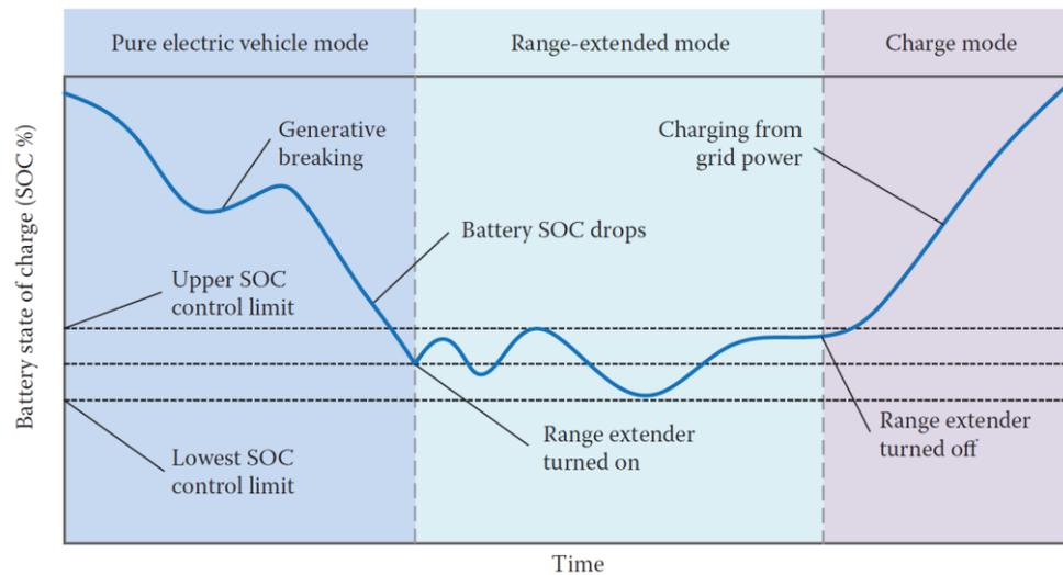
Figure 5: Range-extended electric vehicle operating modes. (Emadi, 2014)
