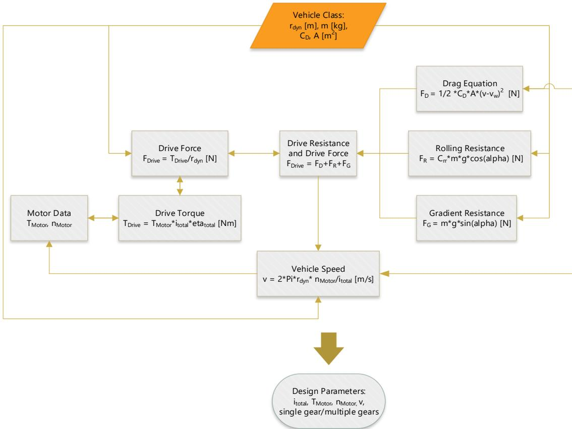
Figure 47: Selection of the Basic Design Parameters of an Electric Axle.
