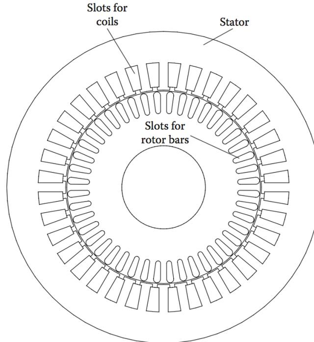
Figure 11: Cross-section view of a squirrel-cage induction machine. (Emadi, 2014)
