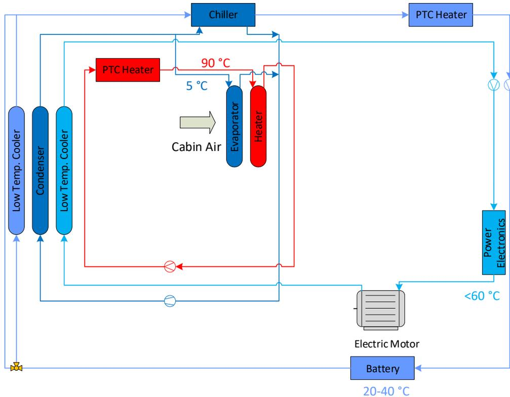
Figure 22: Thermal Management of a BEV with PTC Heater. (cf. Wawzyniak et al., 2017)
