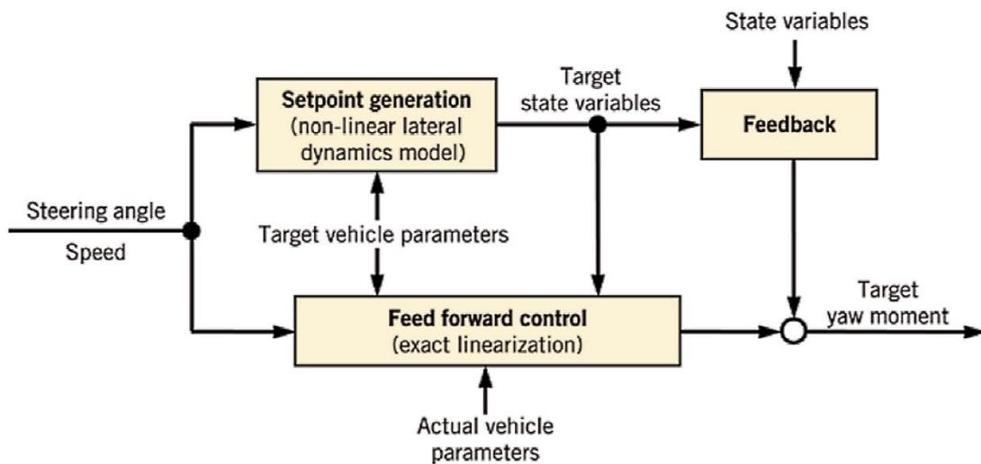
Figure 41: Torque Vectoring Control Algorithm. (Folke et al., 2010)
