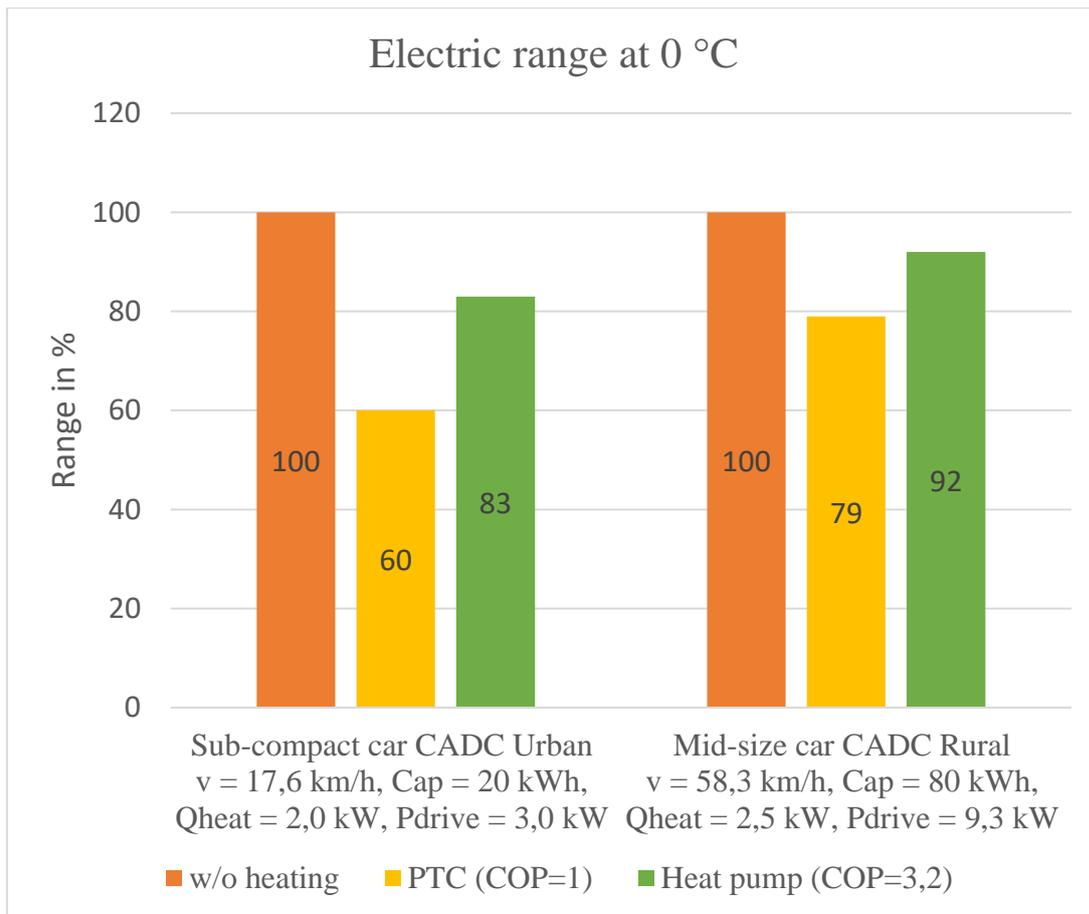
Figure 26: Electric range of BEVs at 0 °C ambient air temperature. (cf. Wawzyniak et al., 2017)
