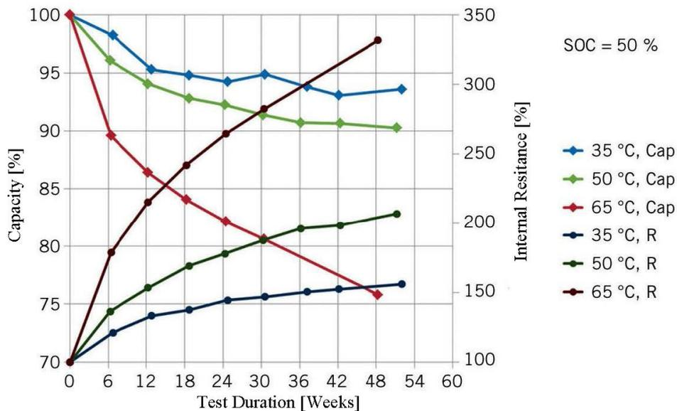
Figure 20: Typical development of capacity (Cap) and inner resistance (R) of a li-ion battery with 50% SOC at different temperatures. (Ecker and Sauer, 2013)
