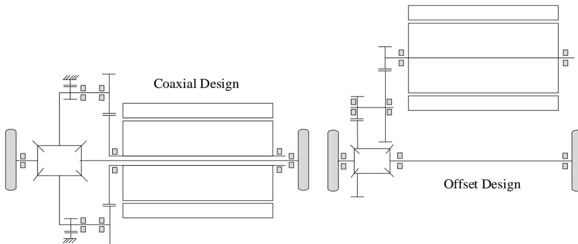
Figure 33: Dimensional Comparison between Coaxial and Offset Design.
