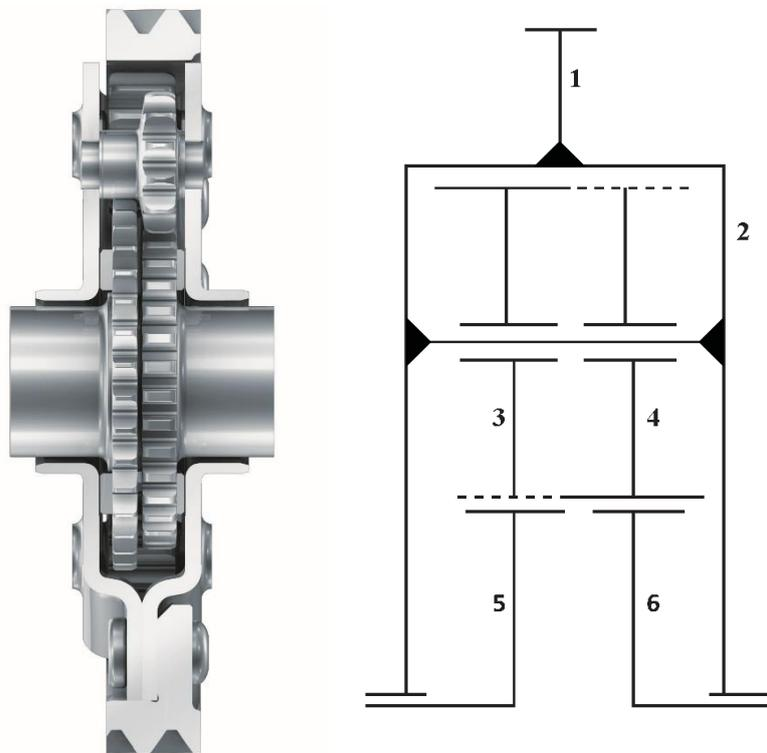
Figure 37: Asymmetric Spur Gear Differential with Input Gear (1), Housing (2), Planets (3, 4) and Sun Gears (5, 6). (Smetana and Biermann, 2011) & (Biermann et al., 2010)
