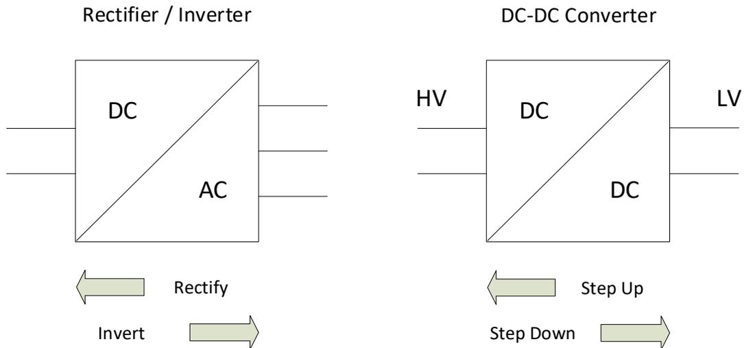
Figure 13: Transformation types of electrical energy. (cf. Hofmann, 2014)
