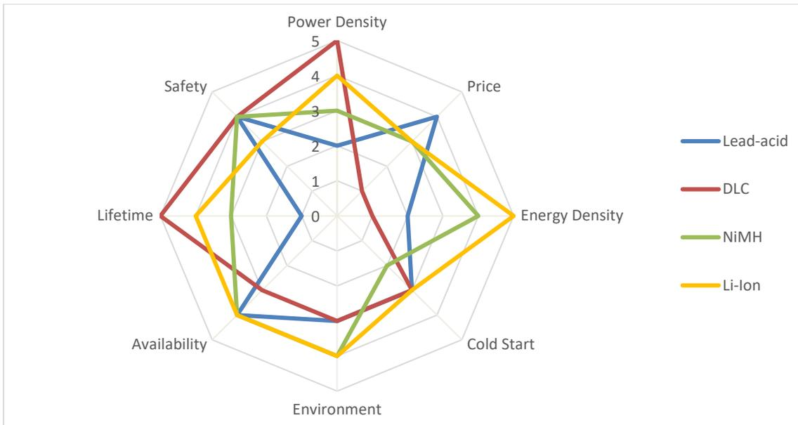
Figure 16: Evaluation of different energy storage systems for automotive application from bad (1) to good (5).(cf. Keller et al., 2009)
