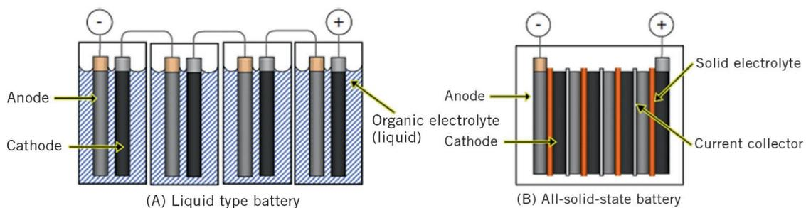
Figure 19: Conventional li-ion battery and stacked solid-state li-ion battery. (Yada and Brasse, 2014)
