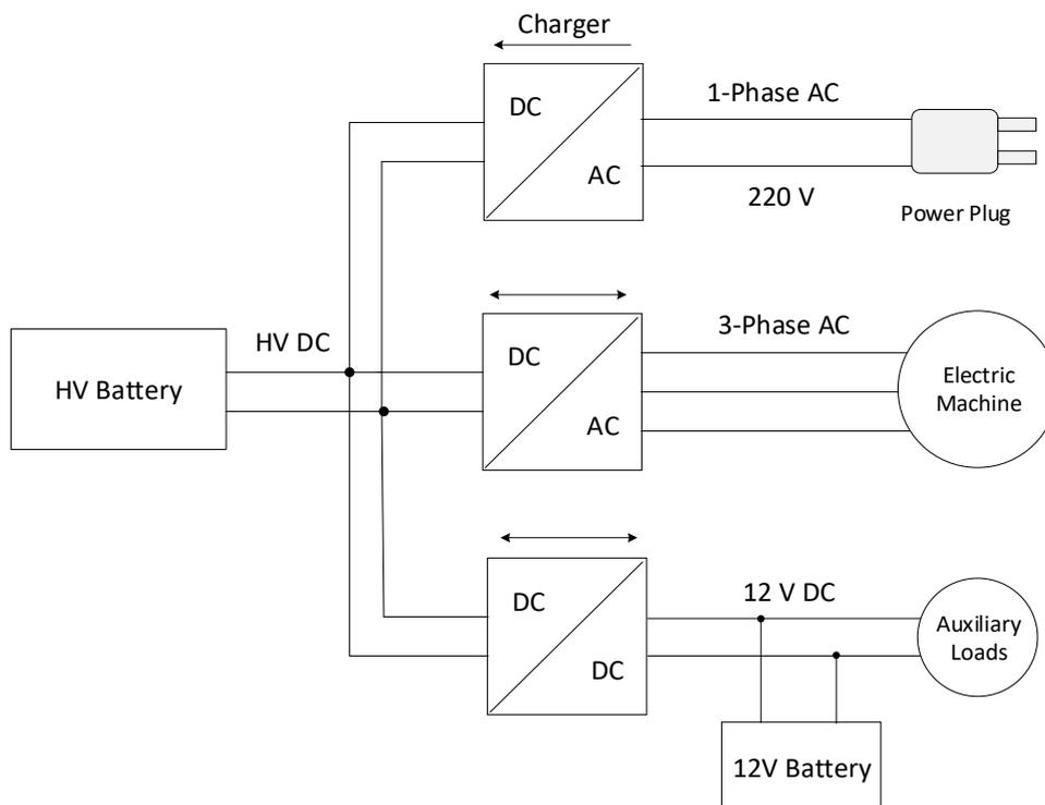
Figure 14: Power electronics in a BEV or PHEV. (cf. Hofmann, 2014)
