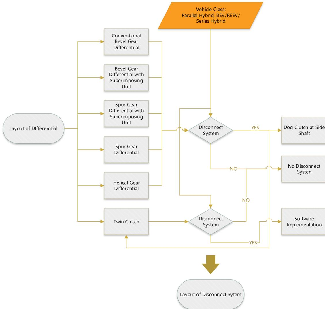
Figure 51: Layout Options for the Implementation of a Disconnect System into an Electric Axle.
