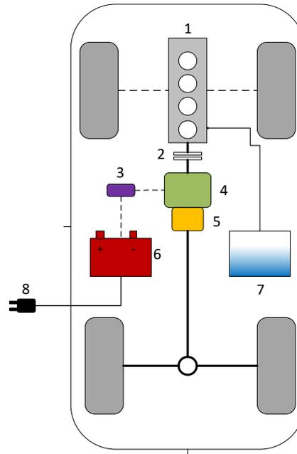
Figure 2: Parallel Hybrid. 1 combustion engine, 2 coupling, 3 power electronics, 4 electric machine, 5 generator, 6 traction battery, 7 tank, 8 power plug. (cf. Tschöke, 2014)
