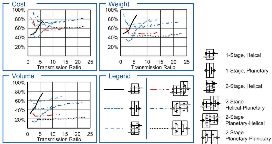
Figure 49: Comparison of different Gearing Designs in respect to Cost, Weight and Volume. (Klocke and Brecher, 2016)
