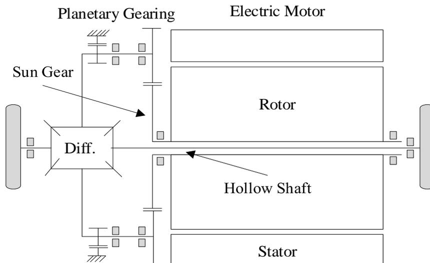
Figure 31: Schematic Layout of Gearing and Electric Machine of a Coaxial Electric Axle.
