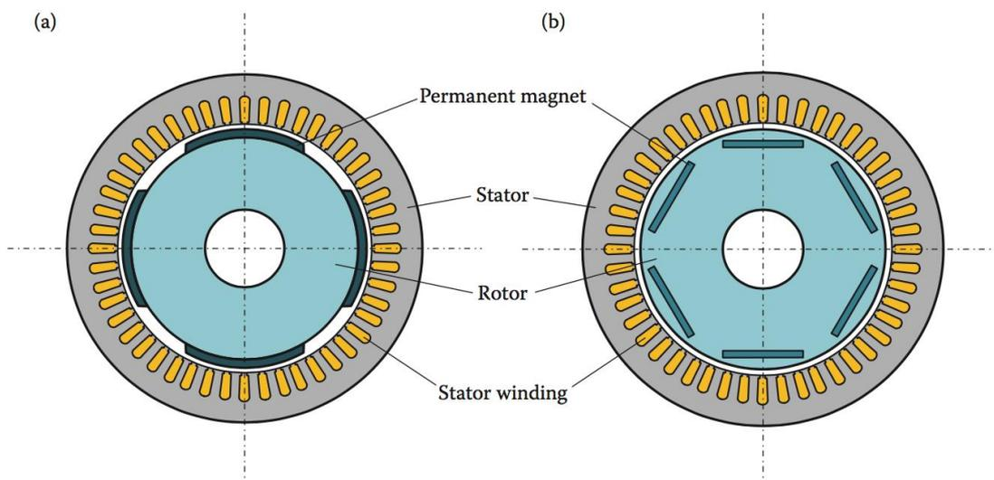
Figure 9: Cross section view of PM machines (a) surface permanent magnet machine (SPM), (b) interior permanent magnet machine (IPM). (Emadi, 2014)
