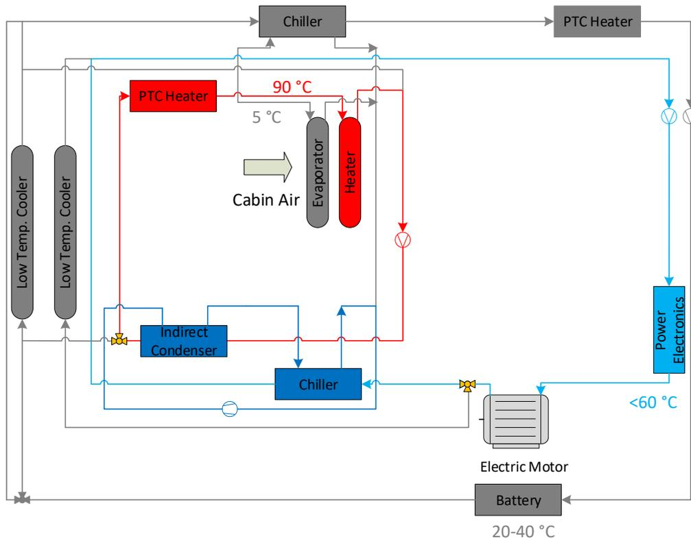
Figure 23: Thermal Management of a BEV with a heat pump, during heating condition. (cf. Wawzyniak et al., 2017)
