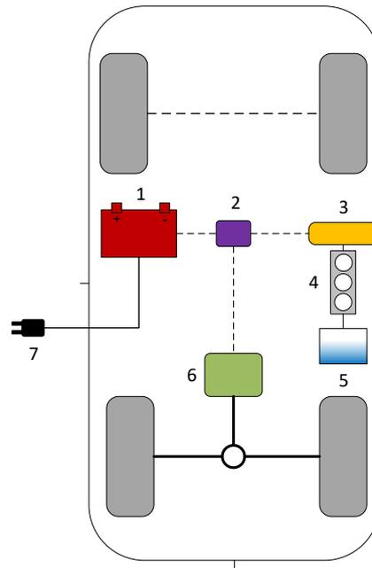
Figure 6: Thermal Range Extender. 1 traction battery, 2 power electronics, 3 generator, 4 combustion engine, 5 tank, 6 electric motor, 7 power plug. (cf. Tschöke, 2014)
