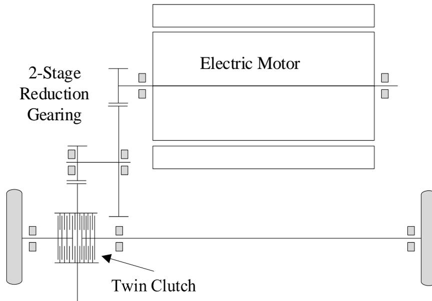
Figure 39: Schematic view of an E-Axle with Twin Clutch and Reduction Gearing.
