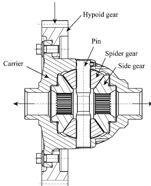
Figure 35: Cross section of an axle differential. (Fischer et al., 2016)
