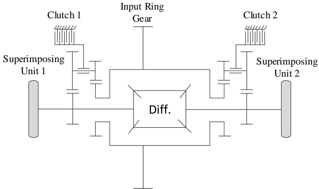
Figure 42: Schematic View of an Axle with a TV Superimposing Unit.
