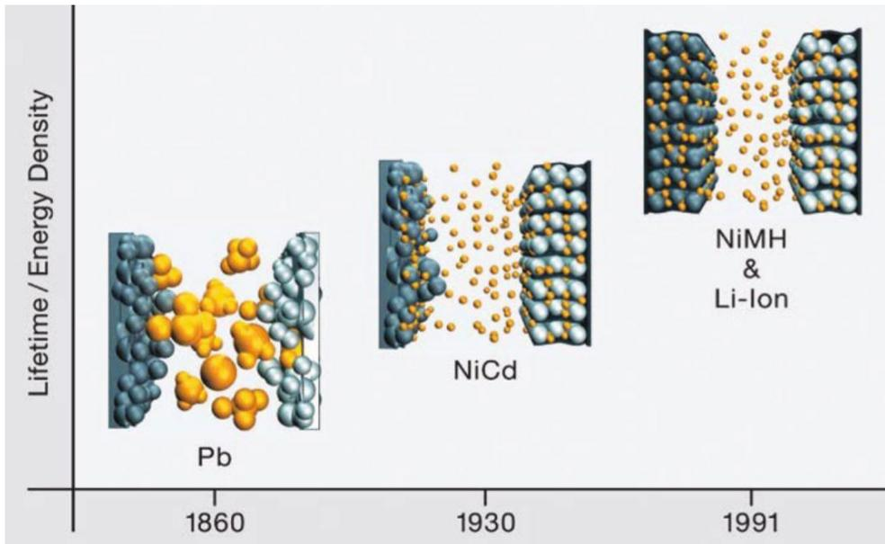
Figure 15: The way from conversion to intercalation electrodes. (Keller et al., 2009)
