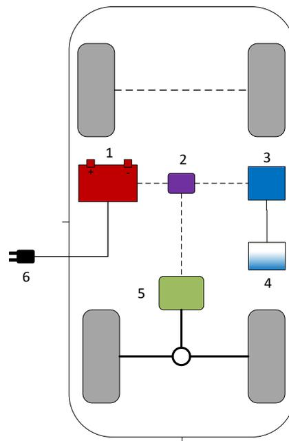
Figure 8: Chemical Range Extender. 1 traction battery, 2 power electronics, 3 fuel cell, 4 hydrogen tank, 5 electric motor, 6 power plug. (cf. Tschöke, 2014)
