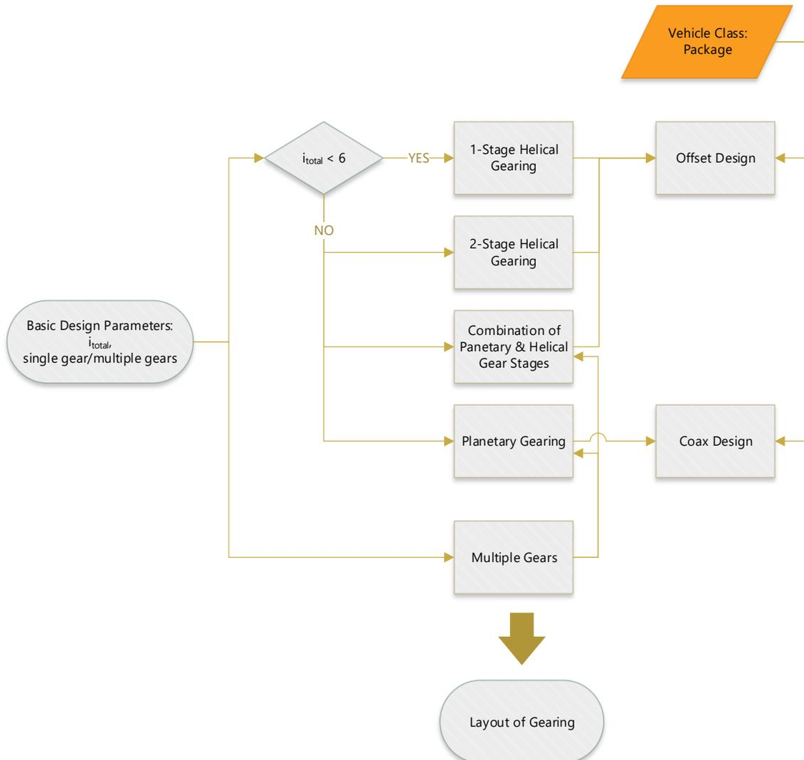
Figure 48: Mechanical Layout of the Gearing of an Electric Axle.
