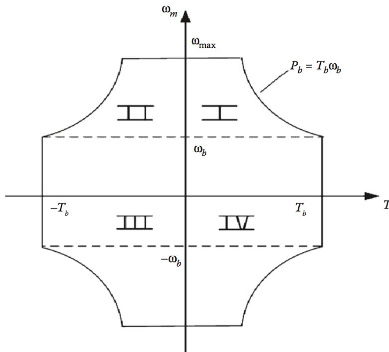
Figure 10: Four-quadrant operation of a PMSM. (Emadi, 2014)
