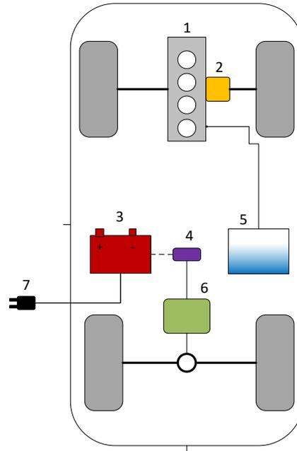
Figure 3: Axle-Split Hybrid. 1 combustion engine, 2 conventional gearbox, 3 traction battery, 4 power electronics, 5 tank, 6 electric machine, 7 power plug. (cf. Tschöke, 2014)
