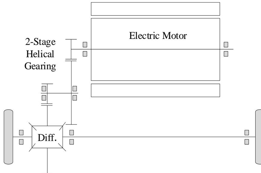
Figure 32: Schematic Layout of an Electric Axle with Offset Layout.
