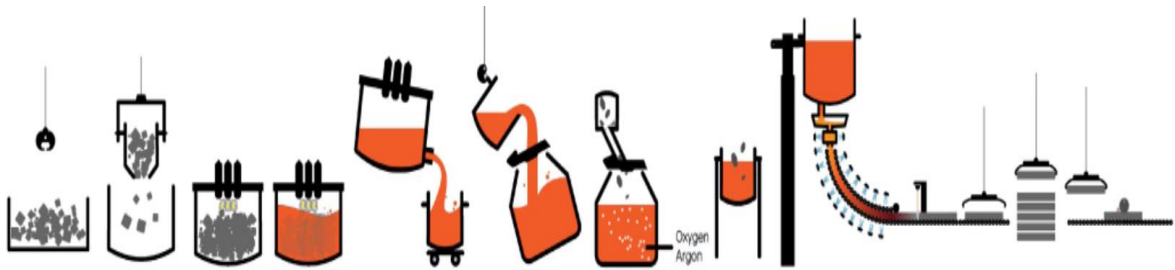
Figure 4. Step 1. Manufacturing process of stainless steel the melt shop [28]
