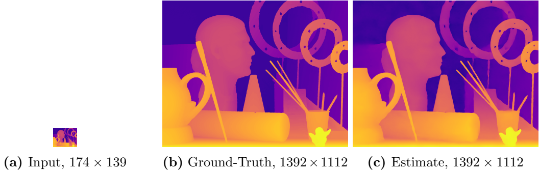
Figure 1.1: The depth super-resolution problem. Given a noisy, low-resolution depth map as input (a), the goal is to recover a plausible high-resolution estimate (b)-(c). The problem is ill-posed because infinitely many high-resolution depth maps can map the noisy, low-resolution input.
