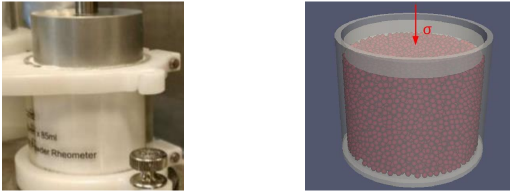
Figure 11: Compressibility module of the FT4 rheometer (left) and simulation of the compressibility testing (right)
