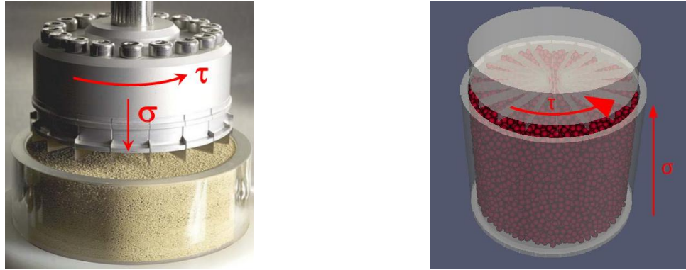
Figure 9: Shear cell module of the FT4 rheometer (left) and model of the rotational shear test (right)
