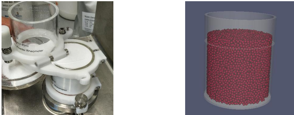
Figure 6: Filled vessel at FT4 experiment (left) and DEM simulation (right)
