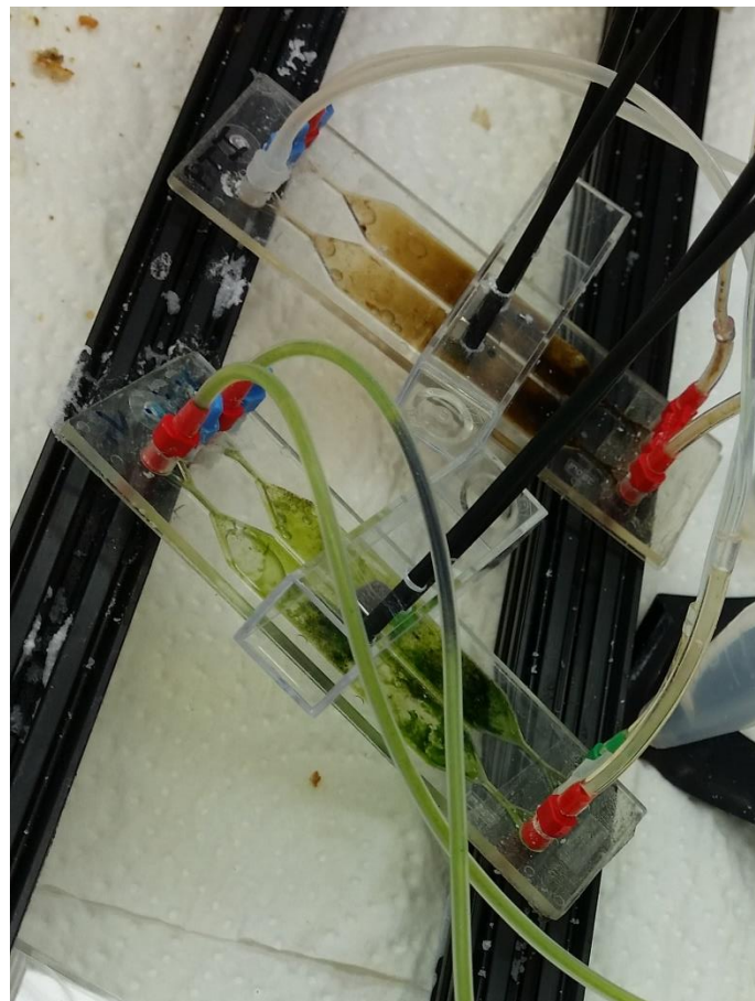
Illustration 28: Green and flint algae after 3 months of cultivation in 250 \mu l rhombic chamber chips
