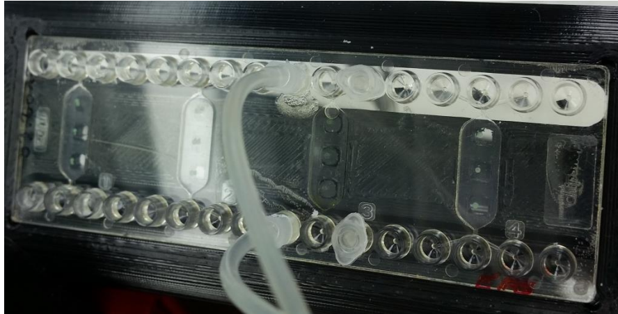
Illustration 26: 20 µl rhombic chamber chips for the examination of the conjunction between the fall of pO_2 and cell number
