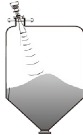
Figure 23: Non-contact Radar technology placed over the hopper.
