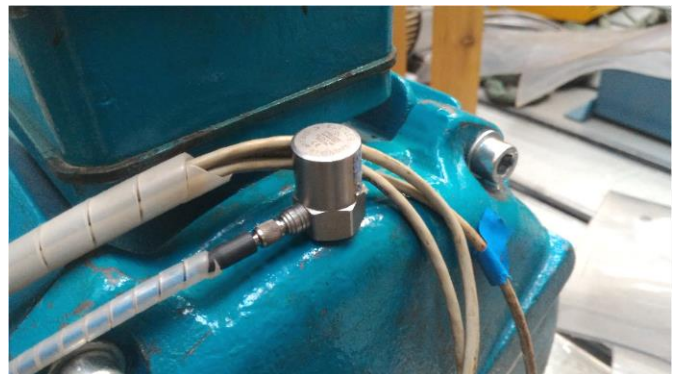
Fig. 1. Accelerometer attachment view.
