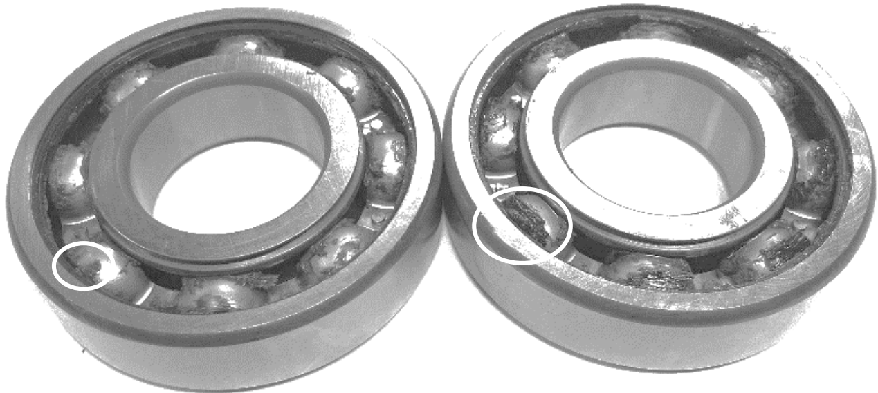
Fig. 1. Used bearings: non drive-end(left) and drive-end (right) with the sampled areas marked by white circles.
