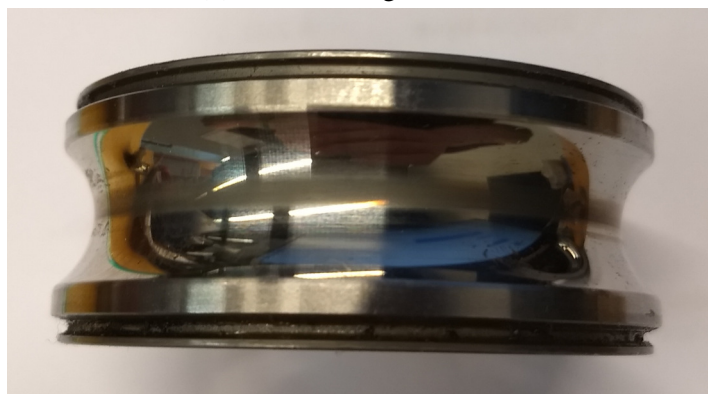
(c) Pitting damage on bearing inner race.
