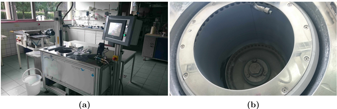
Figure 22. A Dynamic Sheet Former located at Sappi Gratkorn was used to produce oriented sheets. In (a) the entire device together with a laboratory roll press in the background is shown. (b) provides a close-up of the rotational forming wire and the traversing application nozzle.
