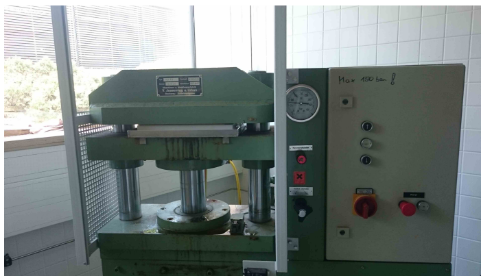
Figure 18. Hydraulic press used to variate paper density on three levels: 1) not pressed 2) pressed with 75 bar 3) pressed with 150 bar.
