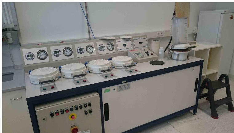
Figure 16. Production of handsheets for five out of six trials was entirely realised on a Rapid-Köthen-Sheetformer.
