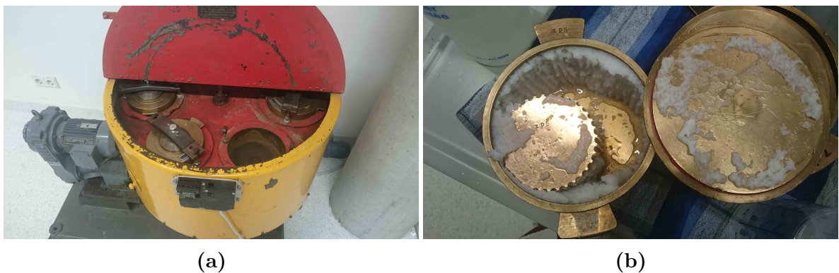
Figure 19. Secondary fines of Santa Fe Eucalyptus kraft pulp were created by beating the pulp in a (a) jokro mill for one hour. The beating body of this device is freely movable within the (b) beater box.
