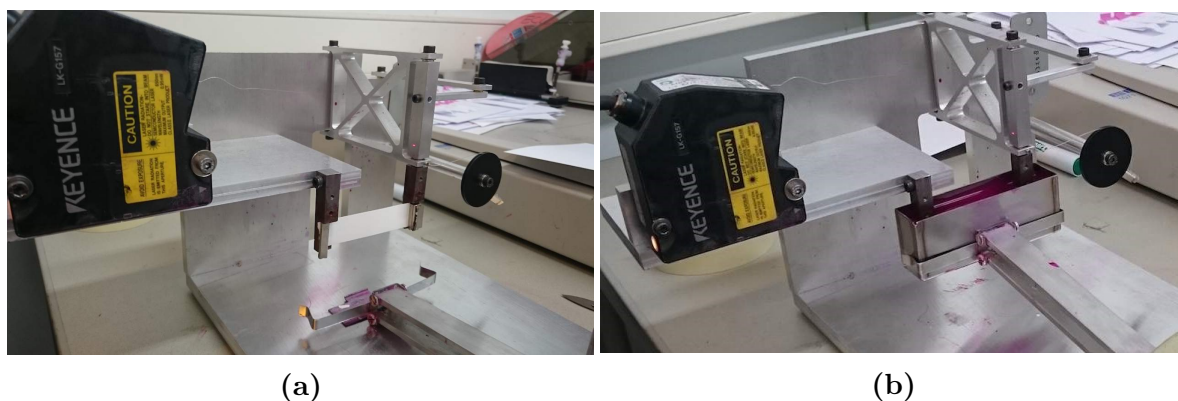
Figure 43. Hydroexpansion in ink was investigated on a simple setup. A paper specimen was clamped onto two sample holders (a), one of them preloaded with a tiny weight of 1.72 g. The sample was then immersed into ink (b) recording the expansion by a laser sensor.
