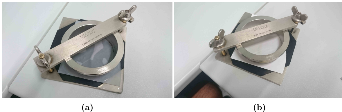
Figure 21. Degree of sizing was measured by a Cobb 60 test. No representative value was achieved by testing unsized papers (a) due to an instant total penetration. In contrast, (b) sized papers showed an appropriate water repellency.
