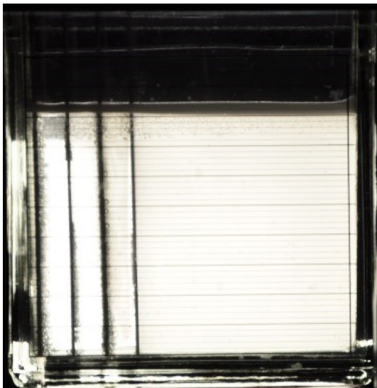
Figure 12.28.: Electric splitting experiment using four plate electrodes after 3 hours at an electric field strength of 300 V/m
