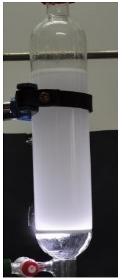
Figure 12.6.: Pressurized air flotation at t=0
