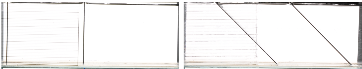
(a) Initial picture of an experiment using two vertical electrodes (b) Initial picture of an experiment using two inclined electrodes with CaAn configuration
