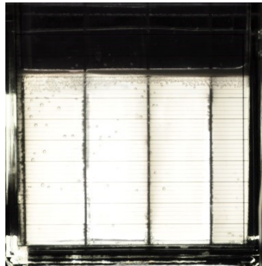
Figure 12.29.: Electric splitting experiment using four plate electrodes after 3 hours at an electric field strength of 200 V/m
