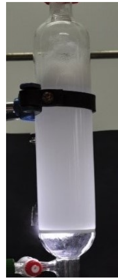
Figure 12.7.: Pressurized air flotation at t=35 min
