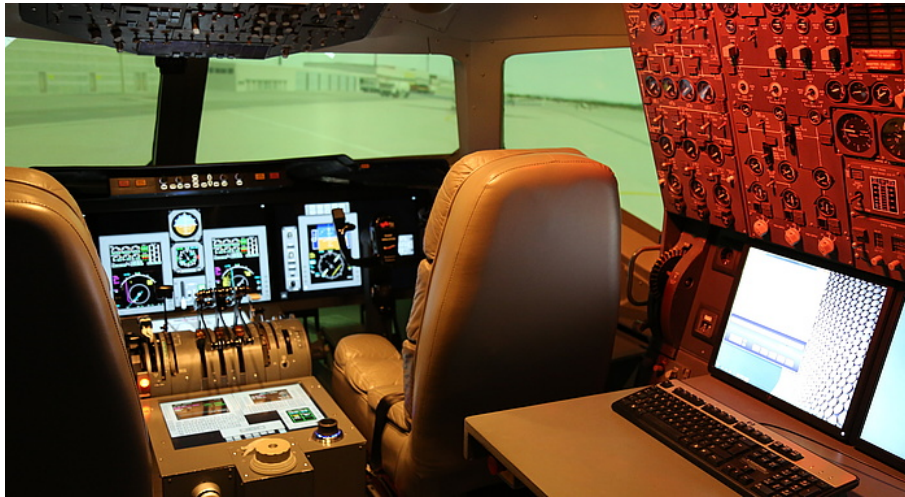
Figure 2.2: Research flight simulator of TU Graz (fixed base, widebody aircraft) © TU Graz
