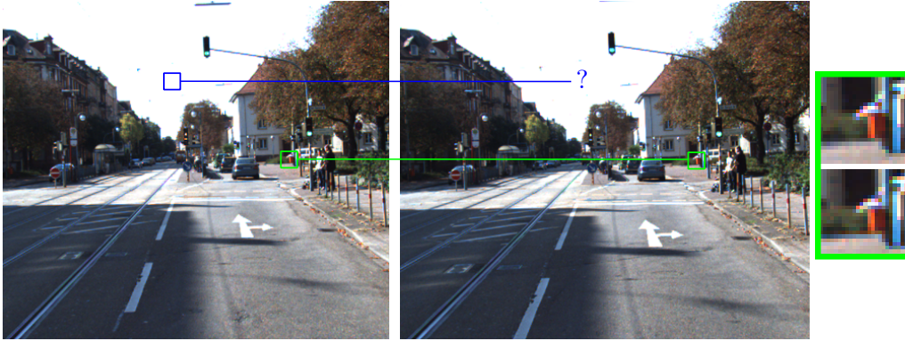
Figure 1.2: Corners and high-contrast texture help to make the correspondence unique (green patches). In homogeneous regions, the problem is ambiguous (blue patch).
