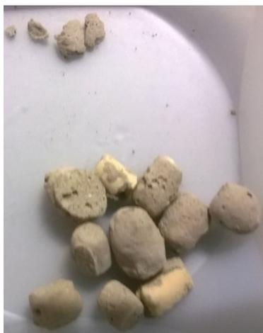
*Figure 11: Coated alumina oxide pellets*
