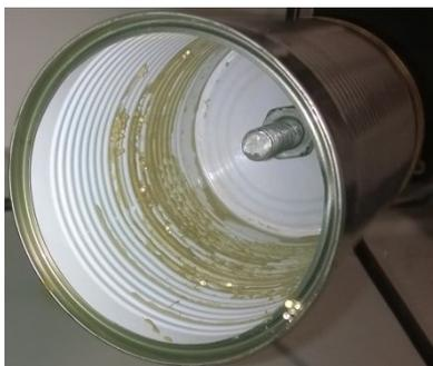
Figure 37: Drum granulator
