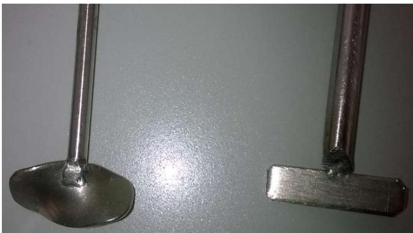
Figure 36: Used stirrer for agglomeration, left: axial stirrer, right: radial stirrer
