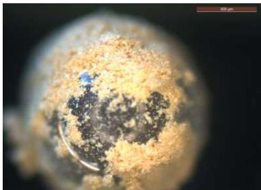
*Figure 8: Glass pellets rolled in catalyst*
