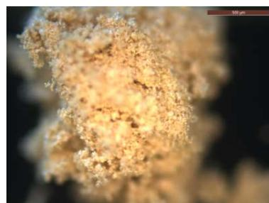
*Figure 6: Catalyst particles with alginic acid sodium salt as binder*
