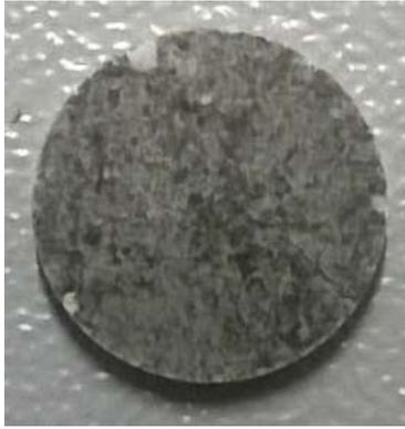
Figure 13: Tablet with die 8 mm
