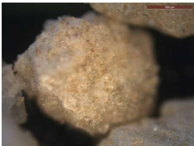
*Figure 12: Sintered catalyst on gravel*
