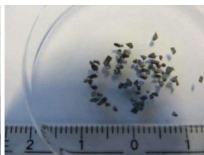
*Figure 19: Tablet 2:1 (catalyst:binder), milled with peppermill*
