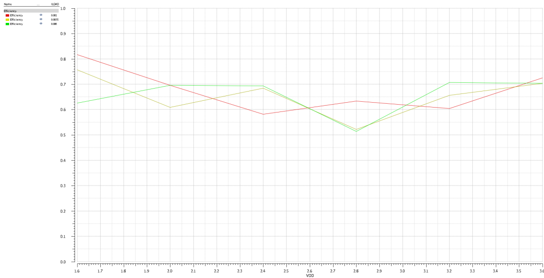
Figure 4.24: Efficiency of the converter over the whole input voltage range.
