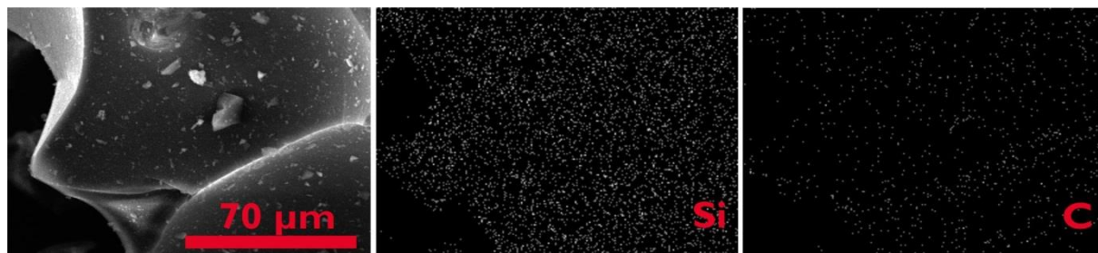
Figure 36 EDX Elemental mapping of 1-naphthyl 2 SiH 2 pyrolysed at 700 °C.
