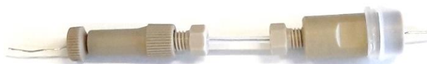
Figure 45 Setup for the metal wire sealing (interim solution) with 2 HPLC fittings and connecting PTFE tubing.
