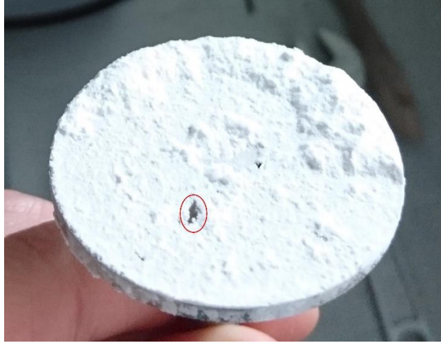
Figure 9: Photograph showing the fracture surface, created by a tensile test according to (Schweiger & Zimmermann 1998) .
