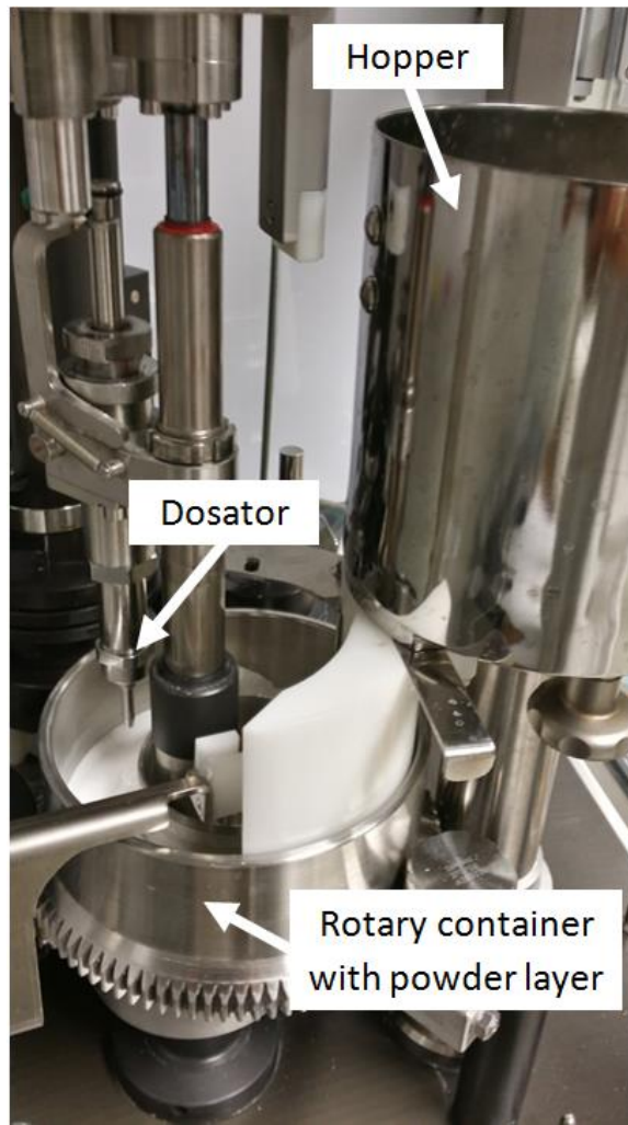
Figure 2: Sketch showing the rotary container with the powder layer, the hopper and the dosator.
