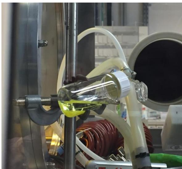
Figure 23: Set up of the crystallization, tilted vial with crystallized yellowish  $\text{SnI}_2(\text{DMF})$  complexes
