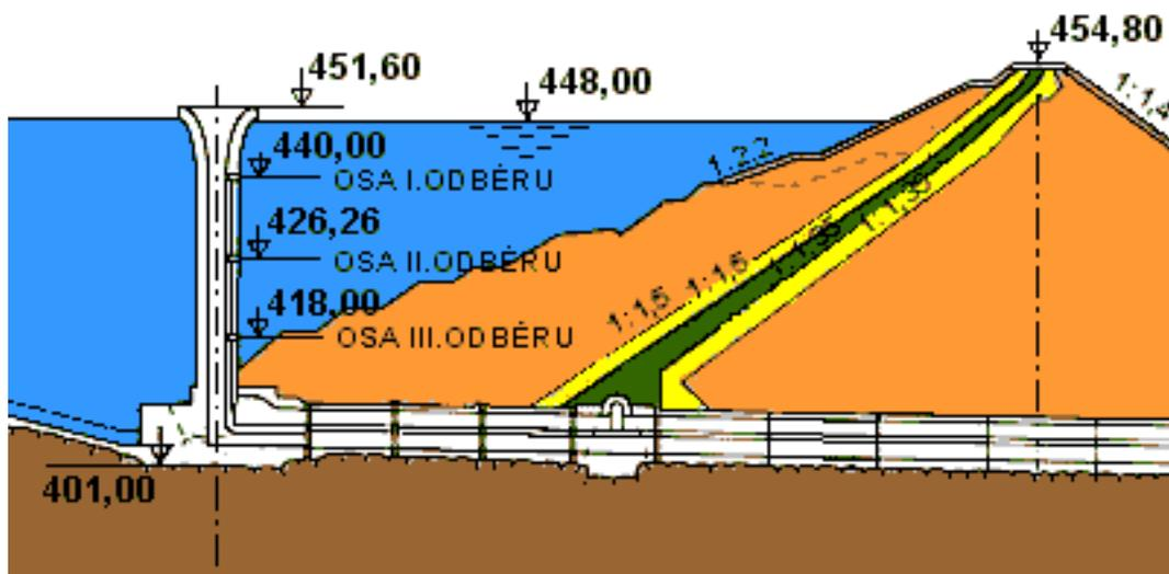
Fig. 1 Jirkov Dam bell-mouth spillway
