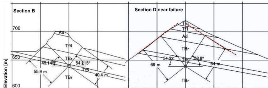
Fig. 2 : Cross sections at minimum cover and near failure
