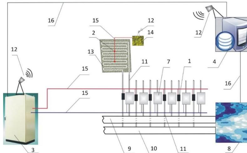
1 interpolated digital temperature measuring device; 2 pre-embedded digital temperature sensor; 3 control cabinet; 4 sever of control; 5 two-way intelligent control valve; 6 flow meter; 7 integrated control device of temperature and flow; 8 pump; 9 main inlet pipe; 10 main outlet pipe; 11 branch inlet pipe; 12 wireless transmitting bridge; 13 mobile multi-point device of displacement acquisition; 14 concrete section; 15 connecting cable of flow and temperature collection; 16 optical fiber cable
