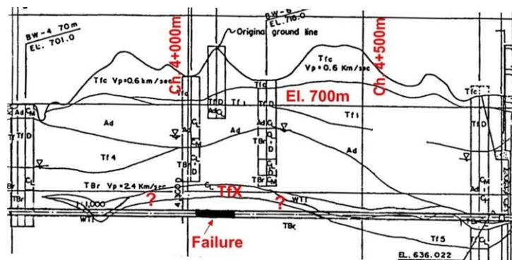
Fig. 1: Longitudinal geological section near the failure
