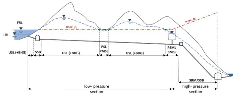
Fig 1: Longitudinal section of a typical Alpine high head power plant, Legend see Tab.1
