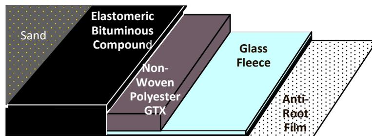
Fig. 1. Typical structure of a bituminous geomembrane
