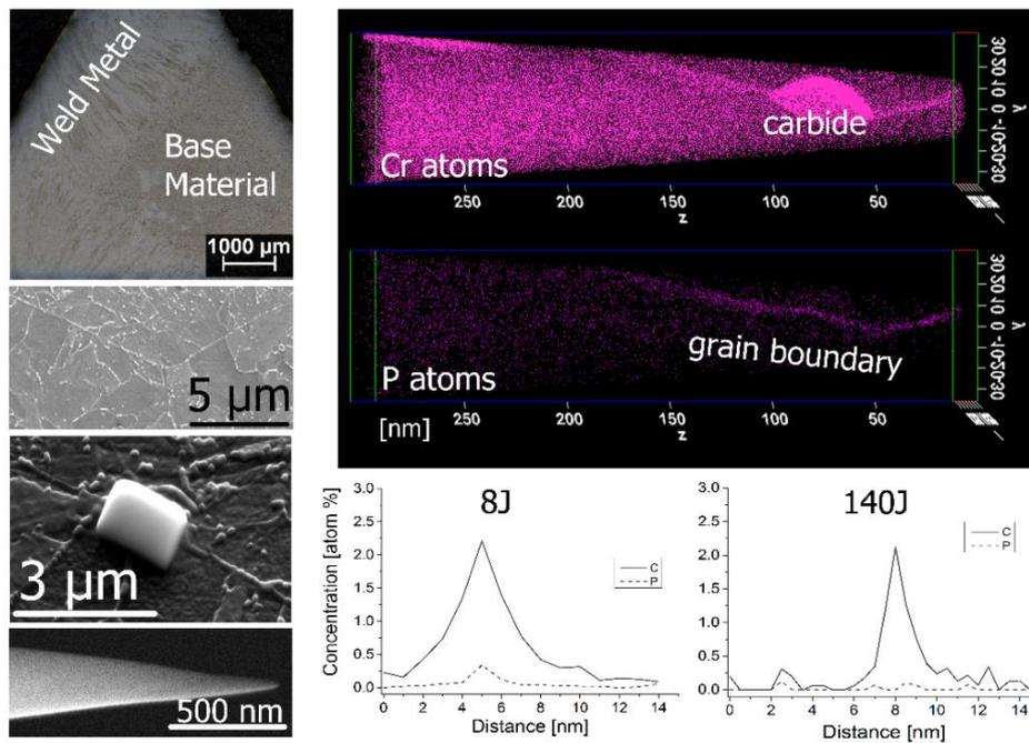
participate in the metal–metal bonds and they are weakened. By the application of a RTE treatment around 600°C, diffusion of the impurities elements occurs faster because segregation starts at lower temperatures (around 550°C). During RTE treatment, the diffusion is much faster, producing the fast recovery of toughness.
