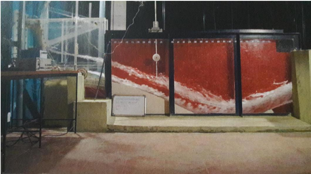
Fig. 1 Model set up for testing of or spillway profile and air demand in an orifice spillway
