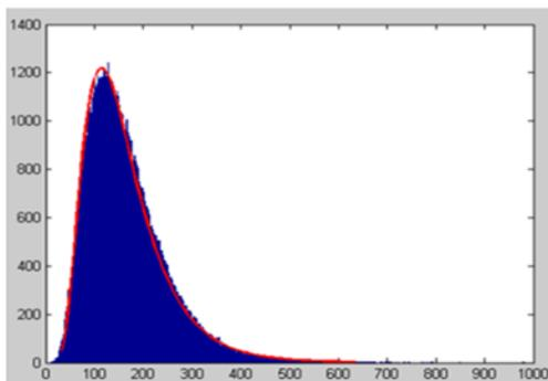
Figure1: Frequency diagram of ultimate bearing capacity of smooth foundation
