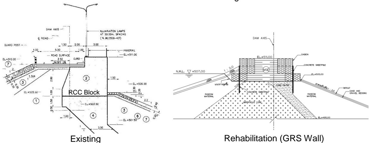
Fig. 3 Dam Crest Rehabilitation Detail
