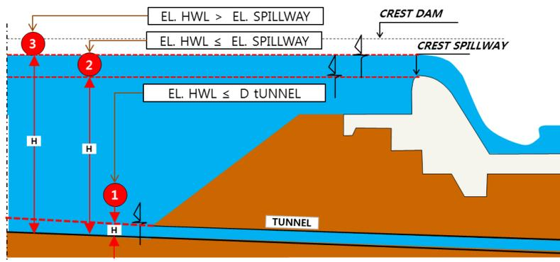
Fig. 2 The Concept of Dry Dam
