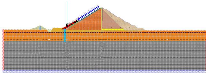
Fig. 2 FE mesh and model for the stress-strain analysis
