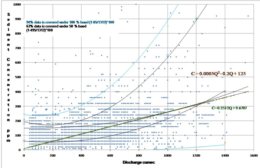
Fig. 1 Discharge and Sediment data used analysis
