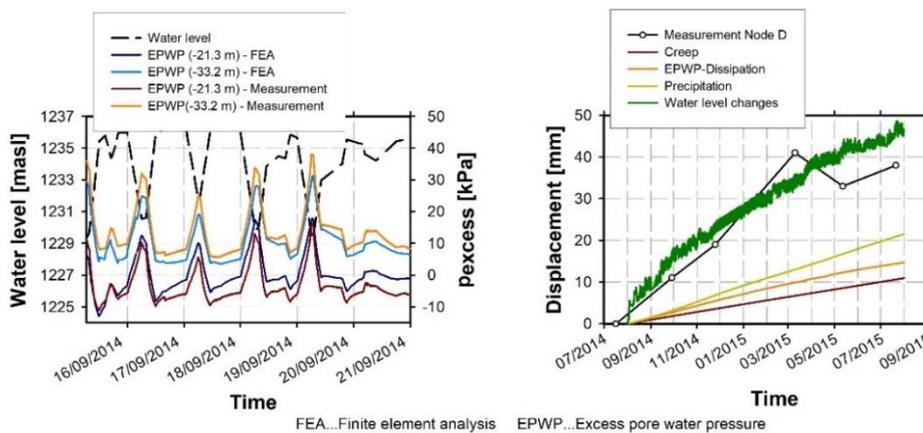
Fig. 2 Comparison of calculated and measured excess pore water pressures (left) and displacements (right)
