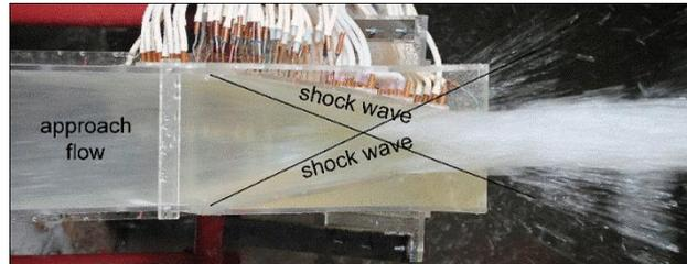
Fig. 1 Flow regime in the STED contraction section
