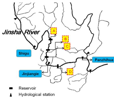
Fig. 1: Location of cascade reservoirs and hydrological stations (The 1st, 2nd and 3rd cascade reservoirs were located between the 1st and 2nd hydrological station, and the 4th reservoir lies between the 2nd and 3rd hydrological station)
