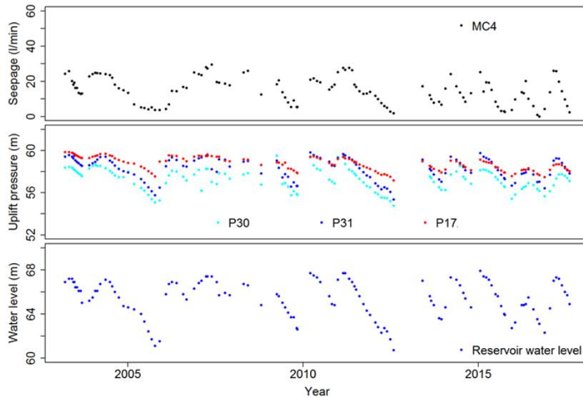
Fig. 1 - Seepage, uplift pressure and water level measured between 2003 and 2017
