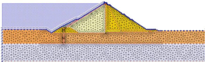
Fig. 1 FE mesh and model for the seepage analysis
