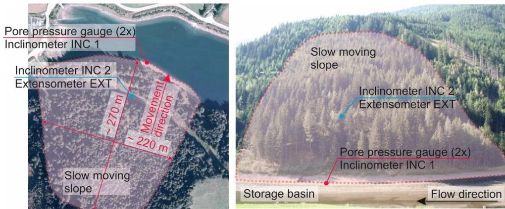
Fig. 1 Plan view and side view of water storage basin and slow moving slope
