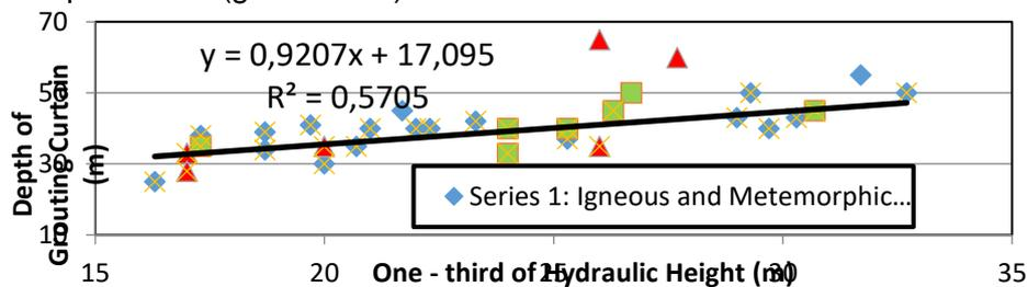
Figure 1. Direct relationship between gout curtain and hydraulic height for three different series
