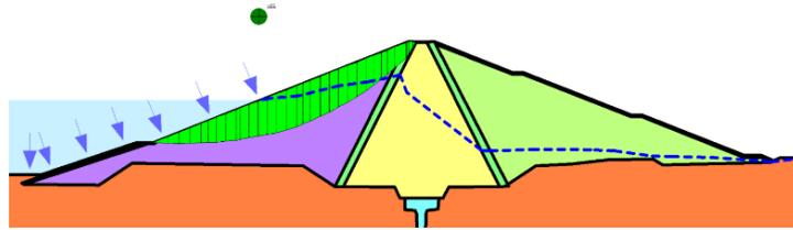
Fig. 1: Safety factor of upper slope in case of the discharge through the tunnel (gravel)
