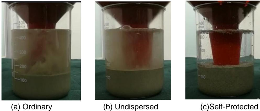
Fig. 1 Comparison among ordinary, undispersed and self-protected technology
