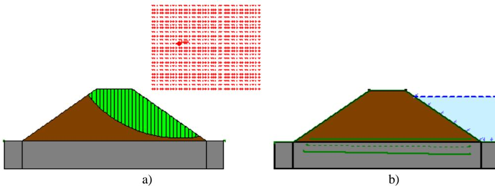
Fig. 24: Factor of safety in dynamic condition, a) Safety map b) model with tank
