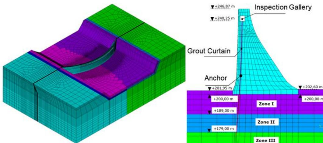
Fig. 1 Nonlinear 3D model of the dam and the foundation
