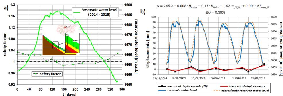
Fig. 2. a) Coupled transient seepage flow and stability analyses; b) Regression analyses
