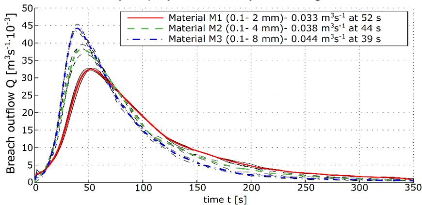
Fig. 1 Breach hydrographs using different shell Materials
