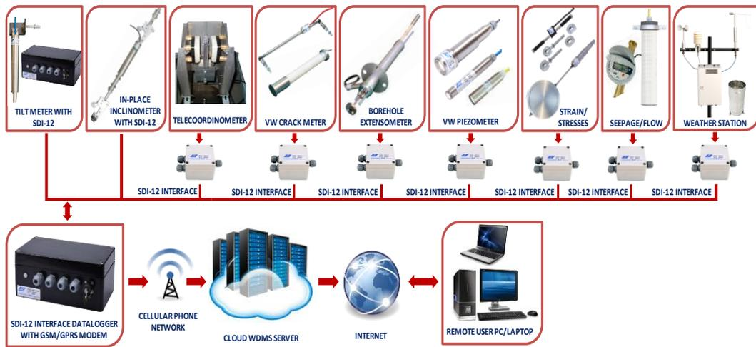
Fig.1 Dam monitoring instruments on an SDI-12 network
