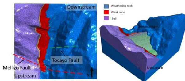
Fig. 2 Finite element numerical model-representation of the dam foundation and rockfill dam.
