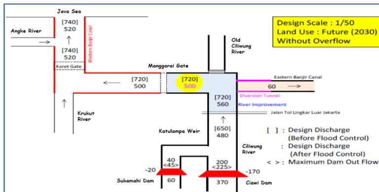
Fig. 1 The Masterplan Of Flood Control In Ciliwung River
