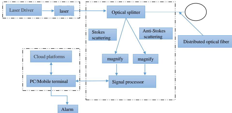
Fig.1 Distributed optical fiber intelligent temperature monitoring system
