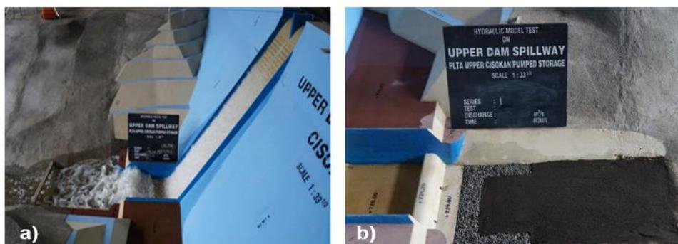
Fig. 1 (a) Stepped spillway model , (b) stone riprap for downstream protection
