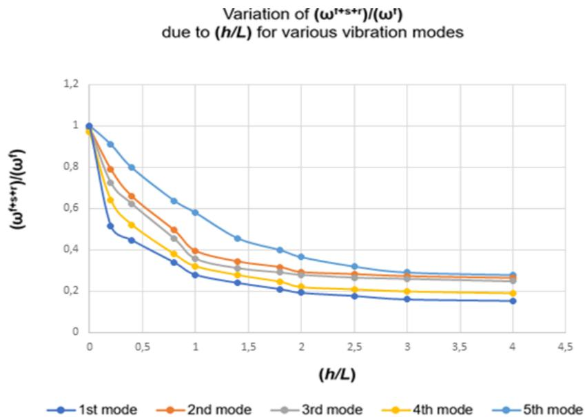
Fig 1. Results from the numerical models in Ansys, for various  $h / L$  and vibration modes.
