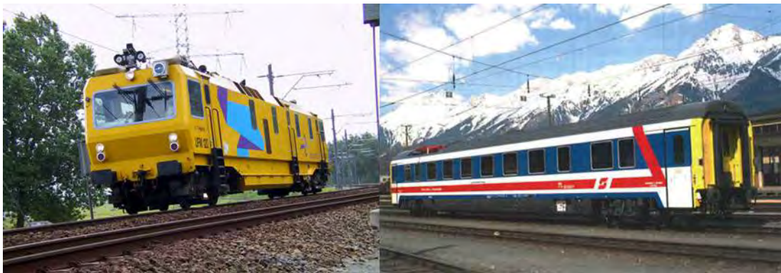
Figure 112 Recording cars: self-driving [left] [Plasser & Theurer 2013] or coupled to a train [right] [Hanreich 2004]
