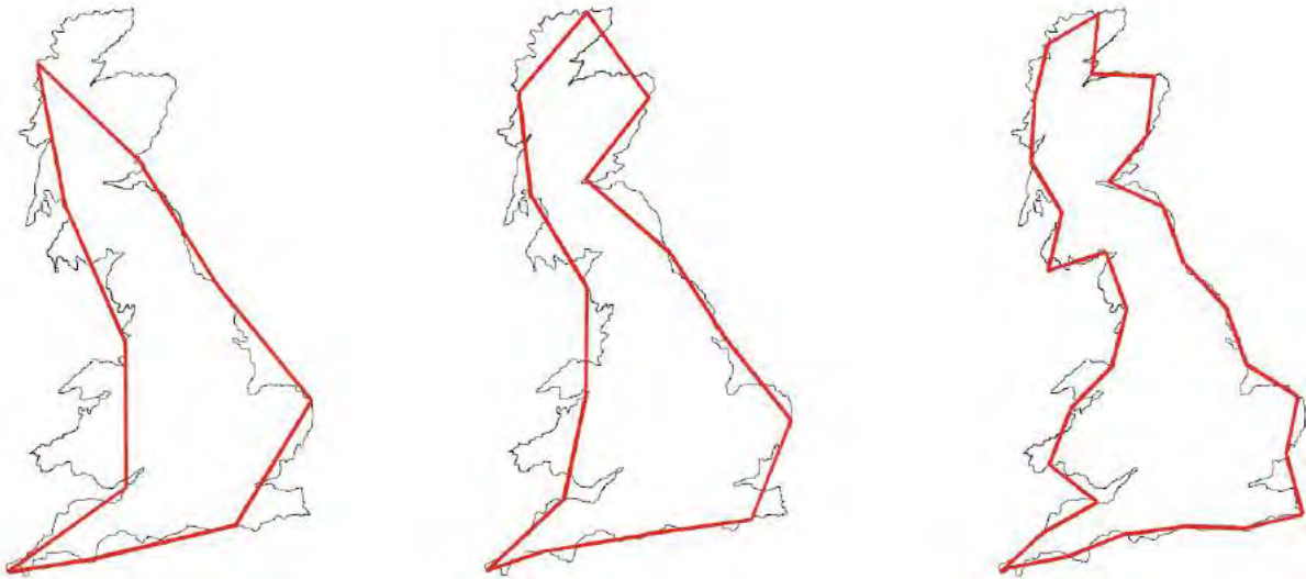
Figure 65 Describing the Length of Great Britain's Coastline with the help of the Modified Divider Length Method [Hyslip 2002a]
