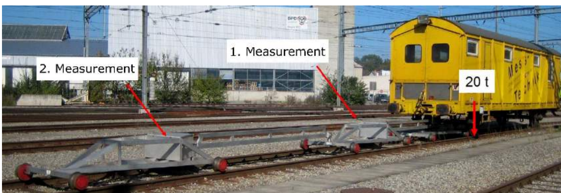
Figure 30 SBB subsidence test vehicle [according to Soldati 2013]
