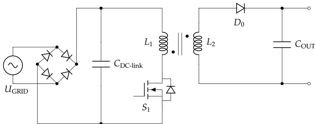
Figure 2.3: Principle schematic of the grid-connected Flyback converter.
