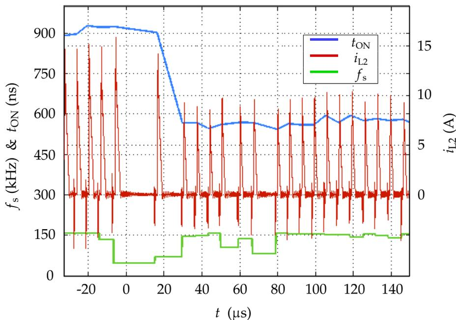
Figure 6.20: VOT reaction to jump from 60 % to 30 % load.
