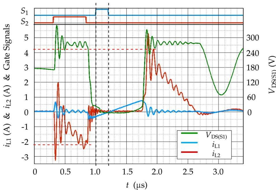
Figure 7.14: Circulating energy due to  $C_{\text{OSS}(S1)}$ .
