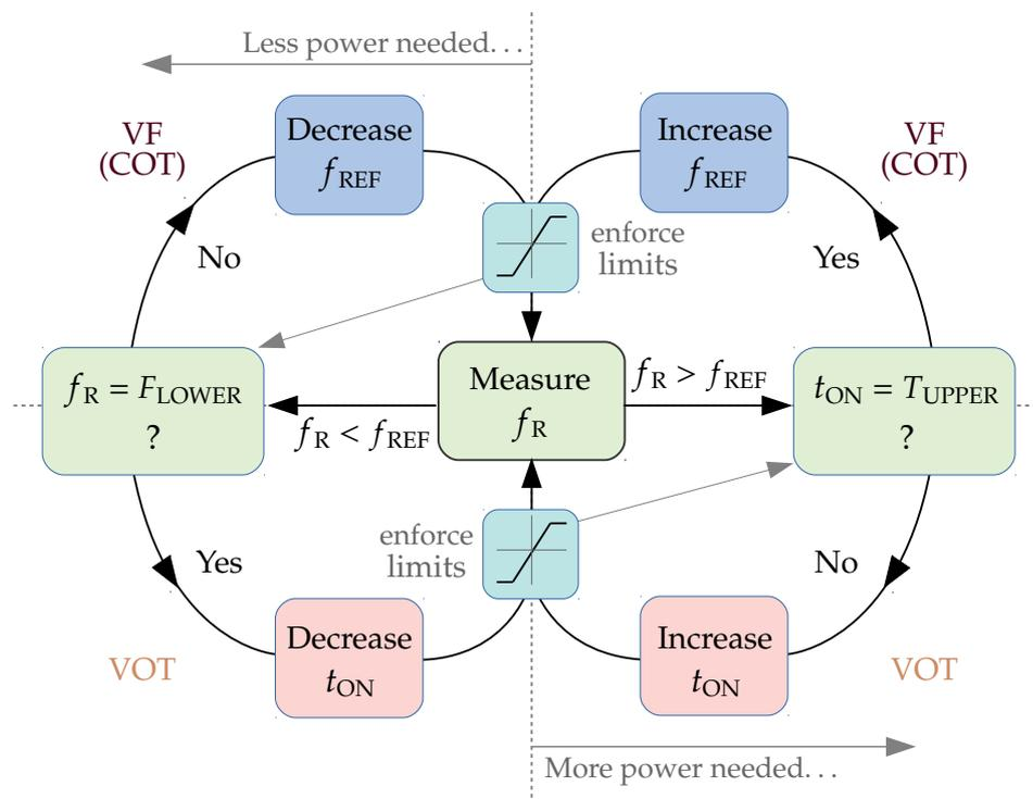
Figure 7.6: Flow chart of VF-VOT control scheme.
