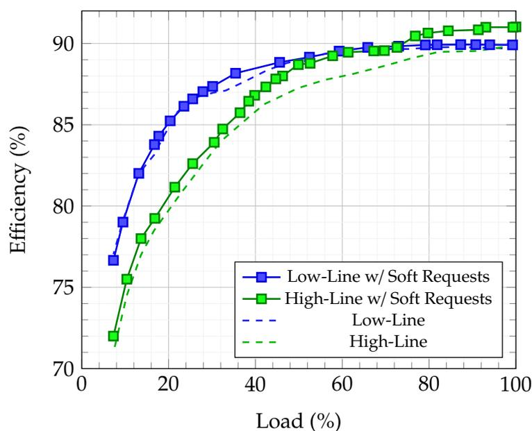
Figure 7.5: *SSCF2* VOT efficiency, with and without soft turn-ON requests.
