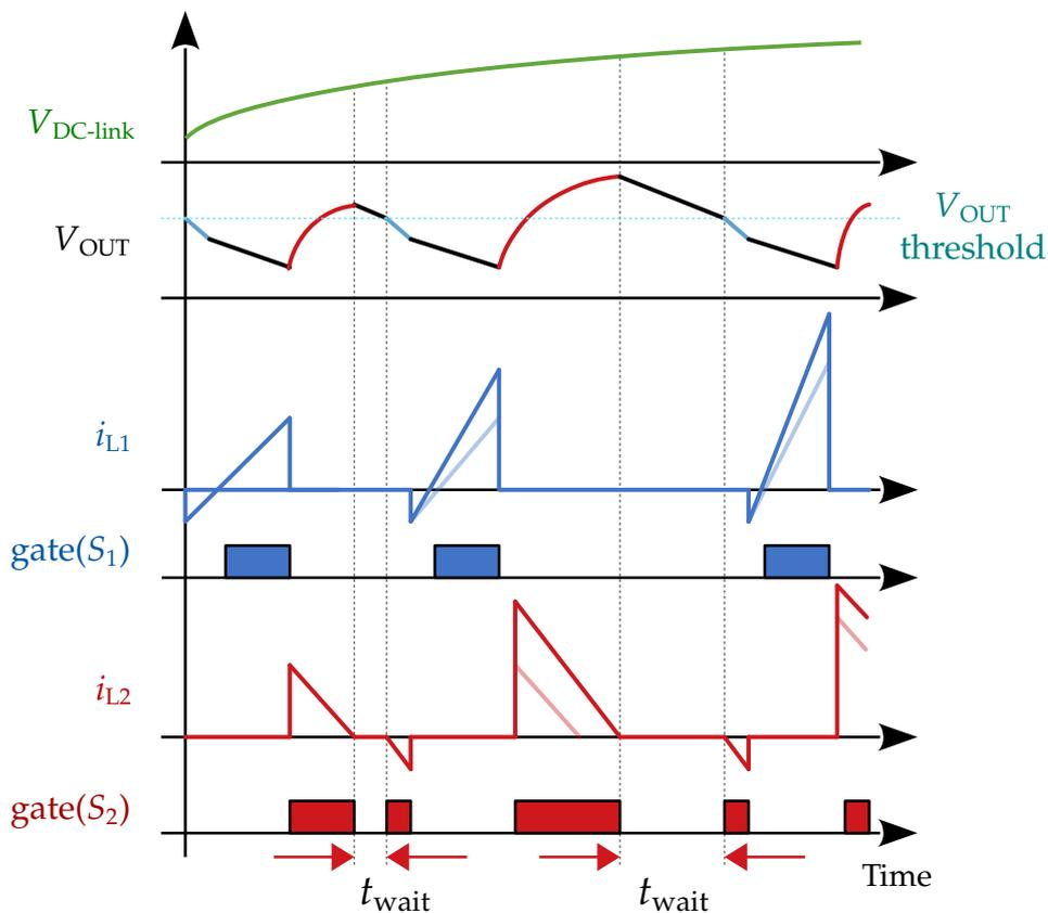
Figure 5.5: Sketch of COT control scheme with rising DC-link voltage.
