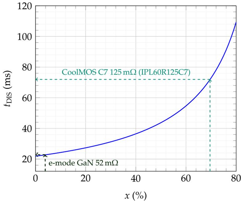
Figure 8.1: Estimated reverse power flow discharge time for versus ratio  $x$ .
