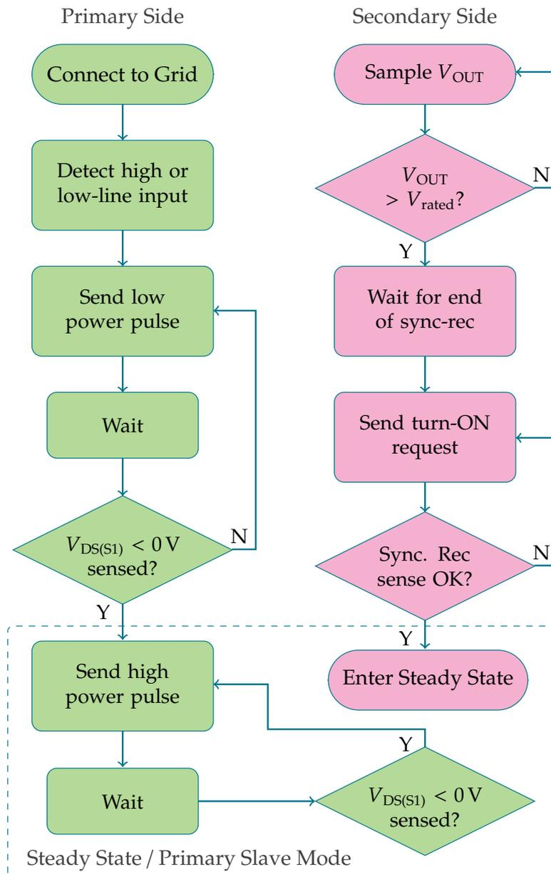
Figure 5.7: Flow chart of primary start-up routine with secondary side response.
