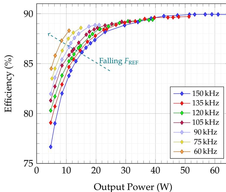
Figure 7.12: Measured low-line *SSCF2* VOT efficiency with various  $F_{REF}$ . Replicating the effect of reducing  $F_{LOWER}$  in VF-VOT control.
