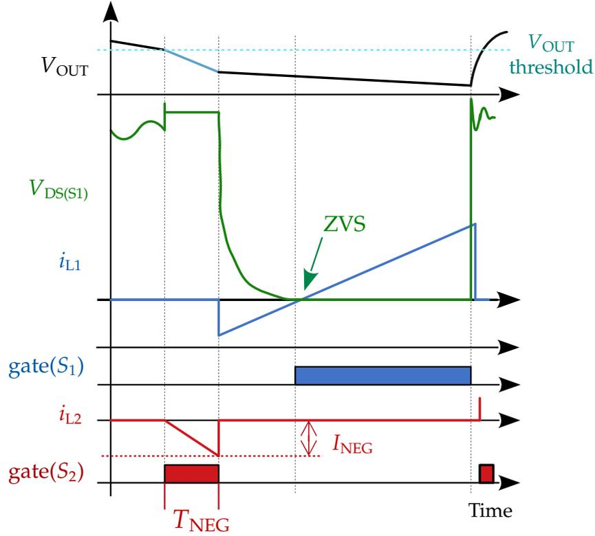
Figure 4.3: Sketched close up of proposed turn-ON request using negative current.
