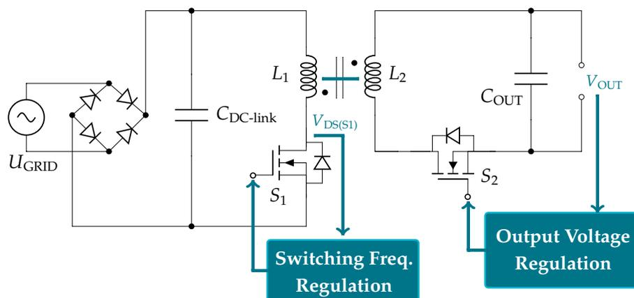
Figure 6.9: Schematic showing split regulation responsibilities resulting from VOT.
