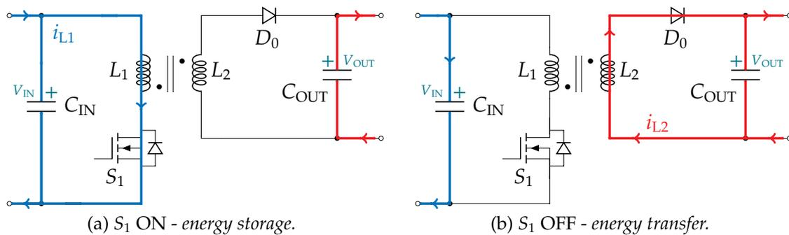
Figure 2.2: Sketch of Flyback current flow during  $S_1$  ON and OFF periods.
