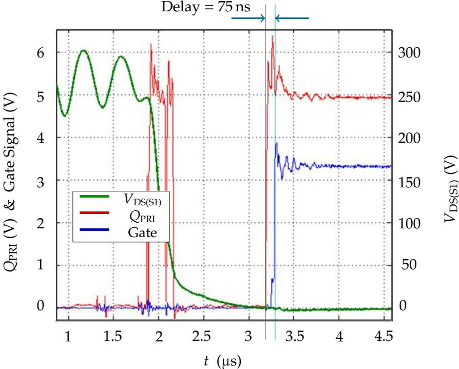
Figure 5.16: Demonstration of primary side  $V_{DS}$  sensing at low-line.
