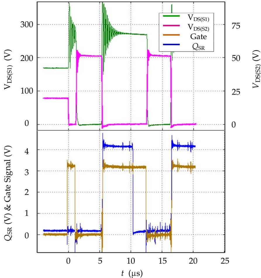
Figure 5.13:  $V_{DS}$ , sync. rec sense and  $S_2$  gate signals in overload conditions.
