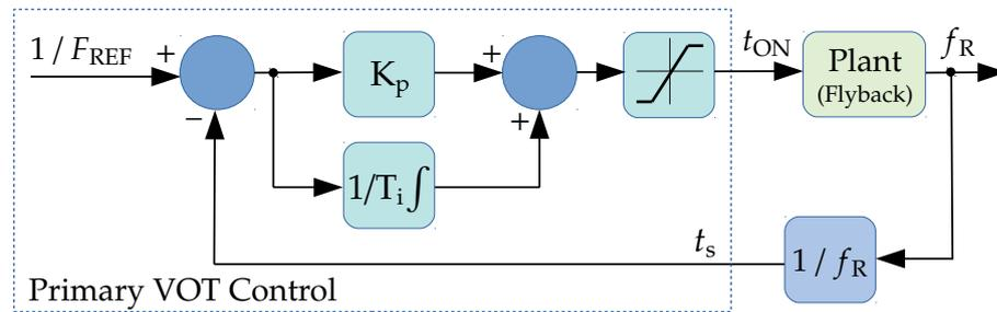
Figure 6.8: Simplified diagram of implemented primary side control loop.
