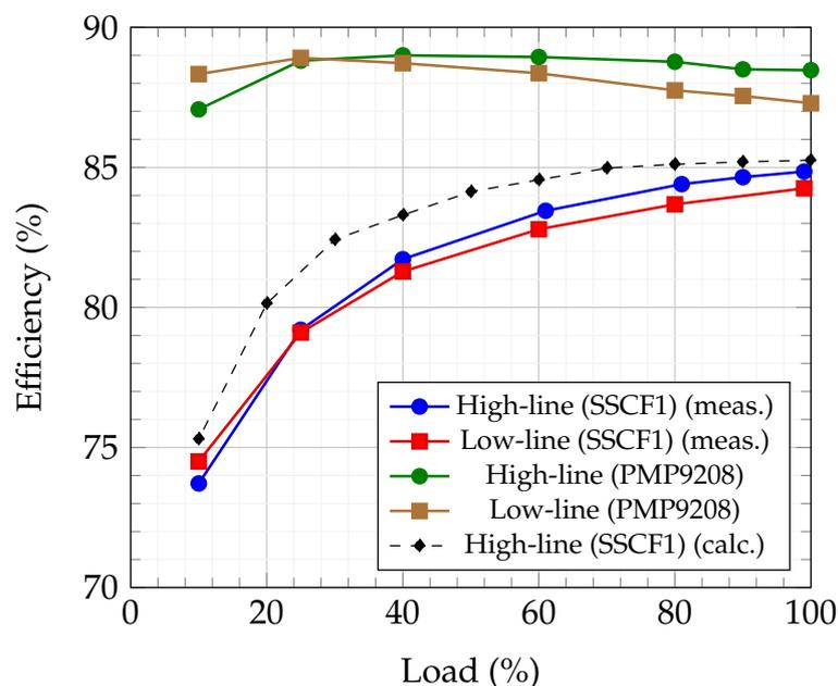
Figure 5.20: Measured and calculated *SSCF1* efficiency against PMP9208.
