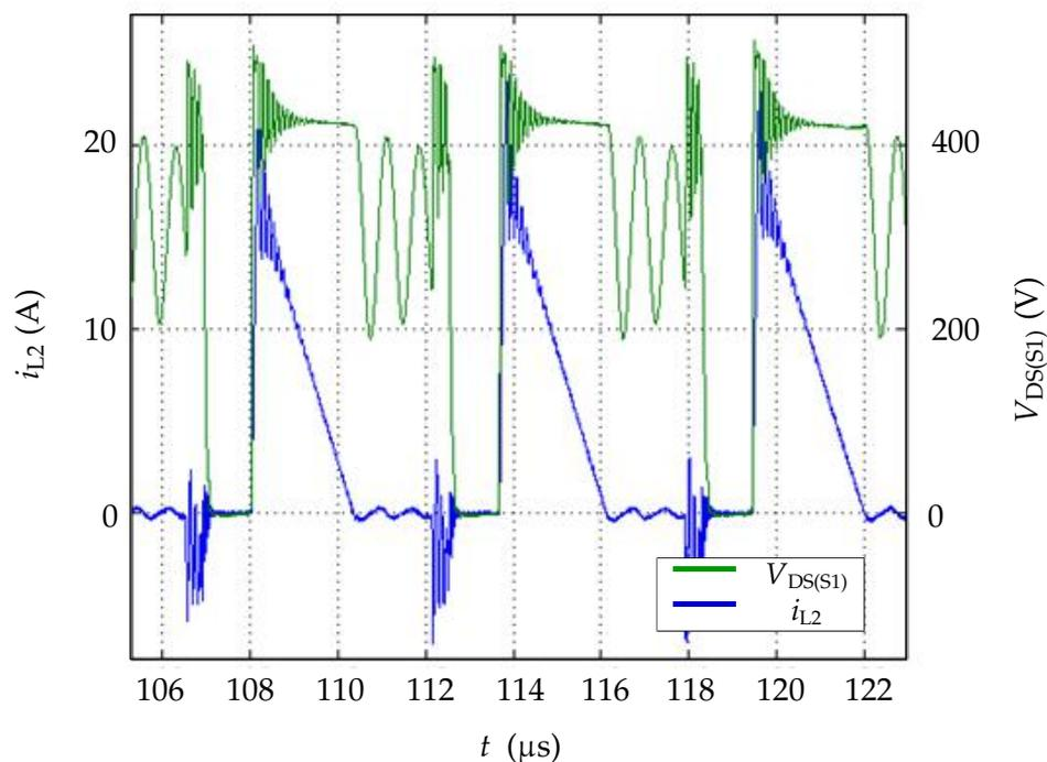
Figure 5.11: Measured  $V_{\text{DS}(s1)}$  and  $i_{L2}$  in high-line steady-state COT operation.
