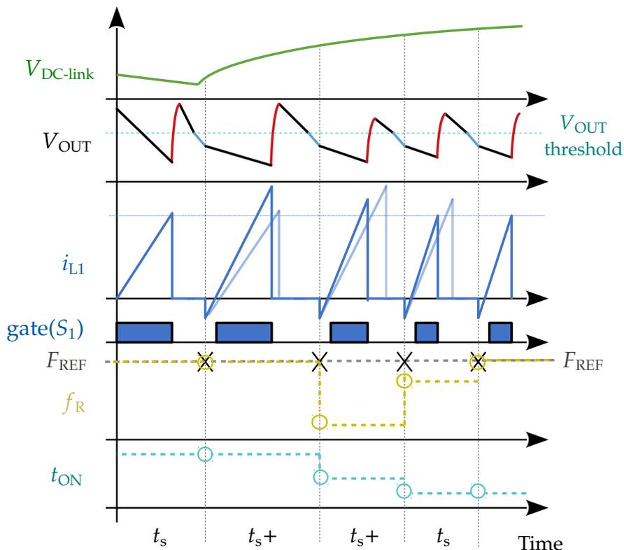
Figure 6.5: VOT control response to rising DC-link voltage.
