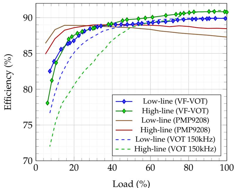
Figure 7.11: Comparison of SSCF2 VF-VOT vs. 65 W TI PMP9208 demonstrator.
