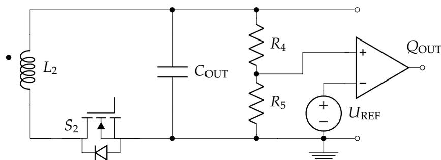
Figure 5.4: Schematic of output voltage sensing circuit in context with  $L_2$  and  $S_2$ .
