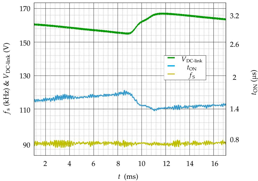
Figure 7.9: SSCF2 low-line VF-VOT at 25% load.
