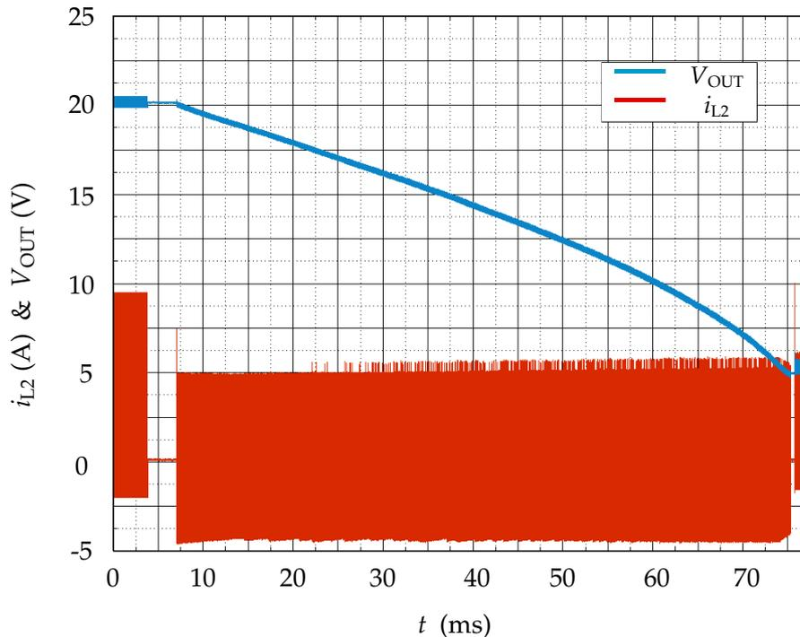
Figure 7.15: Measurement of reverse power flow; discharging 20 V to 5 V.
