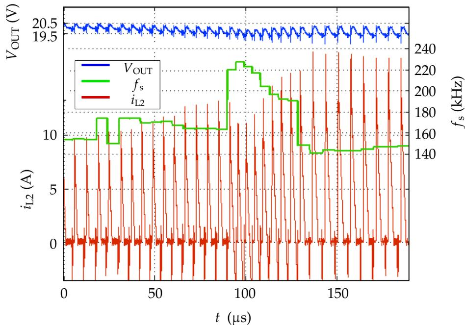
Figure 6.19: VOT reaction to jump from 30 % to 100 % load.
