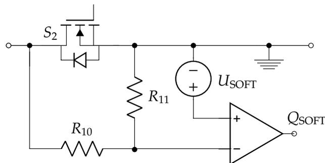
Figure 7.2: Schematic of sensing circuit for soft turn-ON requests.
