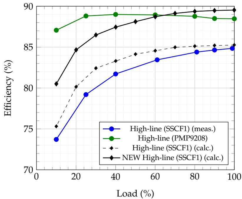
Figure 5.23: Comparison of simulated and measured efficiency of *SSCF1* using original and modified transformer versus PMP9208.
