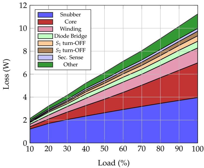
Figure 5.21: Overall loss breakdown for SSCF1 in high-line operation (calculated).
