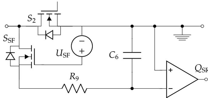
Figure 6.4: Schematic of sensing circuit for synchronous rectification.
