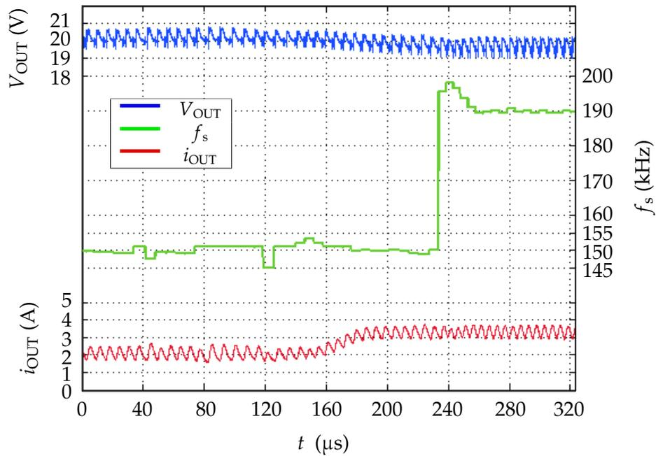
Figure 6.21: Measurement of natural output current limiting at 110 % load.
