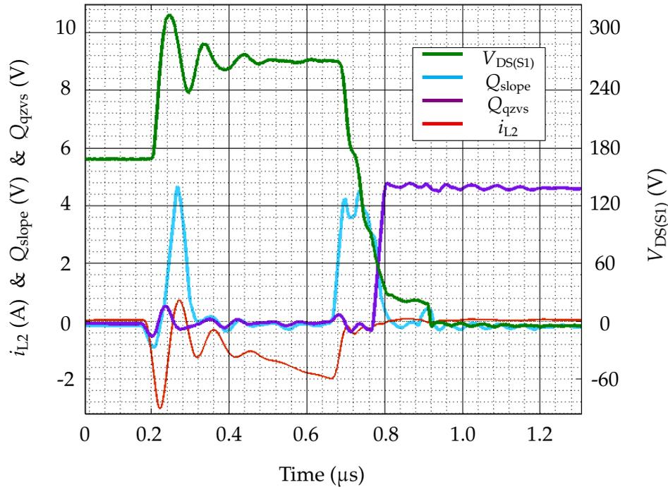
Figure 6.13: Zoomed view of turn-ON request with SSCF2  $V_{DS(S1)}$  sensing signals.
