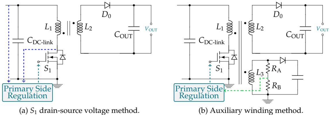
Figure 3.2: Diagram of two primary side regulation variations.
