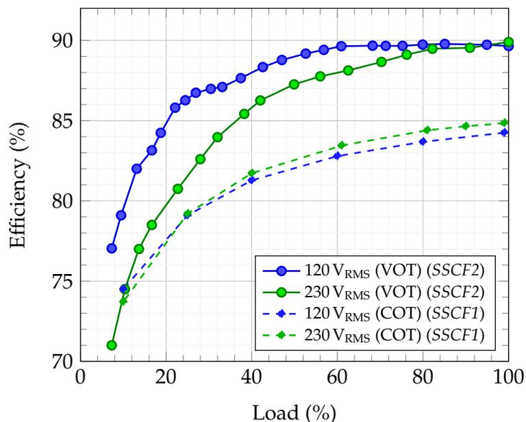
Figure 6.23: Measured efficiency of demonstrator using COT and VOT controls.
