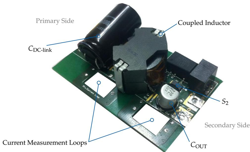
Figure 5.9: 65W demonstrator, *SSCF1*. Dimensions: 3.0 cm × 6.5 cm × 2.3 cm.
