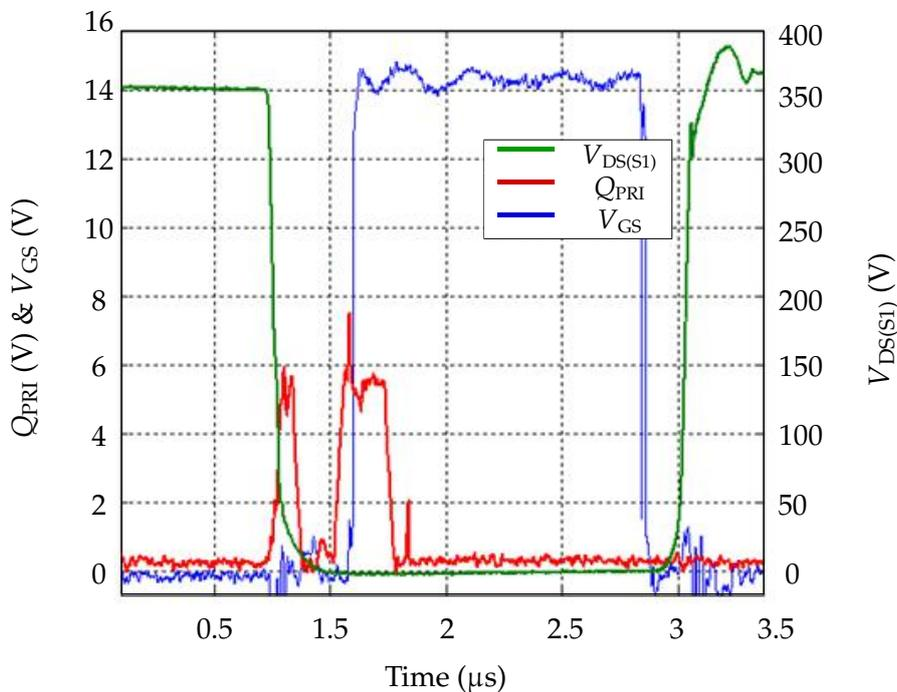
Figure 5.2: Measurement of primary  $V_{DS}$  sensing sub-circuit in operation.
