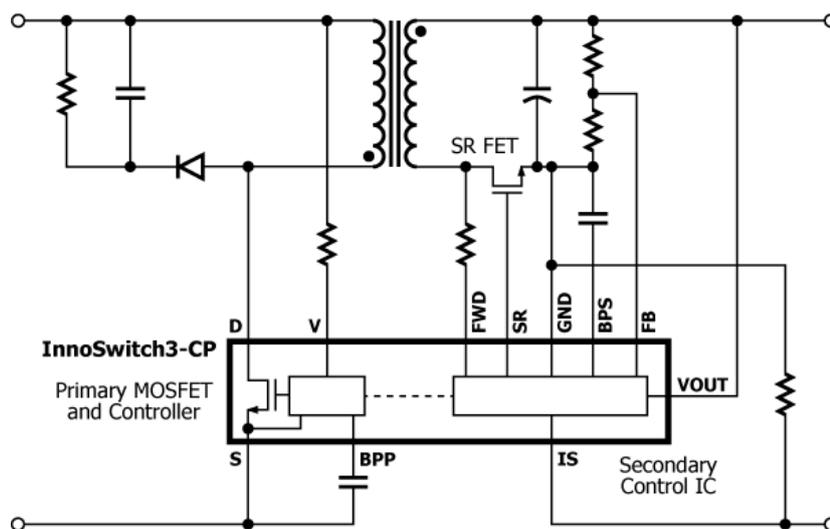
Figure 3.5: Schematic of the InnoSwitch3-CP controller [35].
