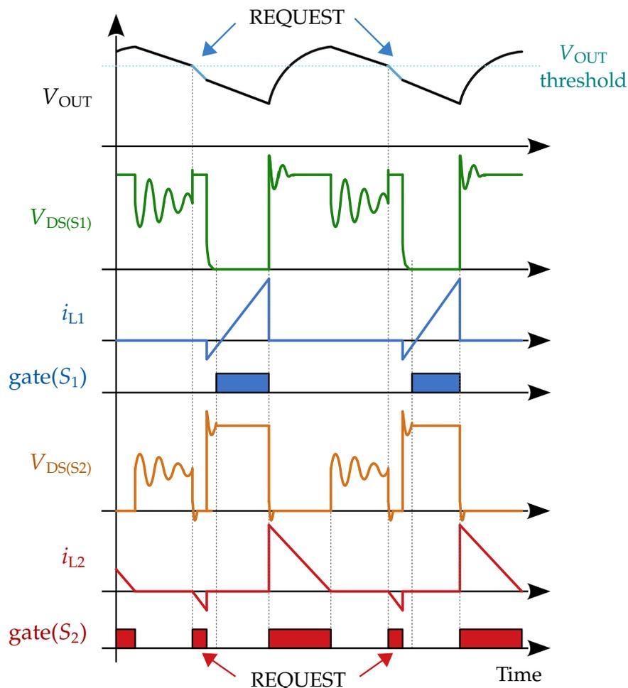
Figure 4.4: Secondary side controlled Flyback turn-ON requests with gate signals,  $V_{\text{OUT}}$ , inductor currents and drain-source voltages.
