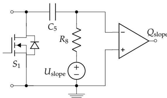
Figure 6.3: Schematic of primary  $V_{DS}$  slope sensing circuit.
