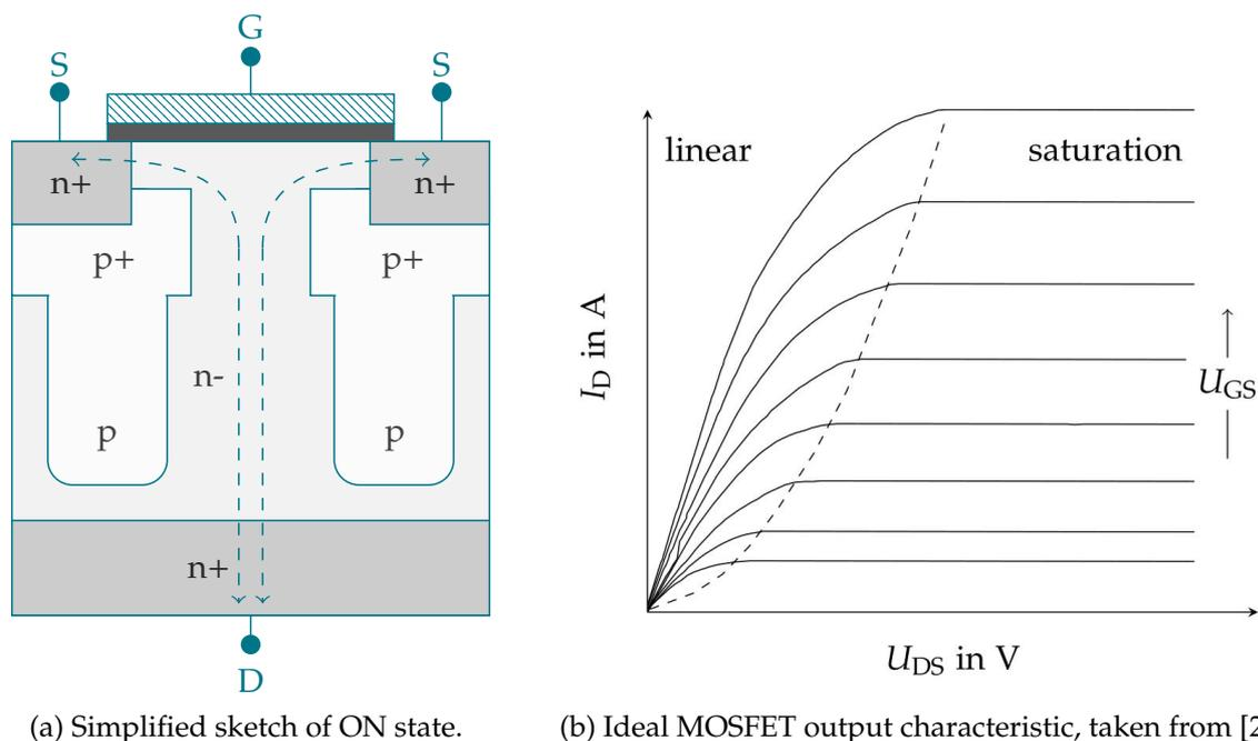
Figure 2.8: Super-junction MOSFET structure during ON state (a) and ideal MOSFET output characteristic (b).
