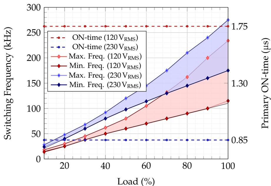
Figure 5.14: SSCF1 Switching frequency and primary ON-time vs. output load.
