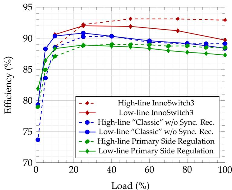
Figure 3.6: Efficiency comparison of various 65 W Flyback demonstrators examples.
