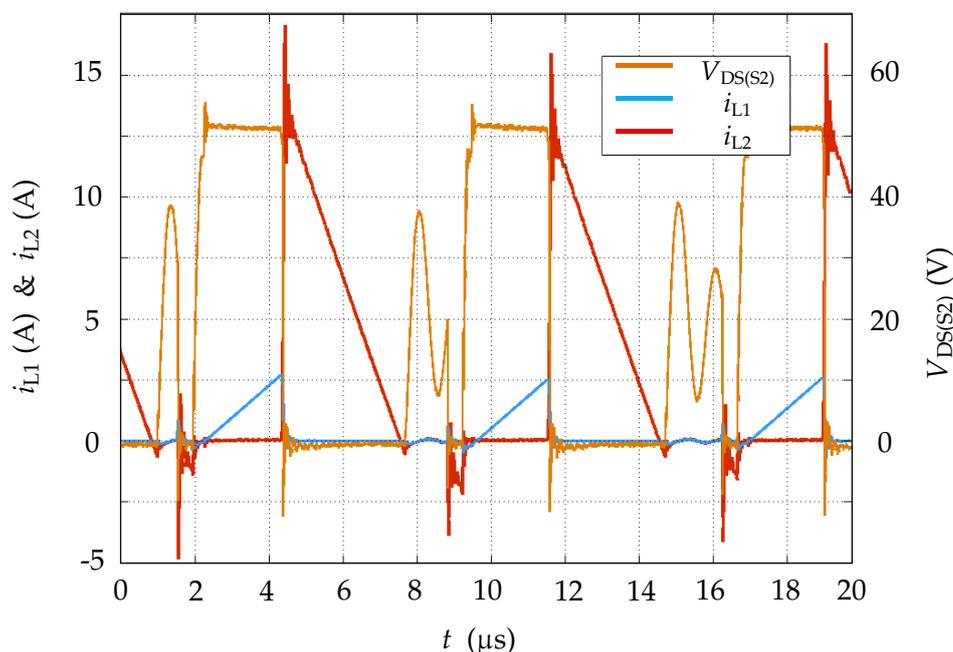
Figure 7.1: Measured effects of irregular  $S_2$  turn-ON voltage.
