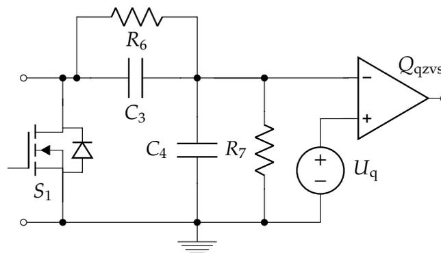
Figure 6.2: Schematic of circuit for detecting quasi-ZVS threshold crossings.
