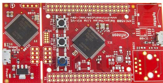
Figure 5.8: INFINEON XMC4500 Relax Lite prototyping controller board.
