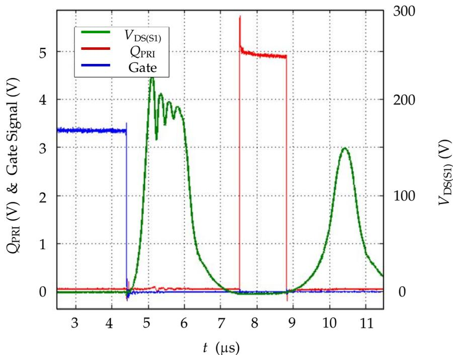
Figure 5.17: Demonstration of blanked zero voltage crossings in Flyback ringing.
