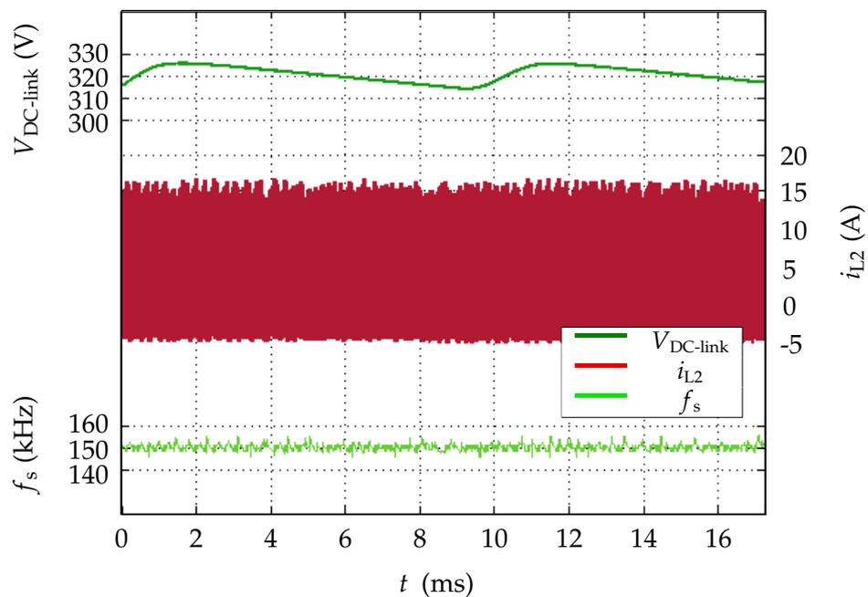
Figure 6.17: SSSF2 steady-state VOT operation. Input:  $230\text{ V}_{\text{RMS}}$ . Output:  $20\text{ V}$ ,  $36\text{ W}$ .
