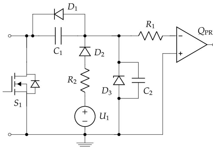
Figure 5.1: Schematic of circuit for detecting zero voltage crossings.
