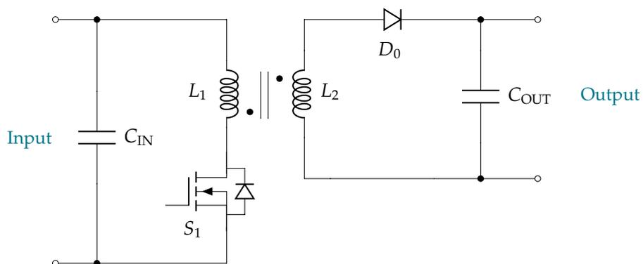
Figure 2.1: Fundamental principle schematic of the Flyback converter.
