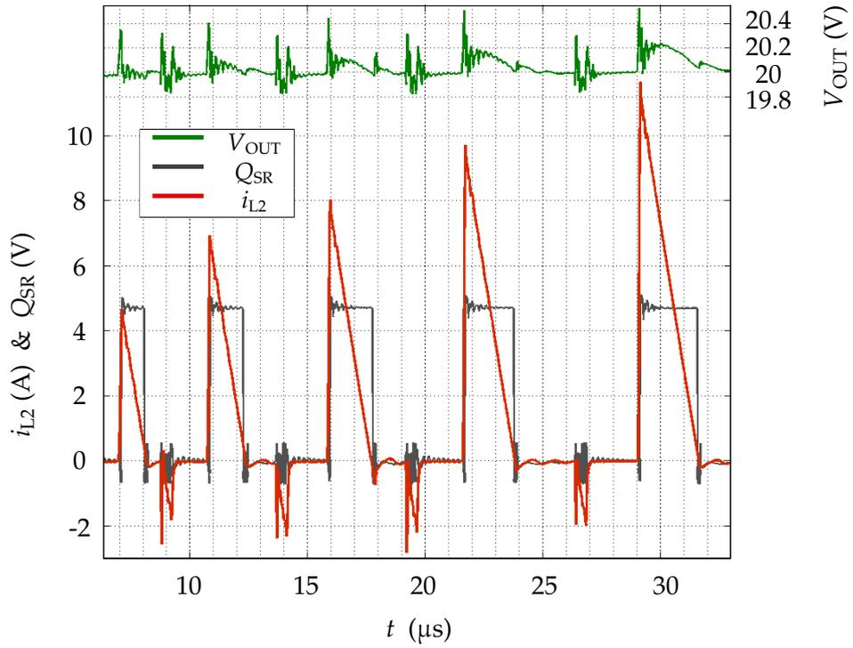
Figure 6.14: SSCF2 synchronous rectification sense response for various currents.
