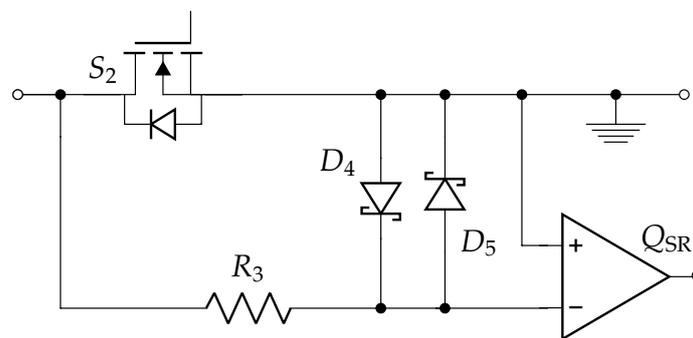
Figure 5.3: Schematic of sensing circuit for synchronous rectification.
