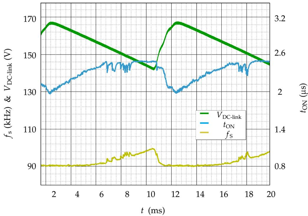
Figure 7.8: SSCF2 low-line VF-VOT at 60% load.
