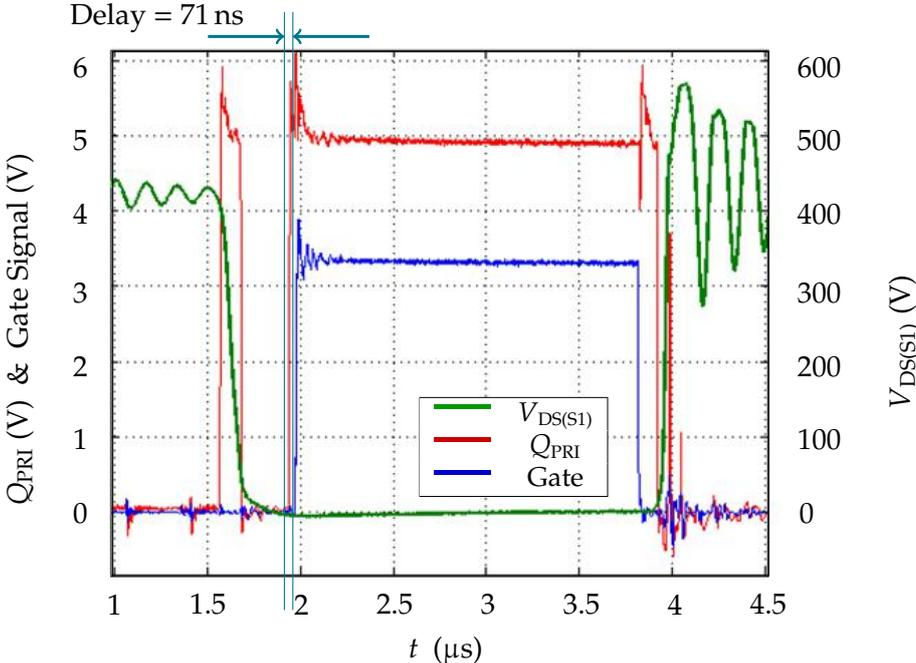
Figure 5.15: Demonstration of primary side  $V_{DS}$  sensing at high-line.
