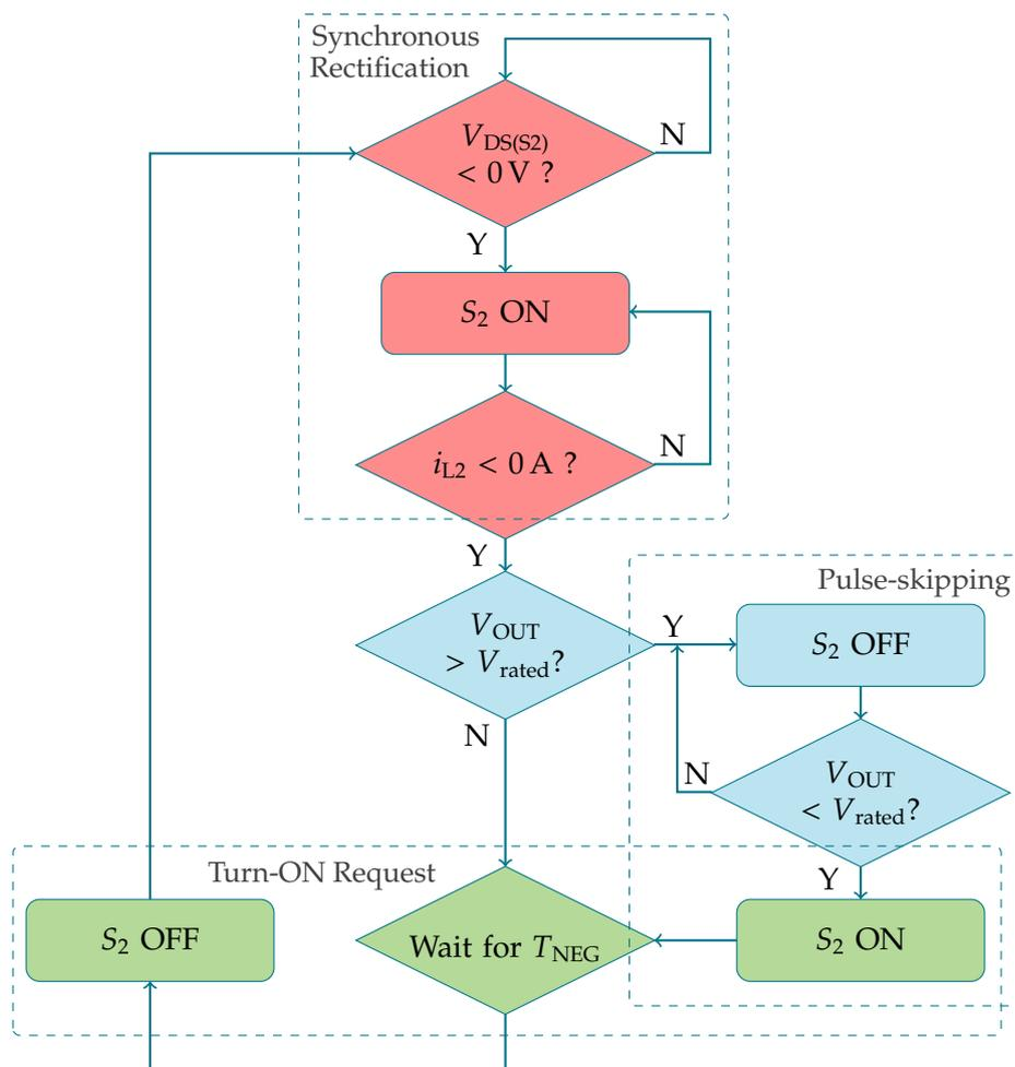
Figure 5.6: Flow chart of steady-state from perspective of secondary side controller.
