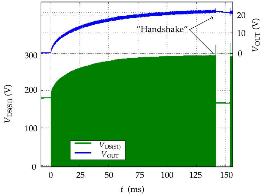
Figure 5.18: Measurement of proposed start-up routine with low-line input voltage.
