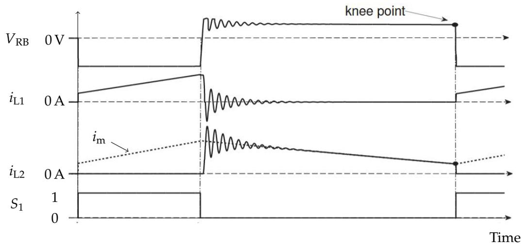
Figure 3.3: Knee-point and typical Flyback waveforms for CCM mode [9].
