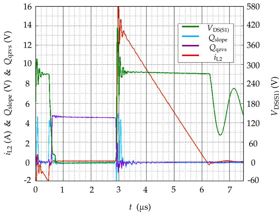
Figure 6.12: Measured response of primary SSCF2  $V_{DS(S1)}$  sensing circuits.
