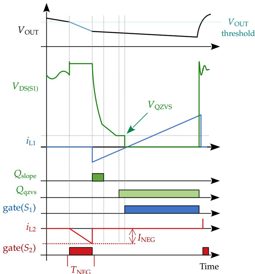
Figure 6.1: Sketch of Q-ZVS turn-ON request, with sense and gate signals.
