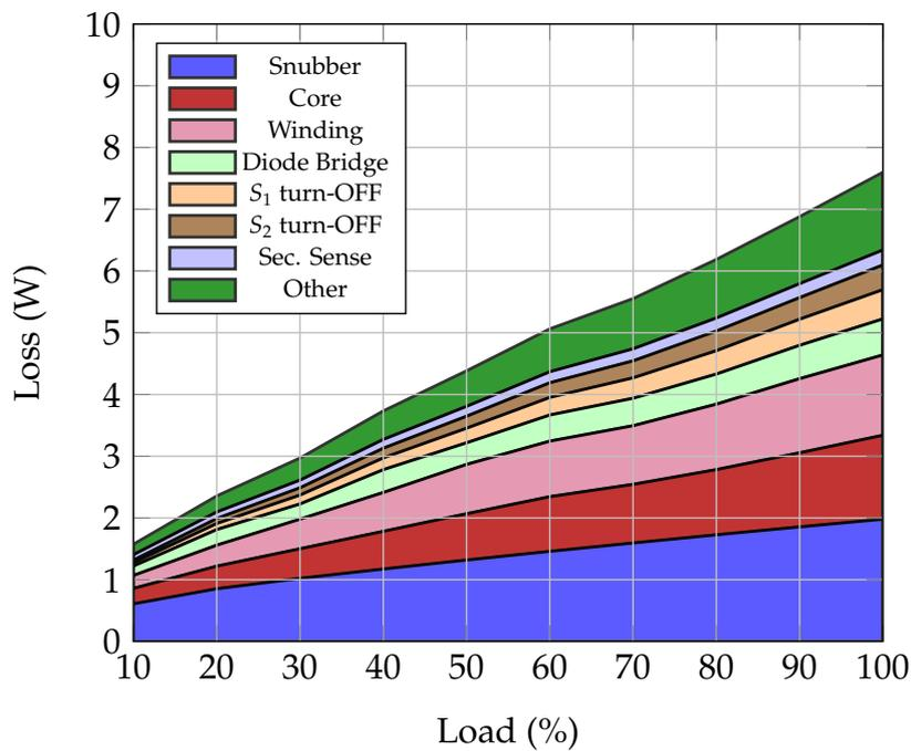
Figure 5.24: Loss breakdown assuming coupled inductor core material 3C96.
