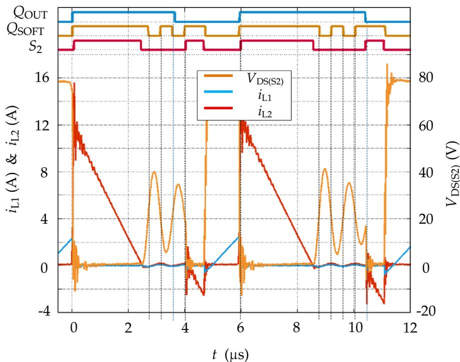
Figure 7.3: Measured application SSCF2 using soft  $S_2$  turn-ON requests.
