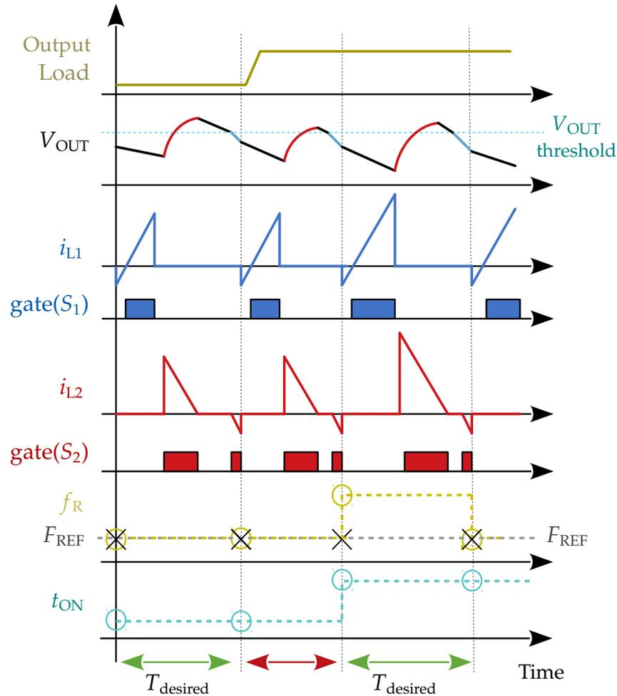
Figure 6.6: Effect of increasing output load on  $t_{\text{wait}}$  and VOT response.
