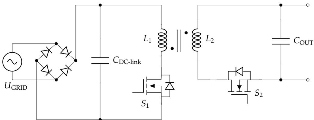
Figure 2.4: Schematic of grid-connected Flyback converter with active synchronous rectification switch  $S_2$ .
