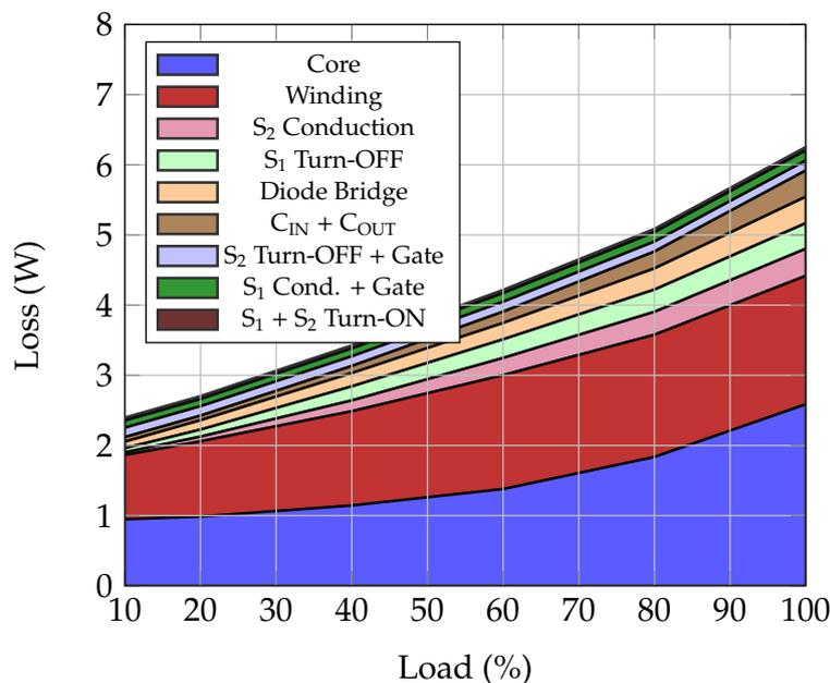
Figure 6.24: Overall loss breakdown for SSCF2 with 230 V<sub>RMS</sub> input and VOT operation (calculated).
