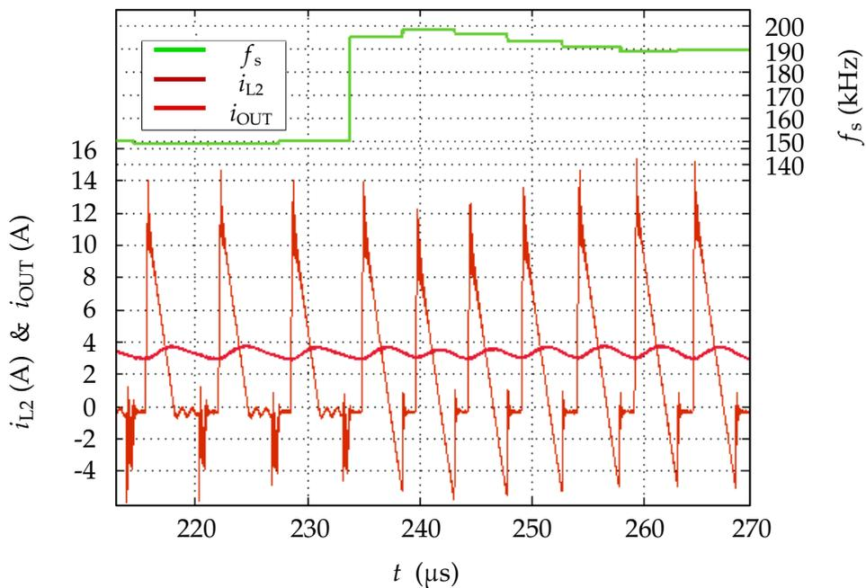
Figure 6.22: Zoomed measurement of natural output current limiting at 110 % load.
