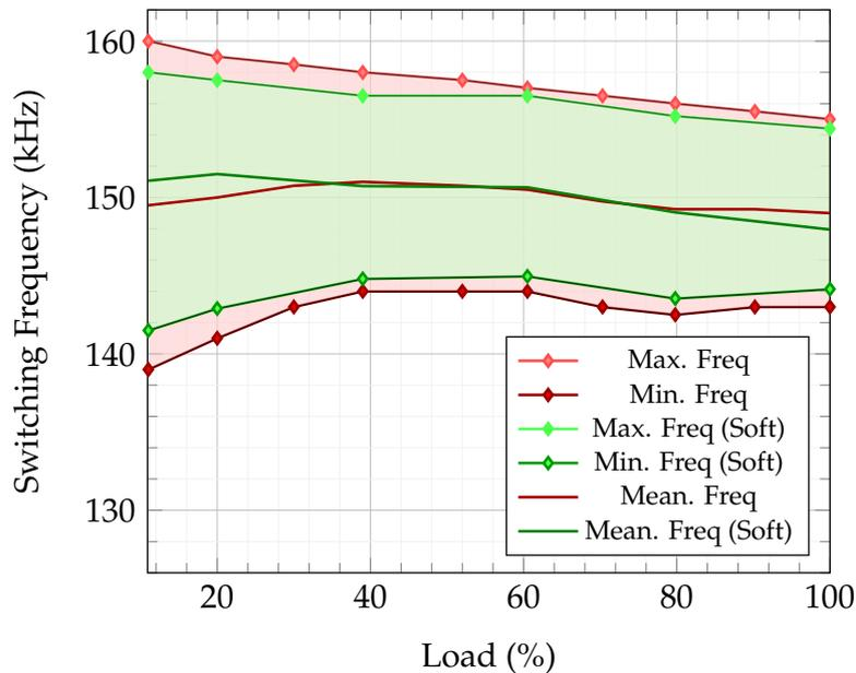
Figure 7.4: *SSCF2* switching frequency vs. load for low-line input with and without soft turn-ON requests.
