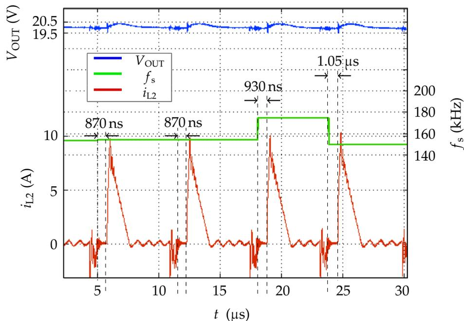
Figure 6.18: Reaction of VOT in case of frequency deviation.
