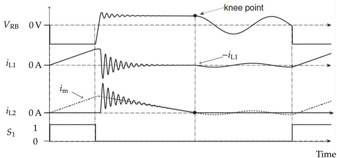
Figure 3.4: Knee-point and typical Flyback waveforms for DCM mode [9].
