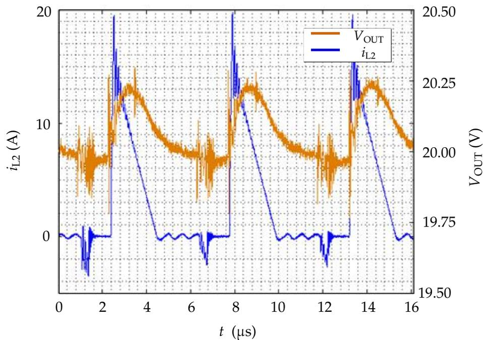
Figure 5.12: Measured  $V_{\text{OUT}}$  and  $i_{L2}$  in high-line COT steady-state operation.
