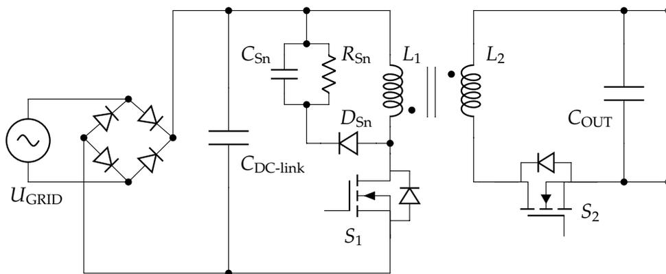
Figure 2.5: Principle schematic of a Flyback converter with  $S_1$  RCD snubber.
