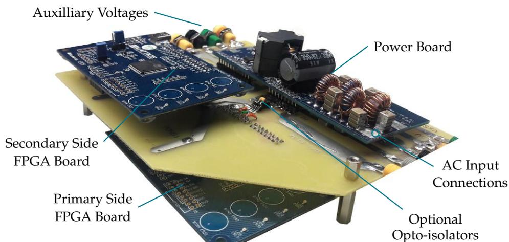
Figure 6.11: Adapter board connecting control boards to SSCF2 power board.
