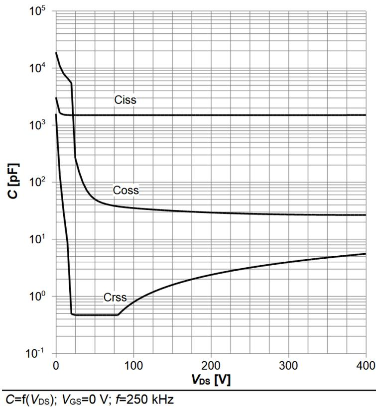
Figure 2.9: Parasitic capacitances of a 600 V CoolMOS C7 (IPL60R125C7) [24].
