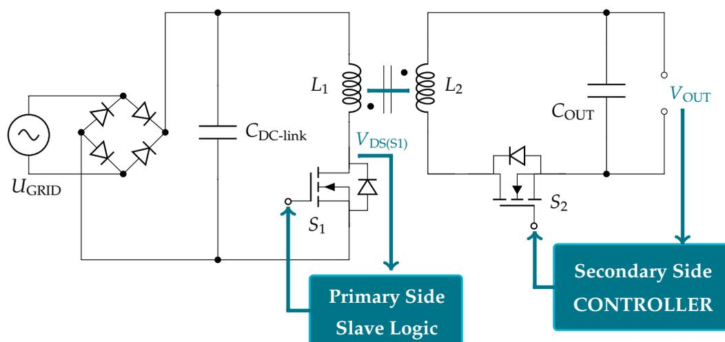
Figure 4.2: Proposed secondary side controller with independent primary side logic.
