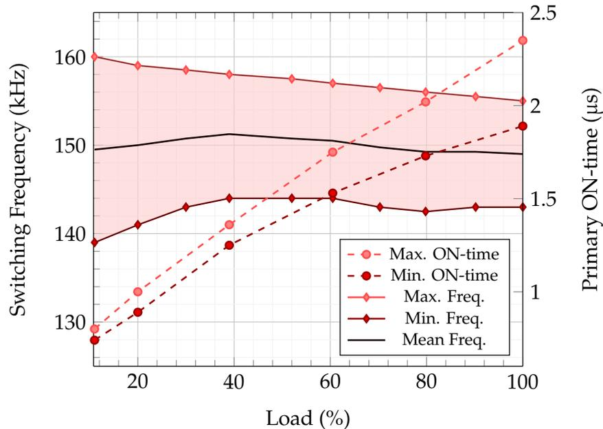
Figure 6.25: Minimum and maximum observed instantaneous  $f_s$  and  $t_{ON}$  for SSCF2 with 120 V<sub>RMS</sub> input voltage.
