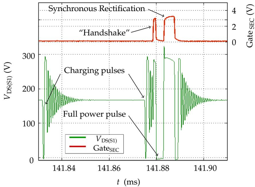
Figure 5.19: Annotated close-up of end of proposed start-up routine.
