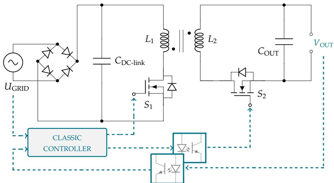
Figure 3.1: Flyback converter with block diagram of conventional control structure.
