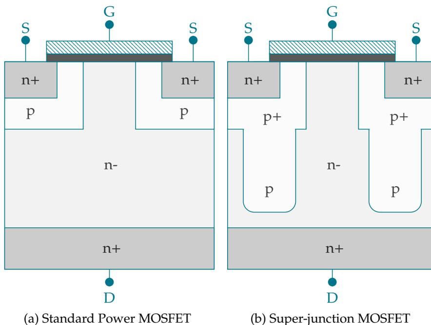
Figure 2.6: Simplified sketch of vertical N-channel power MOSFETs.
