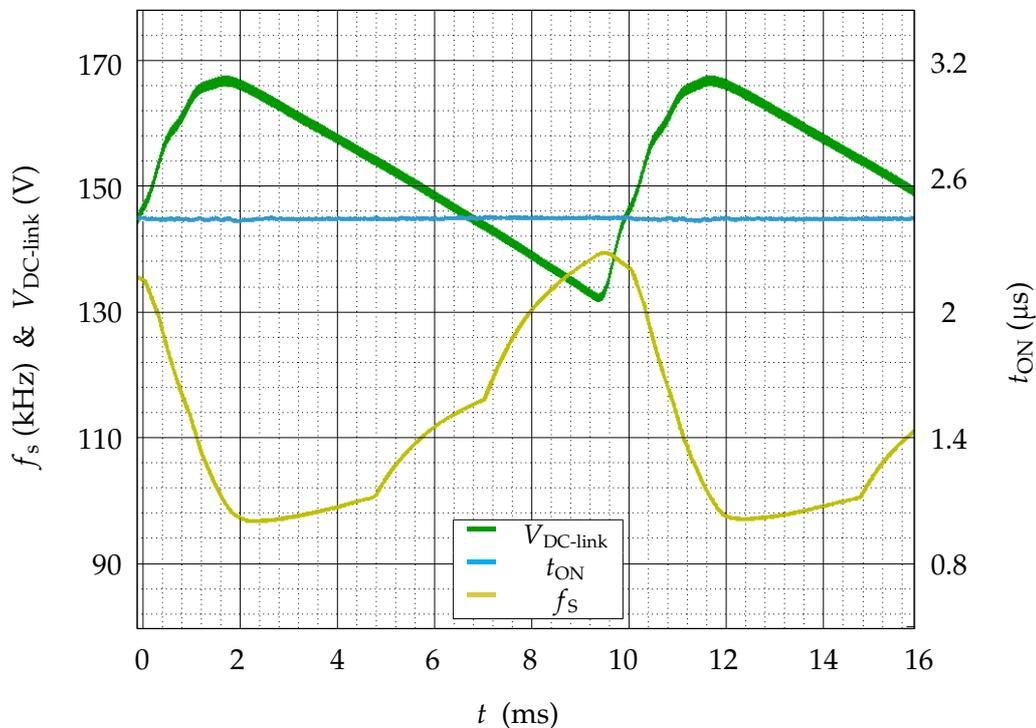
Figure 7.7: SSCF2 low-line VF-VOT at 90 % load.
