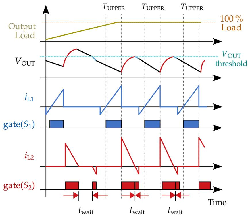
Figure 6.7: Operational effect on  $t_{\text{wait}}$  for full output load, defined by  $T_{\text{UPPER}}$ .
