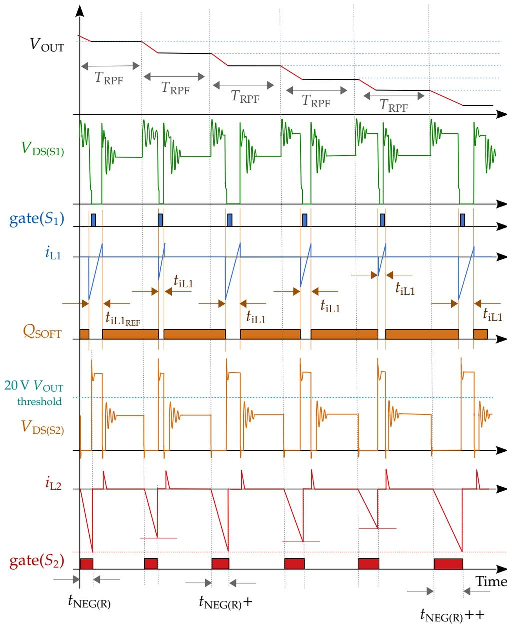
Figure 7.13: Sketch of reverse power flow concept.
