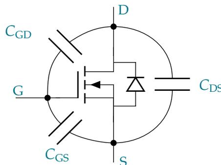
Figure 2.7: MOSFET circuit model.
