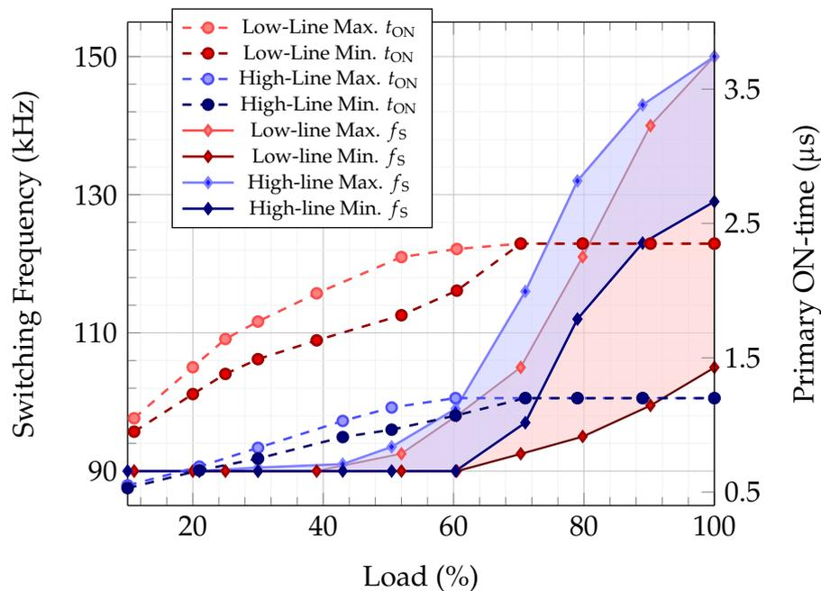
Figure 7.10: SSCF2 VF-VOT Switching frequency and primary ON-time vs load.
