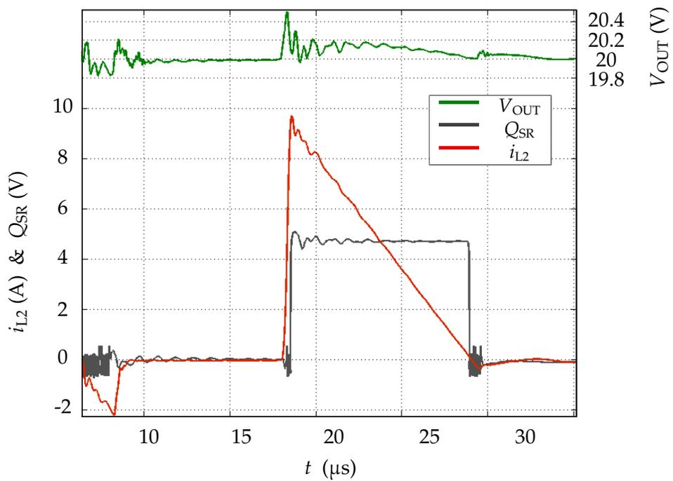
Figure 6.15: Zoom of measured SSCF2 synchronous rectification sense response.
