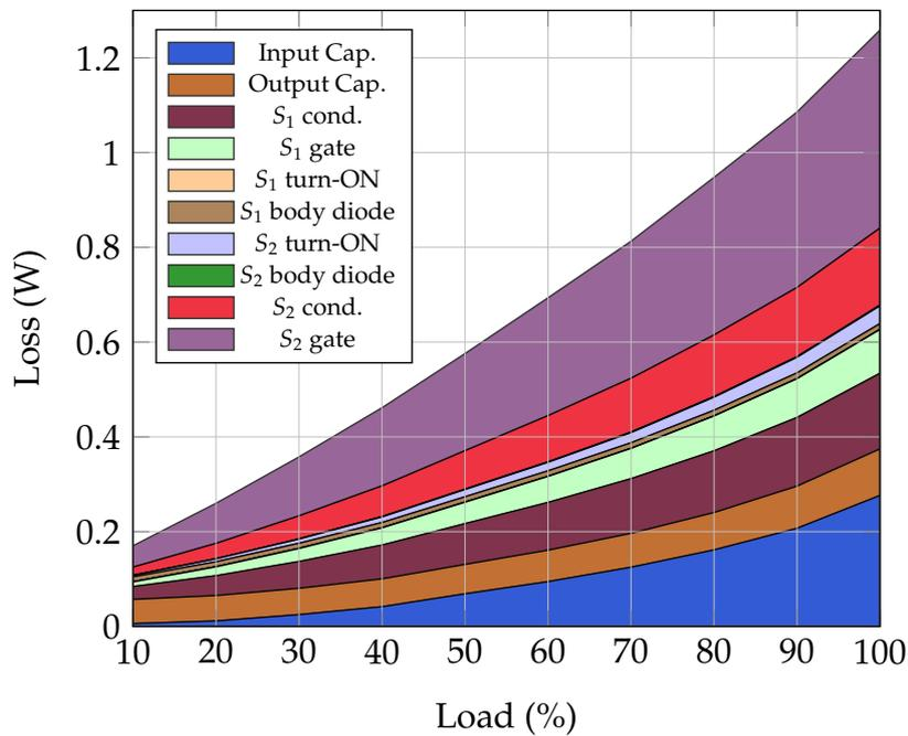
Figure 5.22: Breakdown of loss contributions labelled as "Other" in Fig. 5.21.
