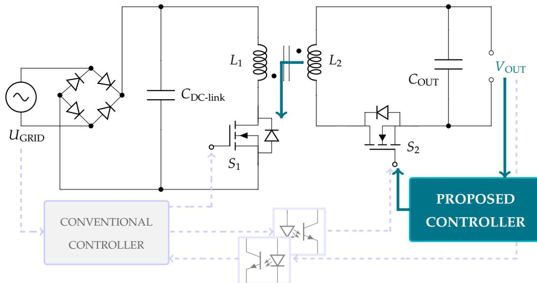
Figure 4.1: Comparison of conventional and proposed Flyback controllers.
