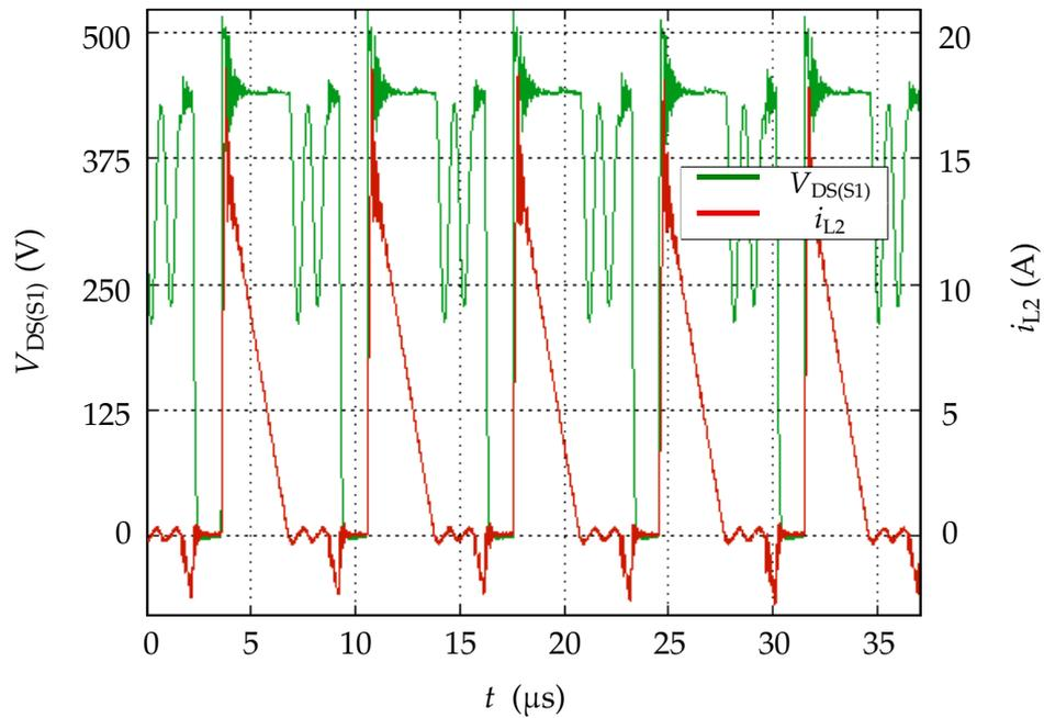
Figure 6.16: Zoom of SSSF2 steady state VOT operation.
