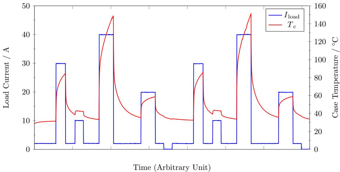
Figure 4.9: This diagram shows two load cycles applied onto an LV MTS which is configured according to Table 4.2. The load current  $I_{load}$  (blue) is set for the appropriate time span and the temperature increase of the DUT’s case is measured simultaneously (red).
