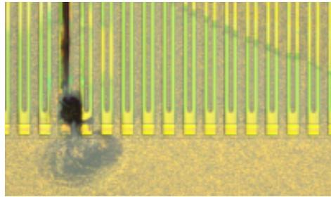
Figure 4.13: Optical micrograph of GaN device failed in short circuit, showing only local damage due to fast protective shut down [23].
