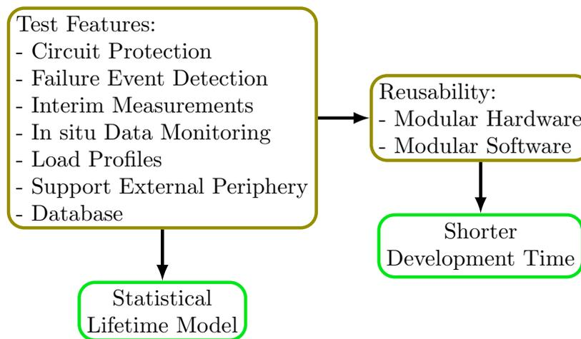
Figure 1.2: Essential features for life test systems are listed which are necessary to gather statistical analyses out of test runs. Re-usage of available test hardware and software is reasonable to provide flexibility, adaptability and future-proofness to various test applications and device requirements and to shorten the development time.
