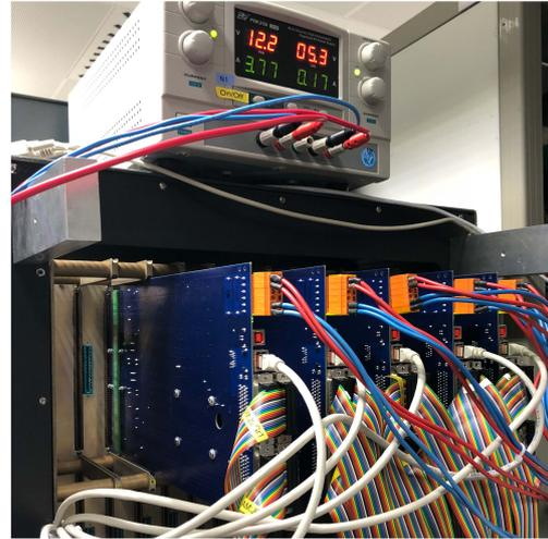
(a) Stress boards within the environmental chamber. (b) At the backside of (a): FPGA-based control modules with cabling.
