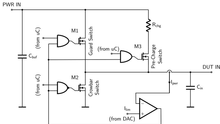
Figure 4.3: Detailed schematic of the three-transistor-solution for the guard block at the LV application module. The two transistors M1, M2 shut down and discharge  $C_{\text{buf}}$  in case of failure. M3 is used for start-up to avoid inrush current peaks which may accidentally trigger the overcurrent shut down.
