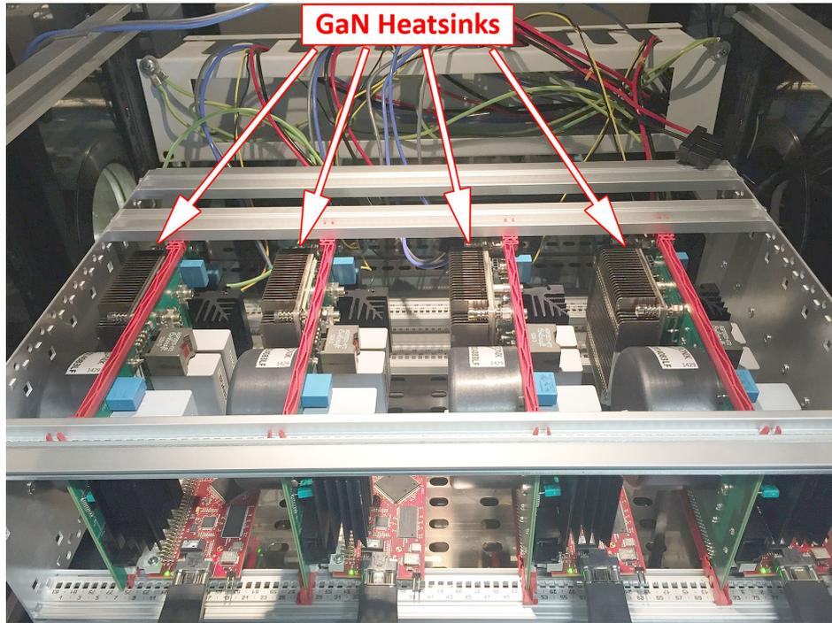
Figure A.3: Four **MV MTS** application boards are mounted in a 19" rack case which is placed within an environmental chamber. In the center of the figure, the heat sinks can be seen which cover the **GaN** transistors. At the bottom and in red **PCB** color the connected control modules are situated. The black inductors for the boost conversion in the center-bottom area are also distinctly visible [23].
