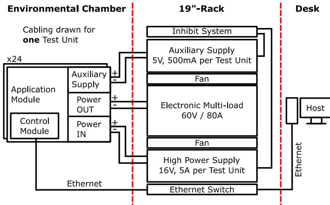
Figure 4.6: In this block diagram, all additionally necessary devices to build up an LV MTS are depicted. In the left area, the LV application modules are shown within the environmental chamber along with their connections to the outside. In the center, the peripheral devices which are the power supplies, the electronic multi-load, the inhibit system, and an Ethernet switch are mounted within a standard 19" rack. The central controlling host computer is symbolized to the right.
