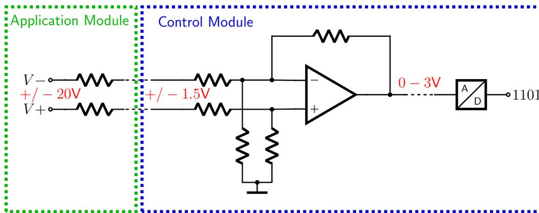
Figure 3.4: The stacked concept of the analog measurements performed by the MTS is depicted. On the control module, the input voltage range of the measurement channels is set to  $\pm 1.5V$  and by choosing an appropriate series resistor down on the application board, the voltage range can be extended.
