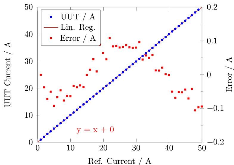
(b) Linear Regression of the  $I_{\text{out}}$  measurement after adjustment.
