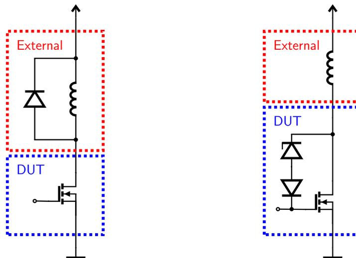
(a) Power MOSFET switch with separate free-wheeling path. (b) Power MOSFET switch with integrated clamped gate circuit.
