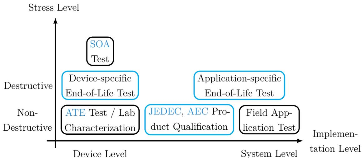
Figure 2.1: General overview of various types of tests which must be performed in the semiconductor industry. Blue boxes indicate tests which are run by automated life test systems and are in focus of this work.
