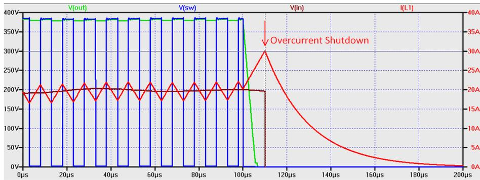
Figure 4.12: Spice simulation of protective system shut down in case of active (low-side) GaN failure by short circuit [23].
