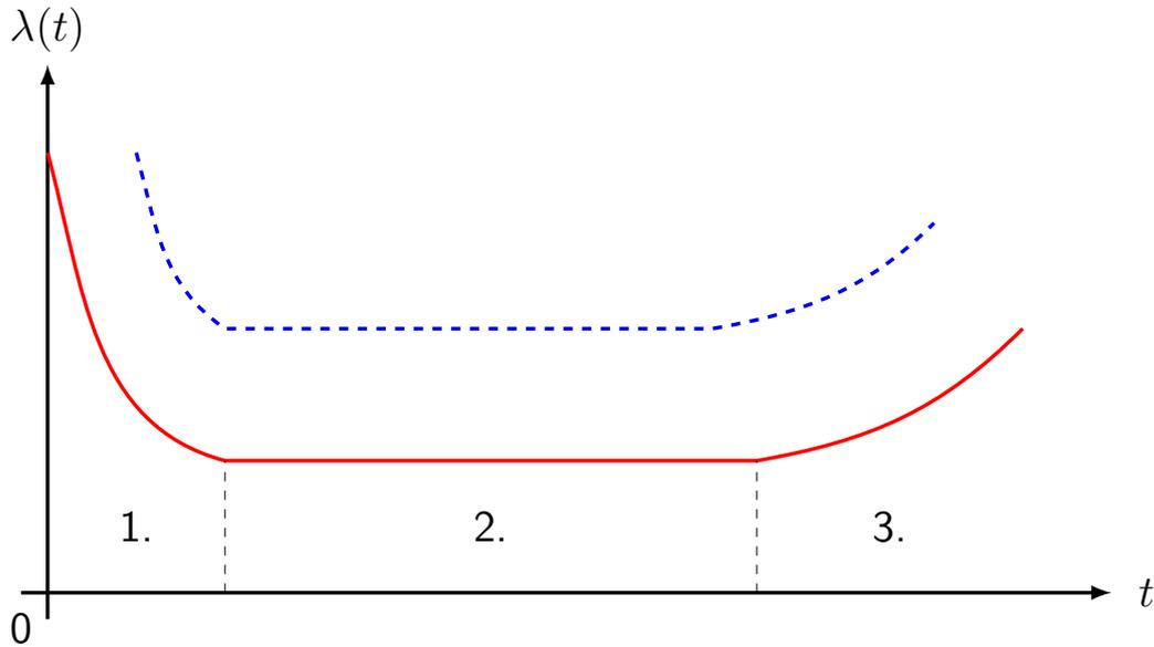
Figure 1.1: In this figure, the typical shape is depicted (commonly denoted as “*bathtub curve*”) for the failure rate of a large population of statistically identical *items*. The blue dashed curve shows a possible shift for a higher stress (e.g., increased ambient temperature) [1, p.7].
