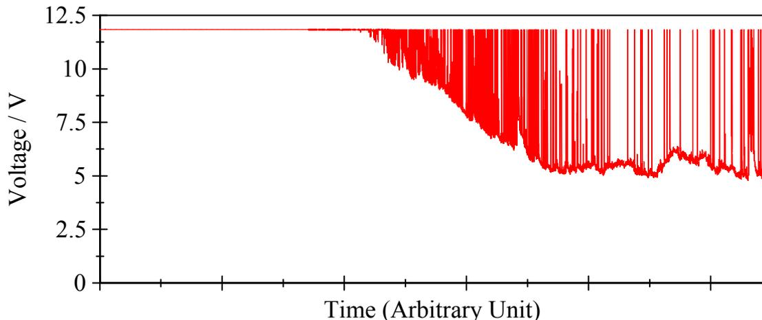
Figure 4.10: The input voltage  $V_{in}$  was continuously recorded during a power cycle test executed by the LV MTS. An interconnect problem occurred at the solder joint of the sense pin. The measurement at this defective contact had been toggling between the input voltage of 12 V and lower values.
