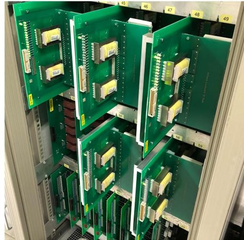
(c) Host computer and main power supplies. (d) The load boards are mounted within a separate rack which is located beside (a) and below (c).
