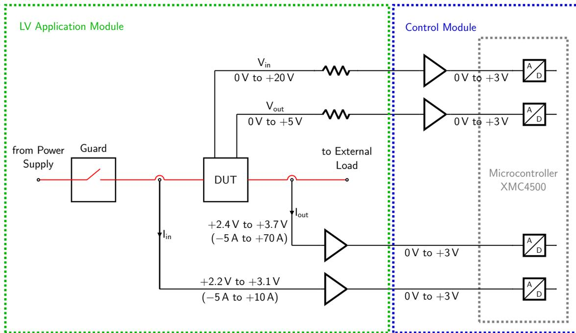
Figure 4.4: Detailed schematic of the current and voltage measurements implementation at the LV application module. All input measurement paths are attenuated to the ADC input range of 0 V to +3 V. The main power path through the LV application module is drawn in red.
