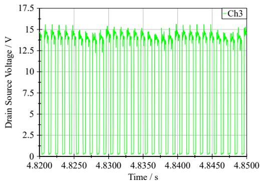
(c)  $V_{DS}$  measurement of load channel 3 from one DUT.
