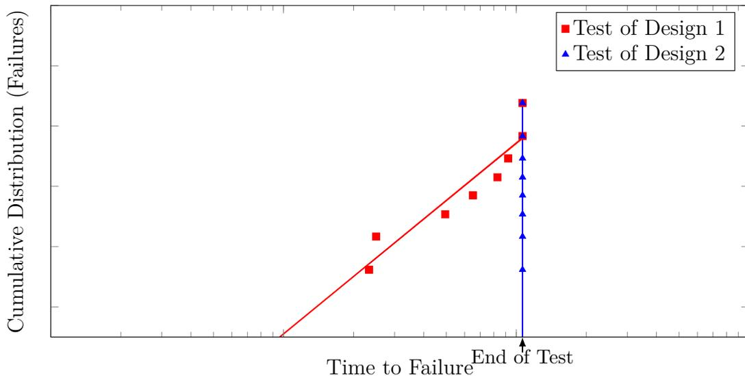
Figure 4.8: Lifetime results of two life tests conducted with the LV MTS.<sup>2</sup> On the x-axis, the run time of the test and on the y-axis the failure distribution are plotted. First, test 1 (red) was executed and device failures occurred. After improving the design of the DUT, the test was repeated (blue) and all DUTs survived the test until test termination.
