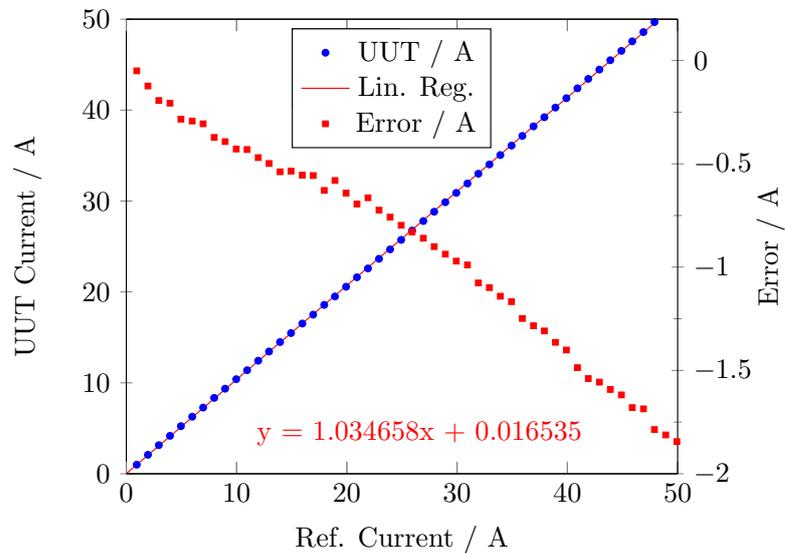
(a) Linear Regression of the  $I_{\text{out}}$  measurement before adjustment.
