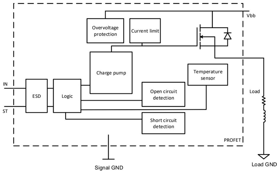
Figure 2.3: The block diagram [52] shows the circuit parts of an Infineon PROFET™ device. The main function of the IC is the high-side power transistor which switches various (resistive and/or inductive) loads in automotive applications. Additionally, it is equipped with protective functions like overvoltage protection, current limiting and temperature sensing. In case of a fault condition within the application, it will shut down the power transistor and provide a status feedback.
