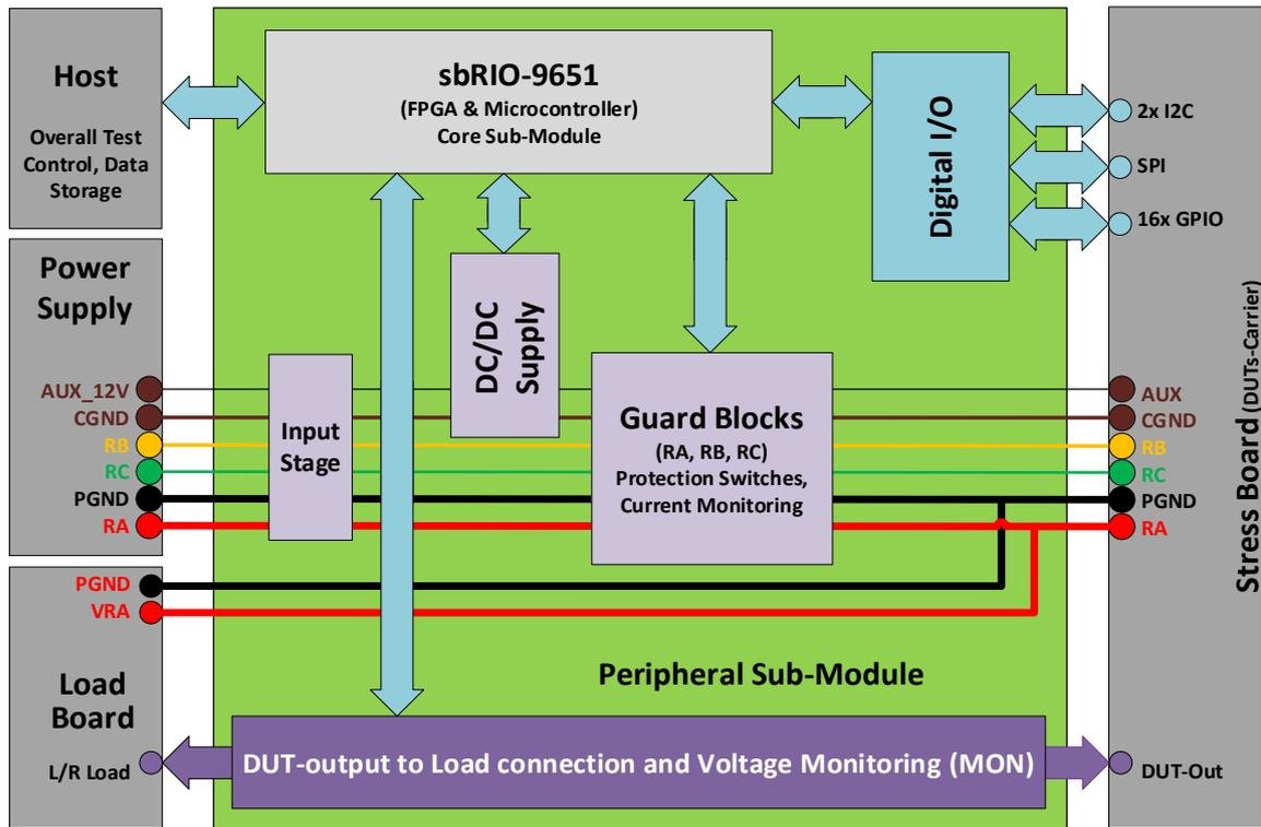
Figure 5.1: Block diagram of the [FPGA](#)-based control module. In the top left area, the core sub-module, the sbRIO-9651 from [NI](#), is shown which is plugged onto the *peripheral sub-module*. The latter is depicted as the green rectangle on which all implemented circuit blocks and their connections are shown. In the gray rectangles left and right of the figure, additionally necessary test system components are depicted [19].
