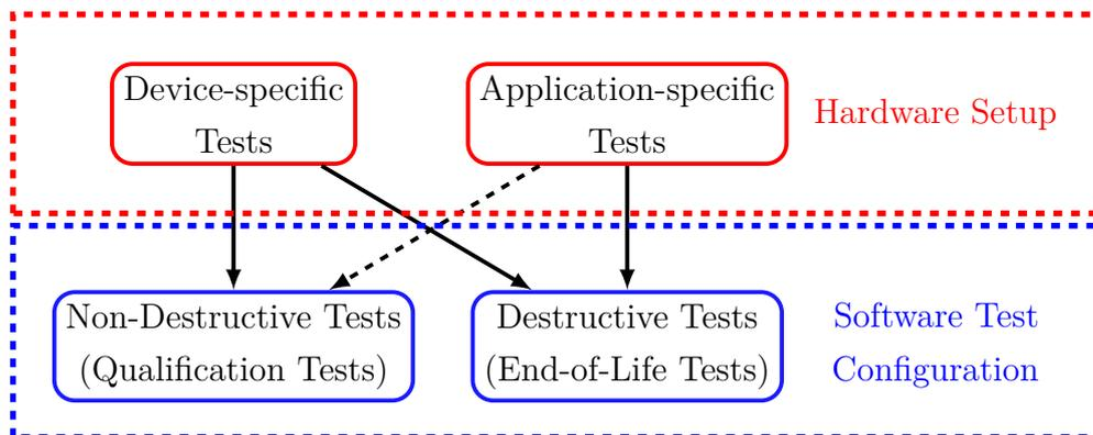
Figure 2.2: Various types of life tests which are all executable by the MTS. Which of their properties are set by hardware or software, is depicted.
