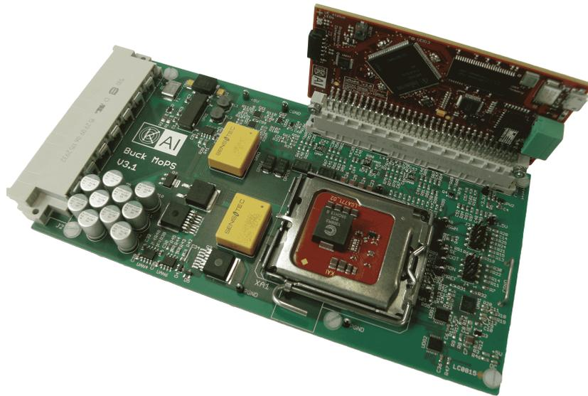
Figure A.1: One test unit of the [LV MTS](#) is depicted. In the center, the red [DUT](#) board is shown which is a separate [PCB](#) holding the [DUT](#). In the top right area, the control module [PCB](#) is connected which is equipped with an Infineon XMC4500 microcontroller. Several monitoring functions are provided on the base board. E.g., the yellow components are the current sensors and the black large [ICs](#) to the left are the guard transistors.
