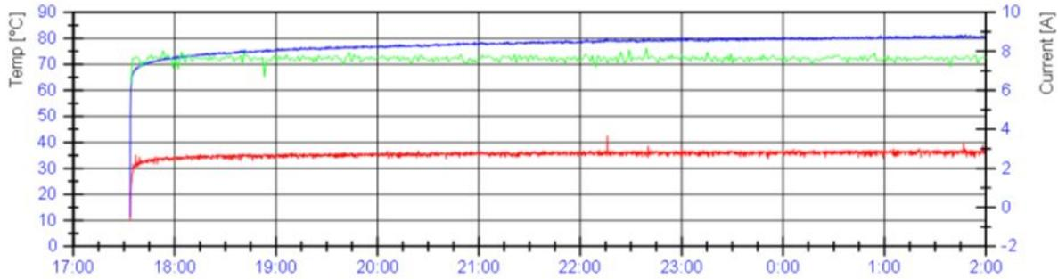
Figure 4.14: In this figure, the case temperatures of the high-side ( $T_{c,hs}$ =red) and low-side ( $T_{c,ls}$ =blue) GaN-transistor which are comprising the half-bridge circuit, are depicted. Furthermore, the input current ( $I_{in}$ =green) to the power converter is monitored during life testing [23].
