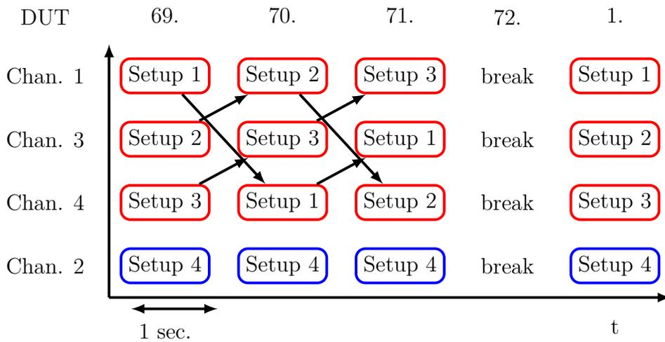
Figure 5.4: HTOL test setup timing: The setup patterns 1 to 3 are impressed onto channels 1, 3, and 4 and each pattern is rotated after one second. Channel 2 is always stimulated by the same setup 4 as it has a differently configured output load.
