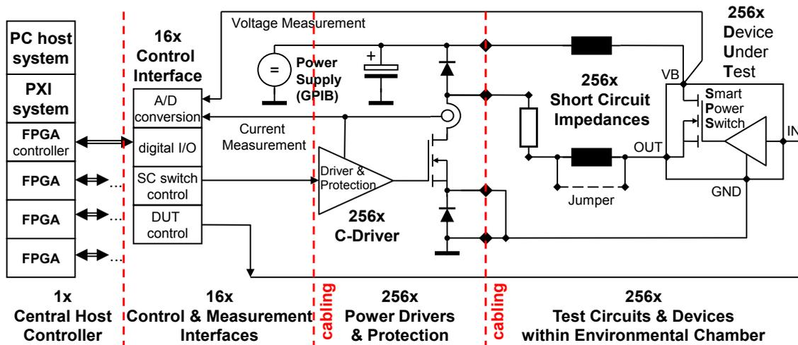
Figure 3.1: Block diagram of the centralized architecture used for the test system presented in [36]. One central host must control and measure all 256 connected DUTs within the test setup.
