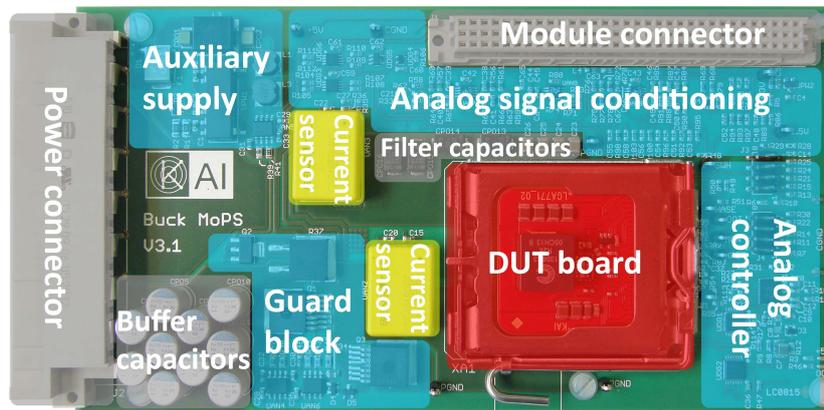
Figure 4.1: The finally manufactured PCB of the LV application module. The different circuit blocks are highlighted and described. The separate DUT board (red) is plugged onto the LV application board approximately in the center. On the top right, the module connector is shown onto which the control module needs to be plugged. The main power connector to the supplies and the electronic load is situated to the left. (In this picture, the DUT was removed from the DUT board for failure analysis.)
