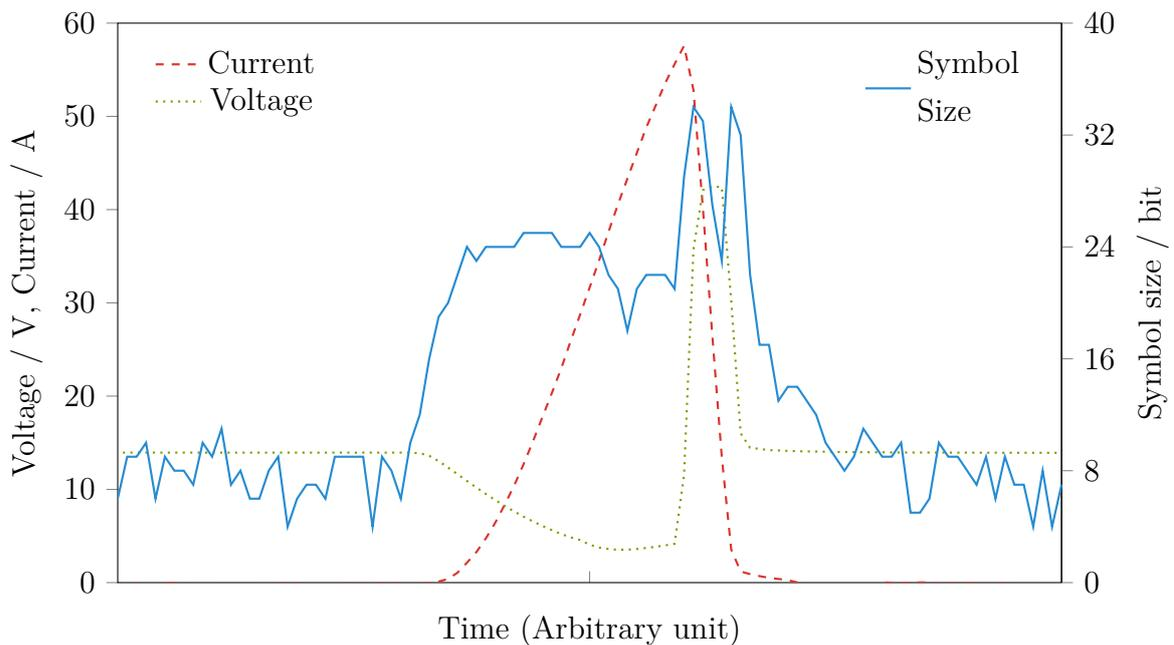
Figure 6.1: Typical symbol size for the samples within a waveform record.<sup>1</sup>
