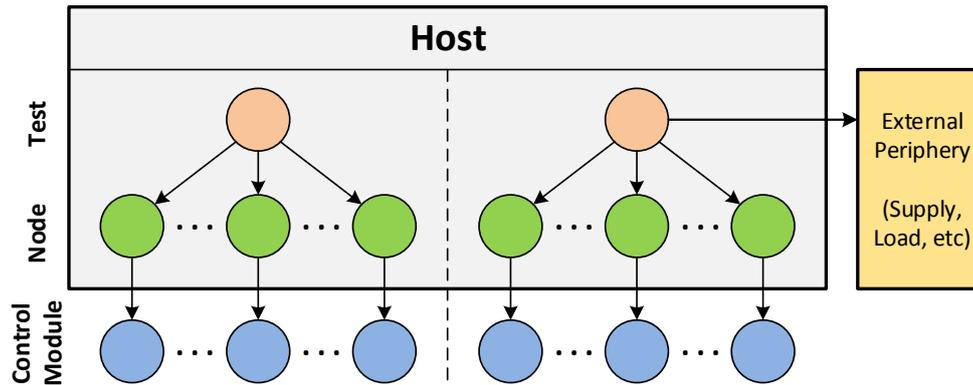
Figure 3.5: Block diagram of the software architecture: Each depicted circle represents a single FSM which holds a block of the high level script language Lua.
