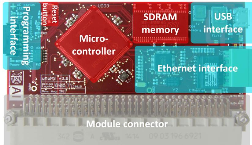
Figure 3.3: The finally manufactured [PCB](#) of the control module. The different circuit blocks are highlighted and described. The Infineon XMC4500 [73] micro-controller is located in the center left area. On the bottom, the module connector is depicted which is the interface to an application module.
