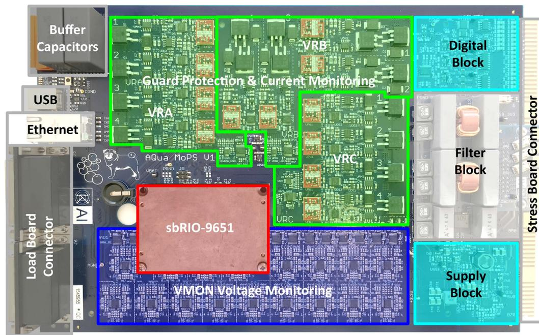
Figure 5.3: The finally manufactured PCB of the FPGA-based control module. The different circuit blocks are highlighted and described.
