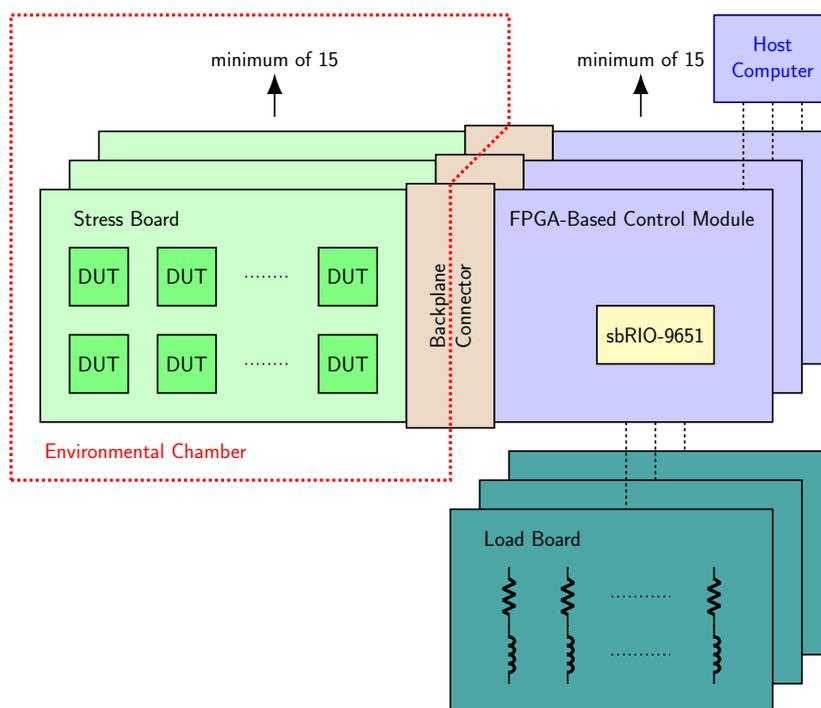
Figure 5.2: Schematic illustration of the necessary elements to establish a test system with **FPGA**-based control modules. To the left, the stress boards which hold the **DUTs** within the environmental chamber are depicted. To their right, the connection via the backplane to the **FPGA**-based control modules is shown. The optionally needed load boards which are connected via the control modules are on the bottom of the picture.
