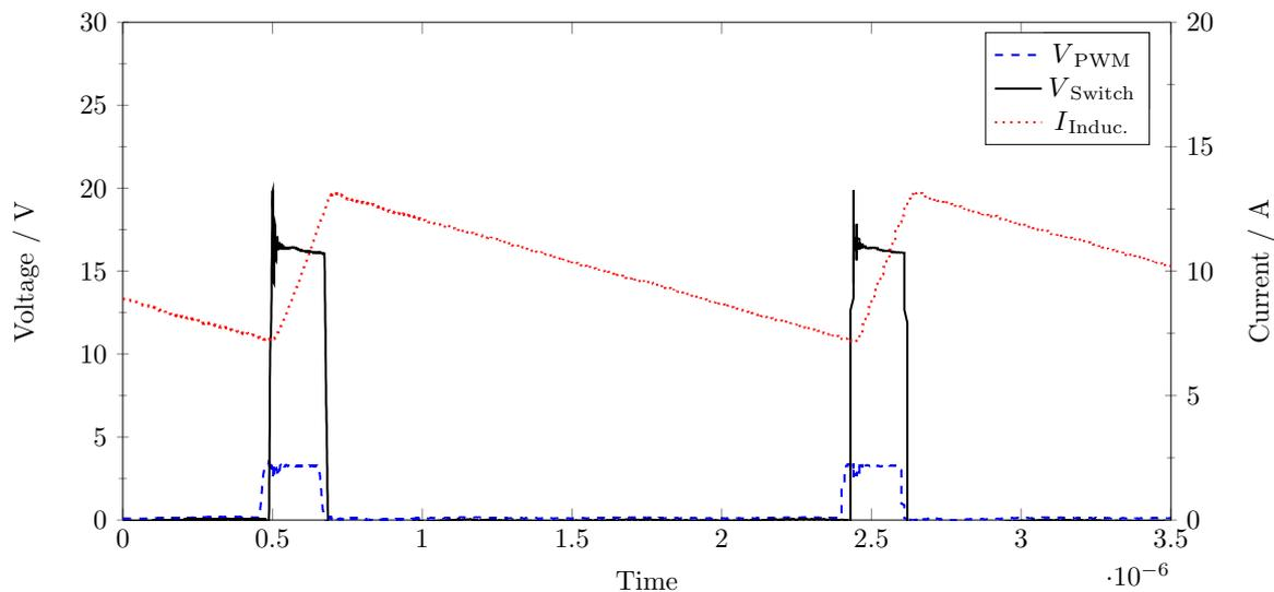
Figure 4.7: Measurement shot of important parameters of an **LV** application module while the converter is running. The blue dashed curve shows the **PWM**-signal coming from the analog controller. The red dotted and the black curve indicate the current through the inductor and the voltage at the node between the switching transistors, respectively.
