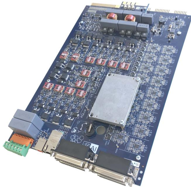
Figure A.4: Aspect view of the final manufactured PCB of the FPGA-based control module. The core sub-module sbRIO-9651 is located approximately in the center which is the solid light gray block. In the top area, the long PCB edge connector which interfaces the backplane connector in the test system can be seen. On the bottom, the black sub-D connectors are the interface to the load boards and next to them on the left, the Ethernet connector is located.
