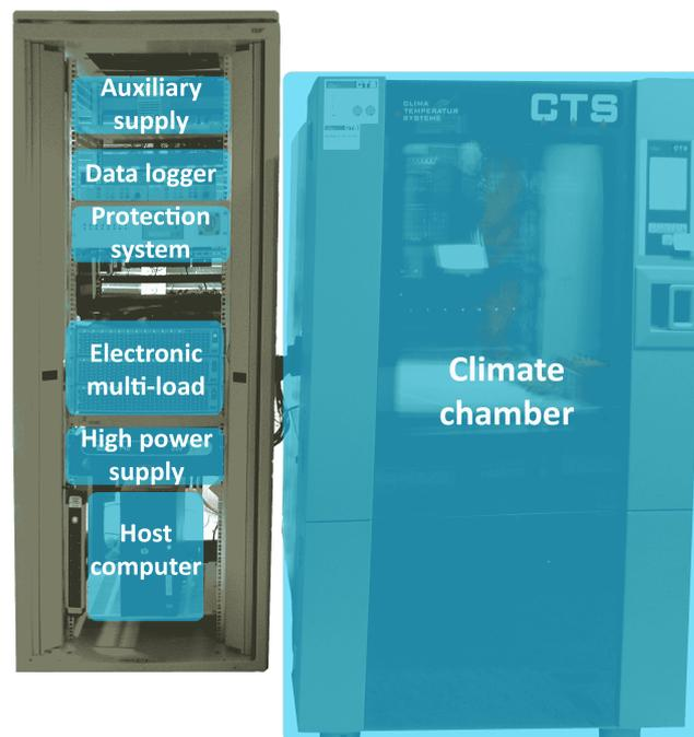
Figure A.2: In this picture, a completely established LV MTS is shown. The test units (which are shown in Figure A.1) are mounted within the climate chamber and the peripheral devices, like power supplies, electronic multi-load, host computer and an additional high voltage safety protection system are located in the 19" rack to the left.
