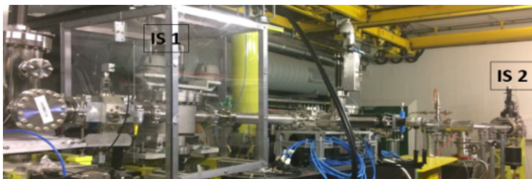
Figure 5.1: Photograph of the AWAKE diagnostics section located downstream of the vapour source (the vapour source is located out of the photo on the left hand side). The protons come from the left hand side. The two imaging stations are marked with IS 1 and 2.
