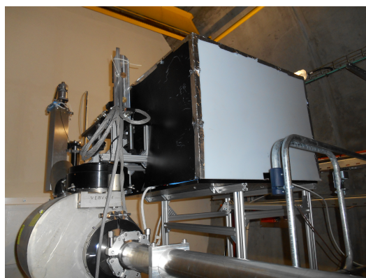
(b) Photograph of IS 2 in the tunnel. The protons come from the right hand side. The optics components are installed under the box.
